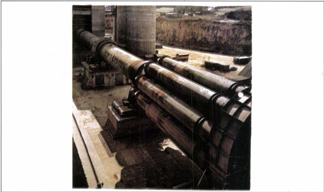
Plate 10.1 Rotary cement kiln with planetary coolers.
