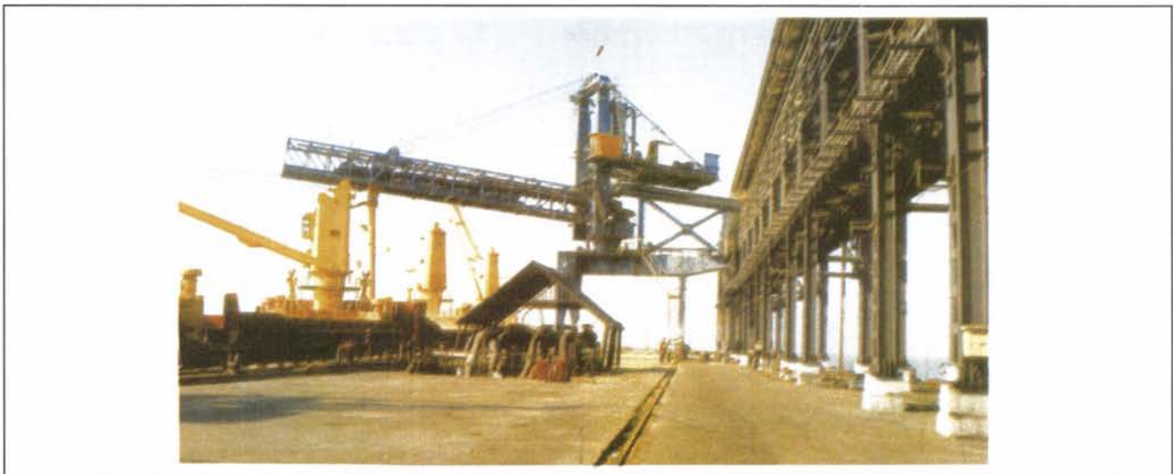
Plate 15.3 Ship loading and unloading machines for bulk cement.
