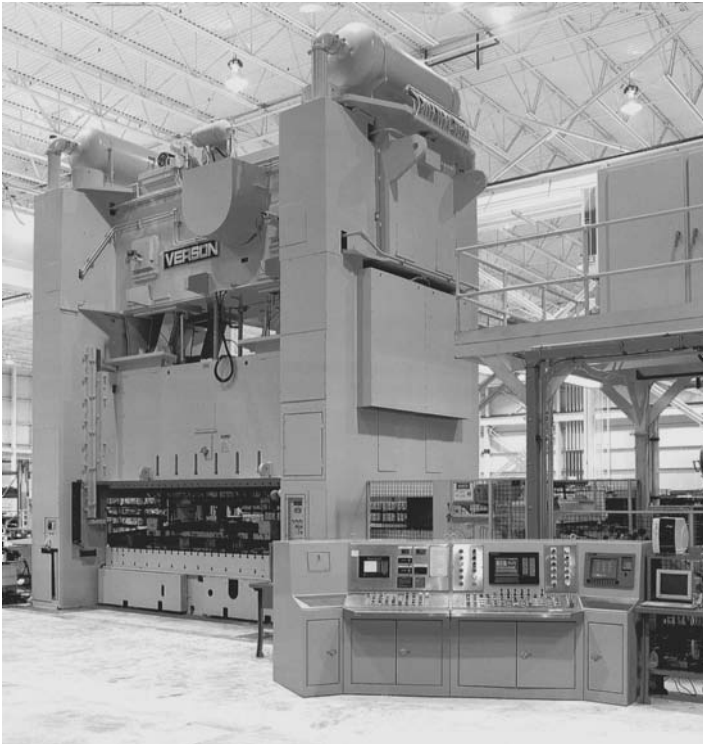
FIGURE 5-18 Verson 1000 ton Link Drive Blanking Press, model LE4-1000-180-96T and integrated blanking line control console. Link drive provides fast advance and slow down during the blanking portion of the stroke to increase production while reducing the shock associated with the blanking operation. This press is typical of automotive blanking presses with 12 in. stroke and speed ranging from 20–60 SPM. (Reprinted with permission from Verson and Danly Division of Enprotech Mechanical Services, Inc., Lansing, MI.)
