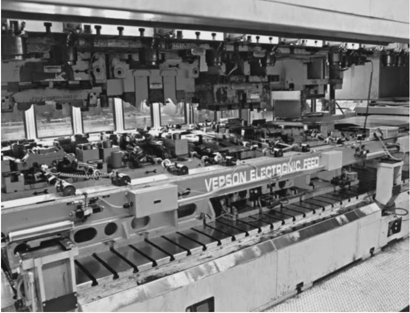
FIGURE 5-14 Danly 2500 ton Automotive Transfer Press, model S4-2500-252-108TF upgraded with a Verson Electronic tri-axis transfer system, model ETF 45-9-8TA for transferring parts up to 45 in. between stations at up to 20 strokes per minute. (Reprinted with permission from Verson and Danly Division of Enprotech Mechanical Services, Inc., Lansing, MI.)
