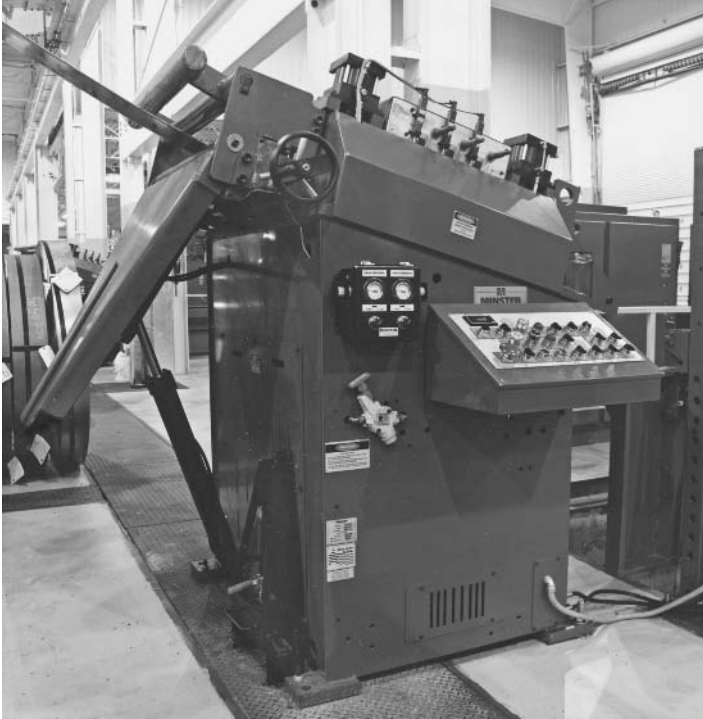
FIGURE 5-23 Straightener with eddy-current drive. (Reprinted with permission from Minster Machine Co., Ohio.)
