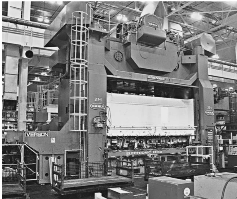
FIGURE 5-13 Verson Model ETF-48-9-10TA Electronic Tri-Axis Transfer System with full programmable servo control for up to 48 in. Transfer stroke, 9 in. Clamp stroke, and 10 in. Lift. Motion parameters and die parameters, including the number of finger sensing and die sensing stations, can be programmed in the “die library menu” and displayed on the Smart Screen operator interface. (Reprinted with permission from Verson and Danly Division of Enprotech Mechanical Services, Inc., Lansing, MI.)
