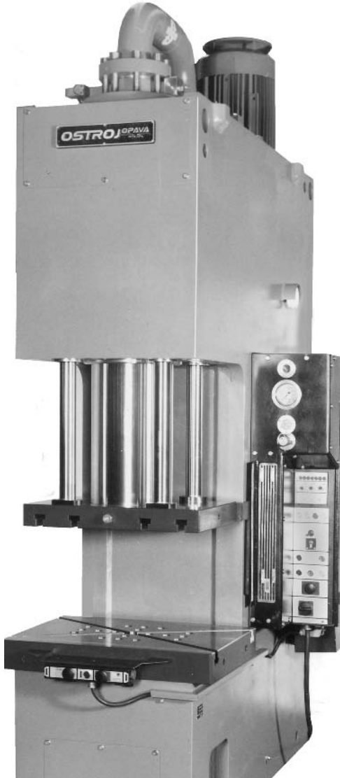
FIGURE 5-11 C-frame hydraulic press. Frame: welded. Capacity: 250 to 2500 kN. Working speed up to 8–38 mm/sec. Maximum pressure 21 to 24.5 MPa. Electrohydraulic controls by Mannesmann Rexroth. (Reprinted with permission from OSTROJ, Opava, Czech Republic.)
