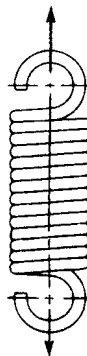
FIGURE 12-3 Helical extension spring. (From "Design Handbook," 1987. Reprinted with permission from Associated Spring, Barnes Group, Inc., Dallas, TX.)
