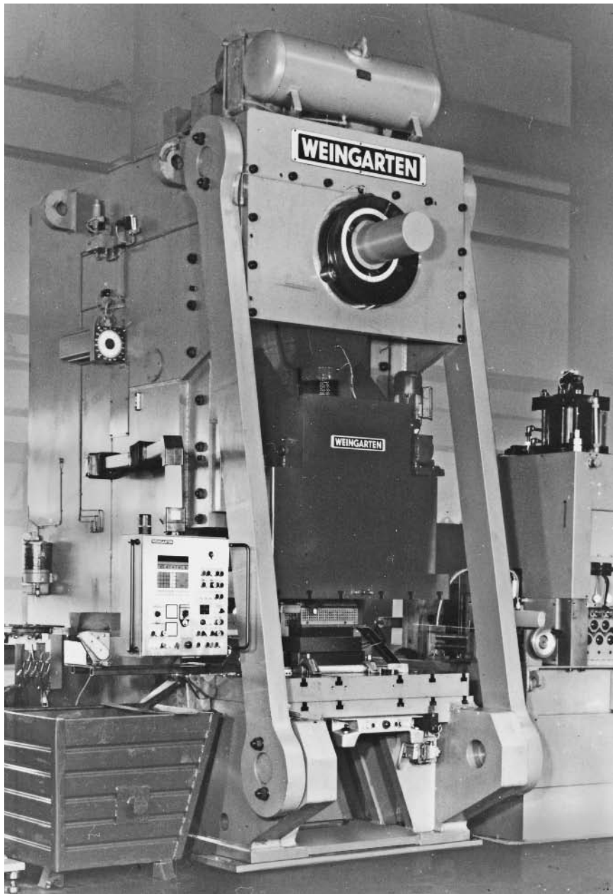
FIGURE 5-12 Open-front power press. Notice the heavy tie rods. (Reprinted with permission from Müller Weingarten AG, Germany.)
