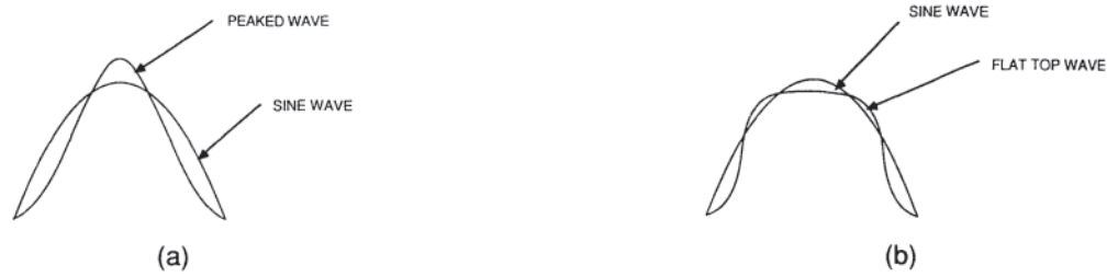
Figure 5.3 Flux density distributions, (a) Peaked wave compared to a sine wave, (b) Flat-topped wave compared to a sine wave.
