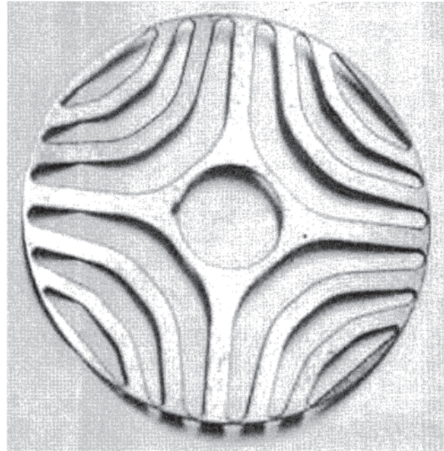
Figure 2.133 Example of optimized rotor design.
