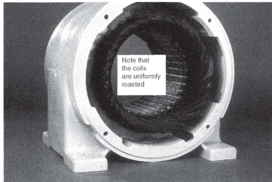
Figure 14.12 Winding damage due to overload. (Courtesy of the Electrical Apparatus Service Association, St. Louis, MO.)
