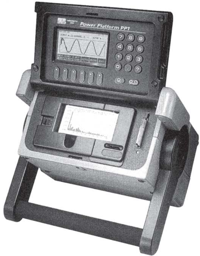
Figure 14.7 AC power monitor, Dranetz Power Platform pp1. (Courtesy of Dranetz-BMI, Edison, NJ.)
