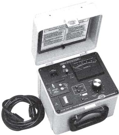
Figure 14.6 Portable dielectric strength tester, Biddle Model 230 425, 0 to 4000 V ac, 0 to 5000 V dc, 12 mA. (Courtesy of AVO International, Dallas, TX.)
