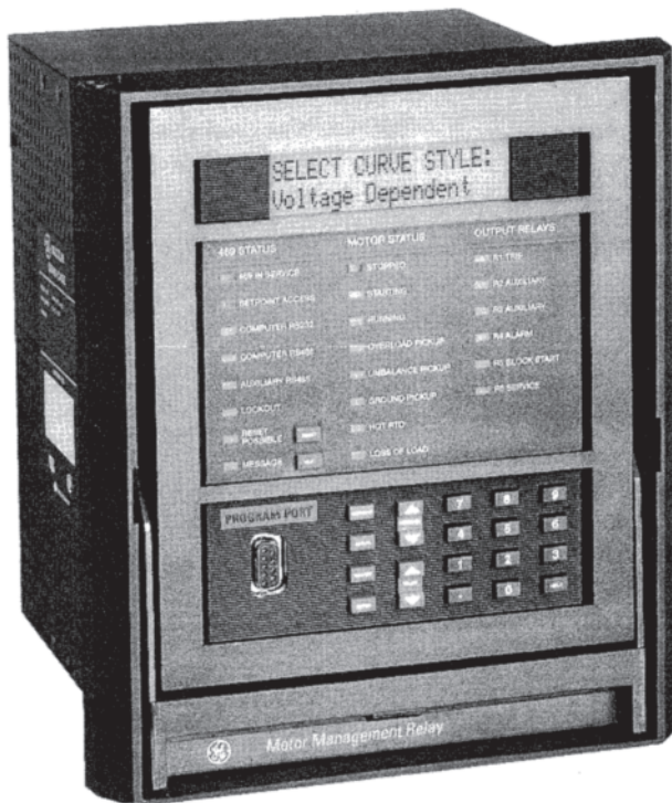
Figure 10.1 Medium-voltage motor protection relay. (Courtesy of GE/Multilin.)
