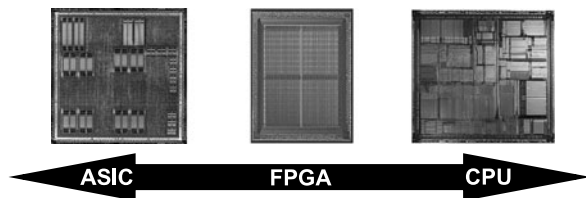
Fig. A.1 On a continuum of generality, CPUs are the most programmable, and ASICs are the least
