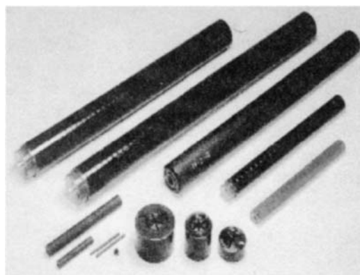
Figure 12.5 Extruded-type solid propellants [10]. (Source: http://www.nof.co.jp/E_nof/business%20activities/Explosives.htm .)
