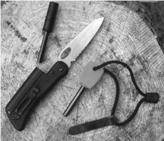
Swedish FireSteel and Tool Logic SL3 knife with FireSteel insert. Fire starters like this one are hot and work in any weather, even rain.
