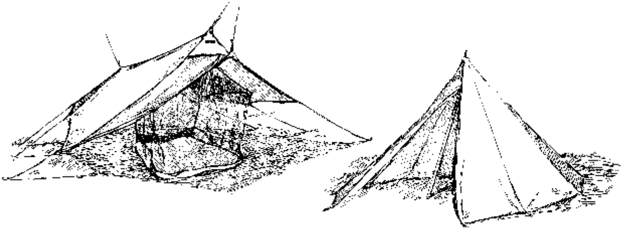
LEFT: Tarp with bug-netting inner. GoLite Cave and Nest. RIGHT: Tarp pitched as a pyramid with a single pole.
