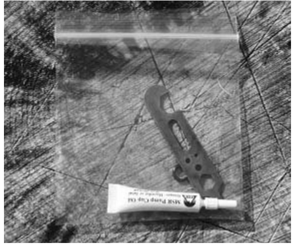
A stove maintenance kit is necessary for white-gas and multifuel stoves. The contents depend upon the model, but a kit usually contains O-rings, a tool for dismantling the stove, pump leather oil, jets, jet needles, and a leather pump cup.
