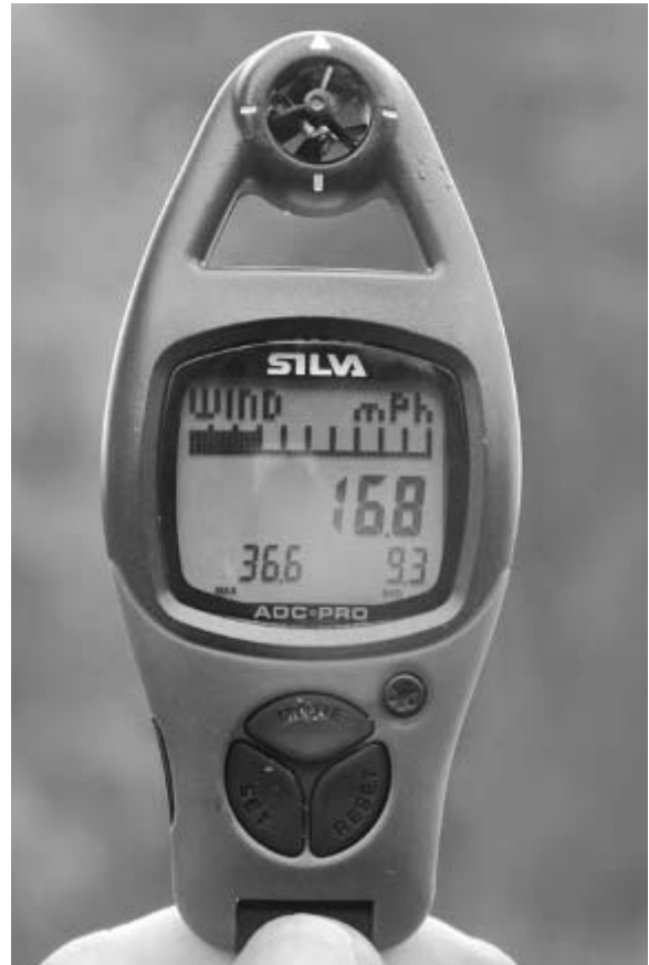
The Brunton (Silva) ADC Pro weather-recording instrument.
