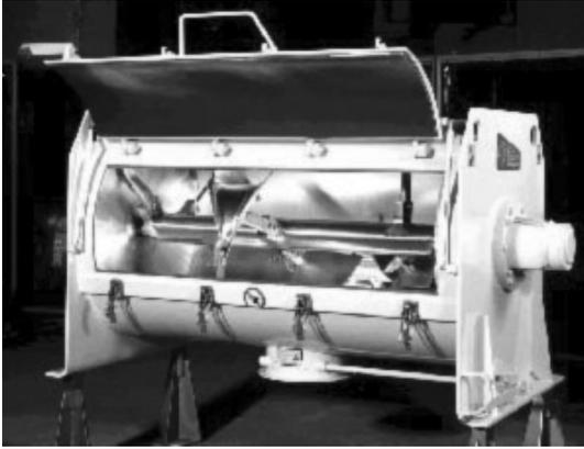
**Figure 15-34** Plow mixer (Courtesy of Scott Equipment Company.)
