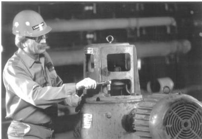
**Figure 22-21** Service engineer adjusting speed reducer.
