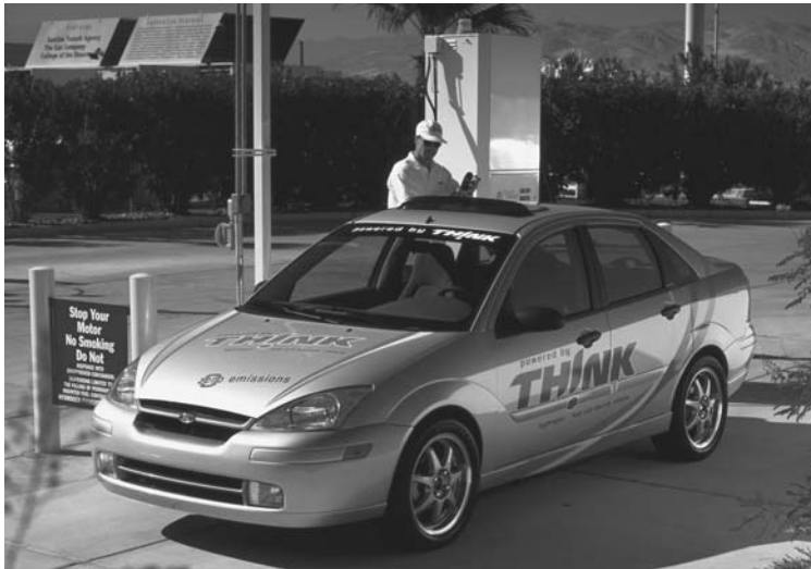
FIGURE 10.9 Ford's Focus FCV vehicle being refueled with hydrogen. (Photograph courtesy of Ford.) (Please check Color Figure 10.9 following page 9-10.)
