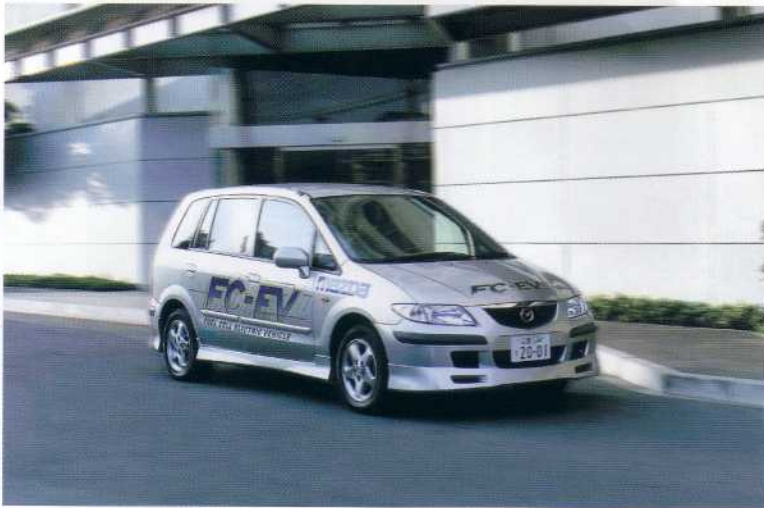
CHAPTER 10, COLOR FIGURE 10.11 Mazda's methanol-powered Premacy FC-EV (2001) powered by a Ballard Mark 900 series stack. (Photograph courtesy of Mazda.)
