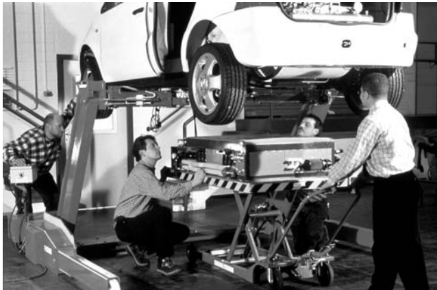
FIGURE 10.6 Simple handling: The compact fuel cells are installed in the NeCar concept vehicle. The sandwich floor of the A-class provides an ideal platform for alternative propulsion systems. (Photograph courtesy of Daimler-Chrysler.) (Please check Color Figure 10.6 following page 9-10.)
