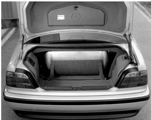
FIGURE 5.2 Liquid hydrogen tank inside a BMW 7 series family sedan powered by hydrogen internal combustion. (Source: BMW.)
