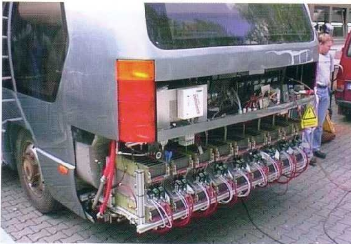
CHAPTER 10, COLOR FIGURE 10.19 Bus developed by Proton Motor (with Neoplan). The bus features a special flywheel energy storage device. (Photograph courtesy of Proton Motor.)
