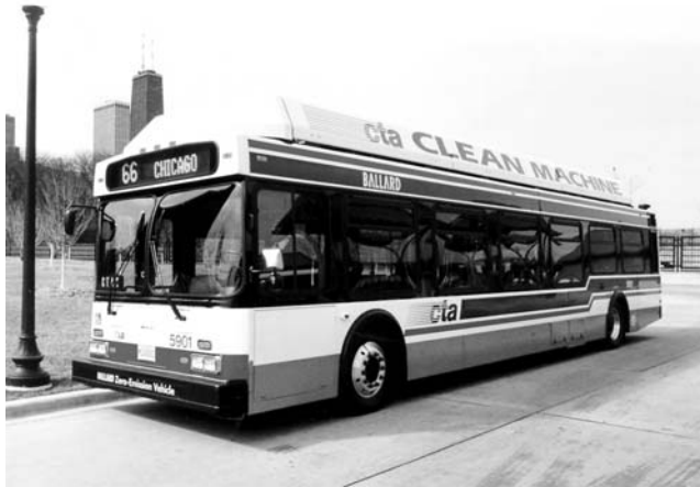
FIGURE 10.13 Xcellsis P3 bus operating during extensive field tests in Chicago. (Photograph courtesy of Ballard Power Systems.) (Please check Color Figure 10.13 following page 9-10.)
