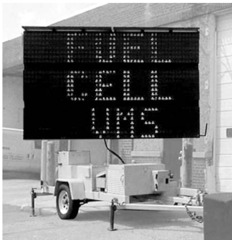
FIGURE 9.9 H-Power variable road message sign with fuel cell backup power. (Photograph courtesy of H-Power.)
