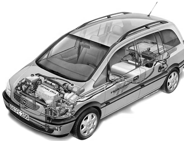
FIGURE 10.2 HydroGen 1 fuel cell prototype produced by General Motors/Opel in 2000. HydroGen 1 runs 400 km on a 75-liter tank of liquid hydrogen. (Photograph courtesy of Adam Opel AG.) (Please check Color Figure 10.2 following page 9-10.)
