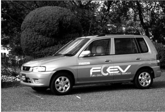
FIGURE 10.10 Mazda’s Demio FCEV presented in 1997. The vehicle was powered by four stacks (20 kW total power) developed by Mazda and assisted by ultra-capacitors. Hydrogen fuel was stored in a metal hydride tank. (Photograph courtesy of Mazda.) (Please check Color Figure 10.10 following page 9-10.)
