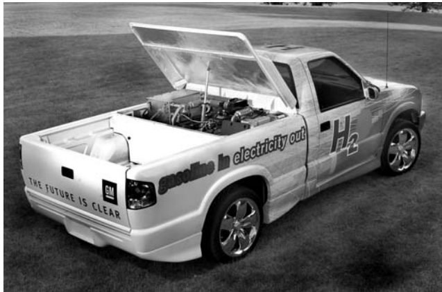
FIGURE 10.3 General Motors has unveiled the world's first on-board gasoline fuel processor for fuel cell propulsion. The Gen III processor, packaged in a Chevrolet S-10 pickup, reforms "clean" gasoline on board, extracting a stream of hydrogen to send to the fuel cell stack. The vehicle was introduced to an automotive management conference on August 7, 2001, in Traverse City, MI, by Larry Burns, GM's vice president of research and development and planning. (Photographer: Joe Polimeni; courtesy of General Motors.) (Please check Color Figure 10.3 following page 9-10.)
