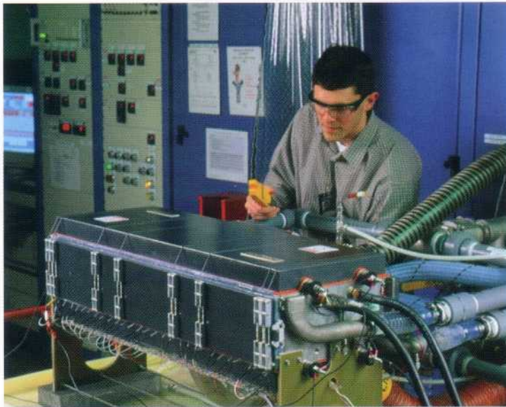
CHAPTER 10, COLOR FIGURE 10.17 A Series 300 transportation fuel cell stack is put through testing at UTC Fuel Cells' research and development test labs. (Photograph courtesy of UTC Fuel Cells.)
