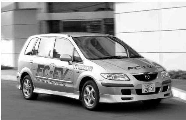
FIGURE 10.11 Mazda’s methanol-powered Premacy FC-EV (2001) powered by a Ballard Mark 900 series stack. (Photograph courtesy of Mazda.) (Please check Color Figure 10.11 following page 9-10.)
