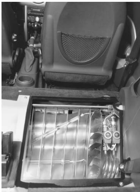
FIGURE 5.3 The package study for MINI Cooper Hydrogen has a hydrogen tank that fits into the body of the MINI. (Photograph courtesy of BMW.)
