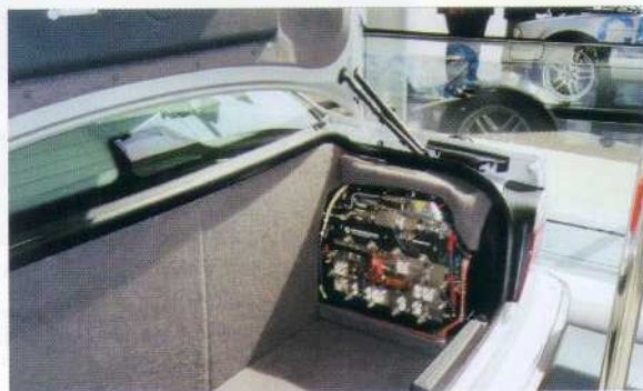
CHAPTER 9, COLOR FIGURE 9.10 (a) Hydrogen-powered APU system developed by UTC Fuel Cells (formerly IFC). (Photograph courtesy of BMW.) (b) APU installed in BMW's hydrogen internal combustion engine car. (Photograph courtesy of UTC Fuel Cells.)
