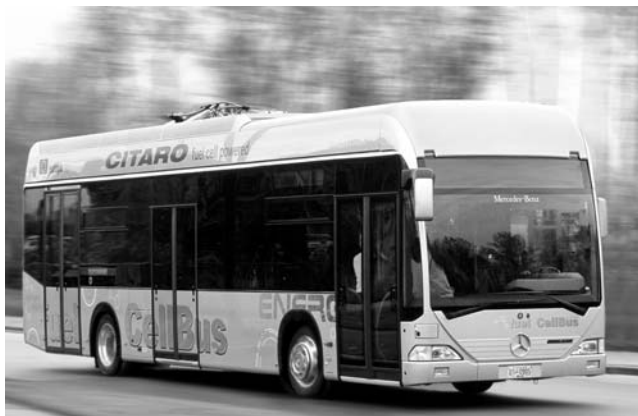
FIGURE 10.14 The first Citaro bus with a fuel cell power system enters driving tests. (Photograph courtesy of DaimlerChrysler.) (Please check Color Figure 10.14 following page 9-10.)
