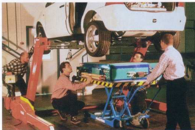
CHAPTER 10, COLOR FIGURE 10.6 Simple handling: The compact fuel cells are installed in the NeCar concept vehicle. The sandwich floor of the A-class provides an ideal platform for alternative propulsion systems. (Photograph courtesy of DaimlerChrysler.)
