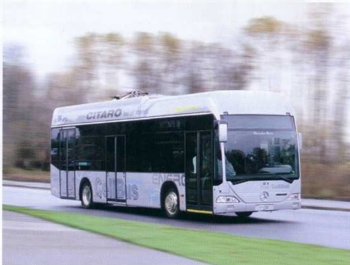
CHAPTER 10, COLOR FIGURE 10.14 The first Citaro bus with a fuel cell power system enters driving tests. (Photograph courtesy of DaimlerChrysler.)
