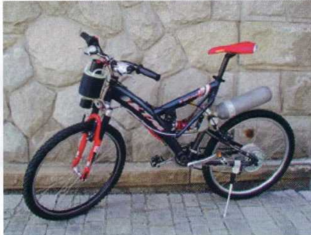
CHAPTER 9, COLOR FIGURE 9.5 (a) This 600-W power supply unit developed by NovArs/Manhattan Scientific is based on a polymer electrolyte fuel cell that uses compressed hydrogen and air to produce electric power. (b) Manhattan Scientifics' Hydrocycle presented in June 2000. On the fuel cell bicycle, compressed hydrogen flows from a 2-liter cylindrical tank to the fuel cell. (Photographs courtesy of Manhattan Scientifics).
