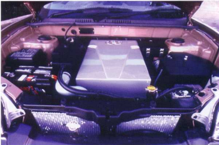
CHAPTER 10, COLOR FIGURE 10.18 (a) Hyundai Santa Fe fuel cell vehicle powered by a UTC ambient-pressure 75-kW fuel cell running on hydrogen. (b) The view under the hood shows system integration. Note that the fuel cell is not under the hood in this application but under the rear seats. (Photographs courtesy of UTC Fuel Cells.)
