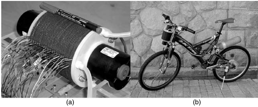
FIGURE 9.5 (a) This 600-W power supply unit developed by NovArs/Manhattan Scientific is based on a polymer electrolyte fuel cell that uses compressed hydrogen and air to produce electric power. (b) Manhattan Scientifics' Hydrocycle presented in June 2000. On the fuel cell bicycle, compressed hydrogen flows from a 2-liter cylindrical tank to the fuel cell. (Photographs courtesy of Manhattan Scientifics). (Please check Color Figure 9.5 following page 9-10.)
