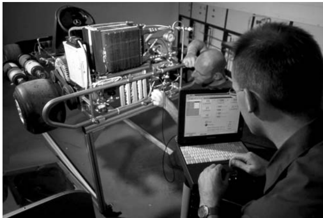
FIGURE 10.8 In 2000, DaimlerChrysler showed a go-cart powered by a direct methanol fuel cell (DMFC). The 3 kW system is the result of an ongoing collaboration between the research groups of DaimlerChrysler and Ballard. (Photograph courtesy of DaimlerChrysler.)
