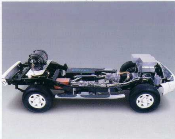
CHAPTER 10, COLOR FIGURE 10.15 (a) Nissan's Xterra FCV. (b) The vehicle is powered by a Ballard Mark 900 fuel cell module. (Photographs courtesy of Nissan.)
