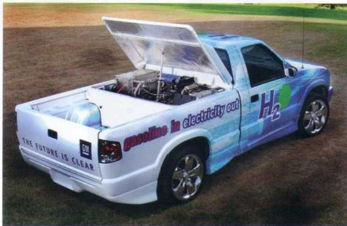
CHAPTER 10, COLOR FIGURE 10.3 General Motors has unveiled the world's first on-board gasoline fuel processor for fuel cell propulsion. The Gen III processor, packaged in a Chevrolet S-10 pickup, reforms "clean" gasoline on board, extracting a stream of hydrogen to send to the fuel cell stack. The vehicle was introduced to an automotive management conference on August 7, 2001 in Traverse City, MI, by Larry Burns, GM's vice president of research and development and planning. (Photographer: Joe Polimeni; courtesy of General Motors.)
