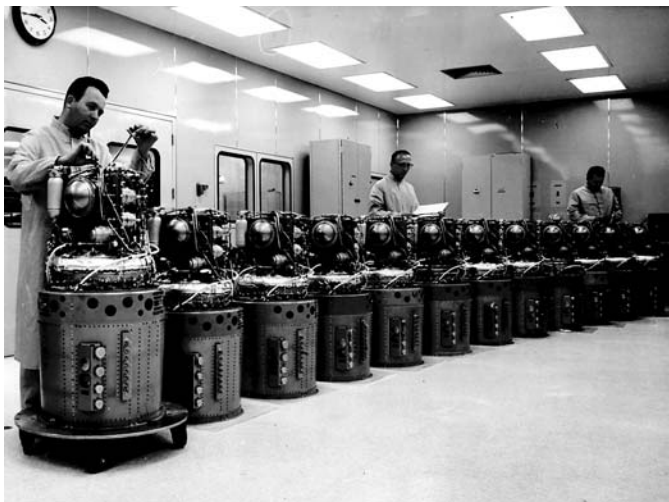
FIGURE 2.11 Apollo fuel cell systems being assembled by Pratt & Whitney Aircraft engineers. The lower half is the stack. (Courtesy of UTC Fuel Cells.)
