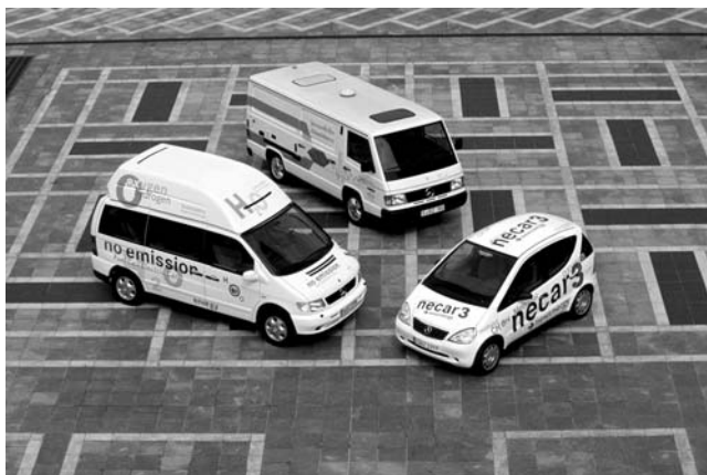
FIGURE 10.5 DaimlerChrysler's first three fuel cell demonstration vehicles, the hydrogen-powered NeCar 1 and 2, and NeCar 3 with on-board methanol reformer. (Photograph courtesy of DaimlerChrysler.) (Please check Color Figure 10.5 following page 9-10.)
