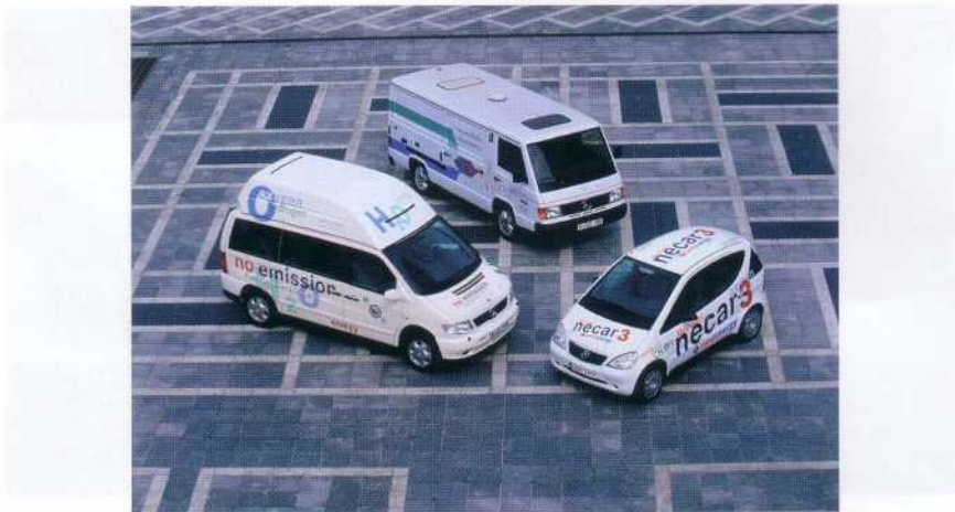
CHAPTER 10, COLOR FIGURE 10.5 DaimlerChrysler's first three fuel cell demonstration vehicles, the hydrogen-powered NeCar 1 and 2, and NeCar 3 with on-board methanol reformer. (Photograph courtesy of DaimlerChrysler.)
