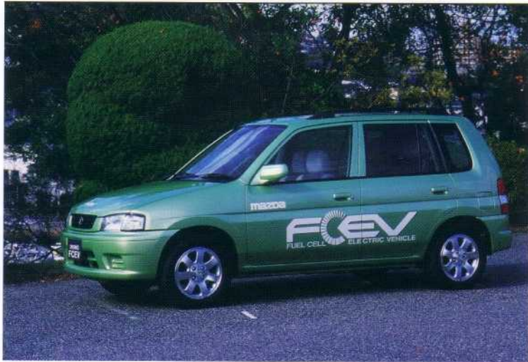
CHAPTER 10, COLOR FIGURE 10.10 Mazda's Demio FCEV presented in 1997. The vehicle was powered by four stacks (20 kW total power) developed by Mazda and assisted by ultra-capacitors. Hydrogen fuel was stored in a metal hydride tank. (Photograph courtesy of Mazda.)
