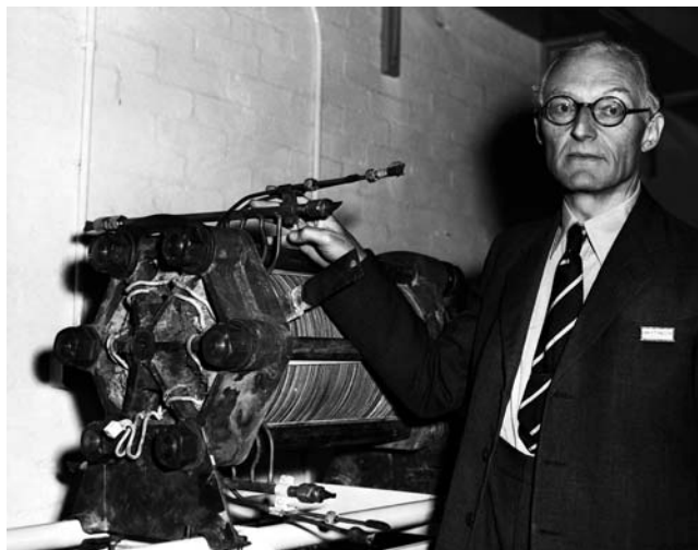
FIGURE 2.10 Bacon with the 6-kW fuel cell stack, presented in 1959. (Copyright Hulton-Deutsch Collection/Corbis.)
