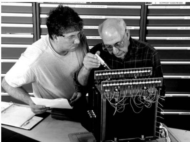
FIGURE 8.16 The fuel cell stack in the picture is at the heart of the residential fuel cell being developed by UTC. (Photograph courtesy of UTC Fuel Cells.)
