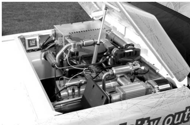
FIGURE 5.6 General Motors has unveiled the world's first on-board gasoline fuel processor for fuel cell propulsion. The Gen III processor, packaged in a Chevrolet S-10 pickup, reforms "clean" gasoline on board, extracting a stream of hydrogen to send to the fuel cell stack. The vehicle was introduced to an automotive management conference on August 7, 2001, in Traverse City, MI, by Larry Burns, GM's vice president of research and development and planning. (Photographer: Joe Polimeni.) For a photograph of the entire car see Fig. 10.3 .
