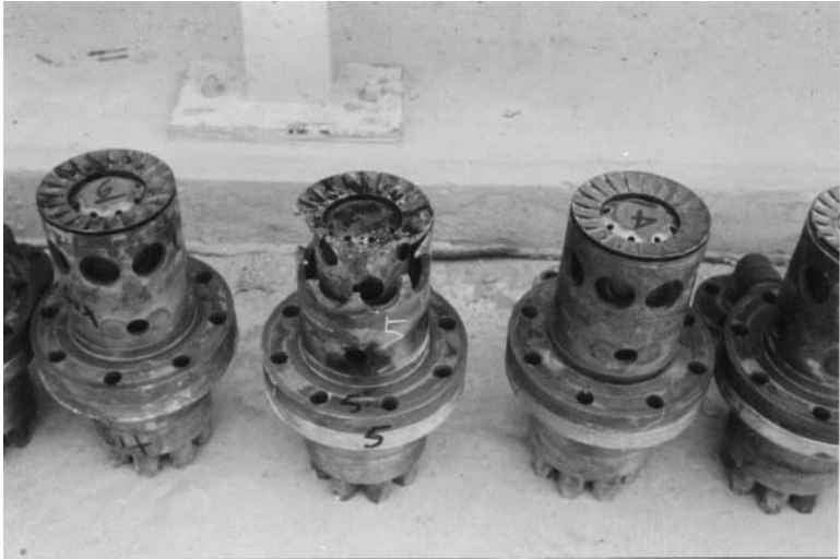
Figure 13-13. Burnt fuel nozzles from can-annular combustor. 55,000 horsepower gas turbine-generator with less than 10,000 operating hours.
