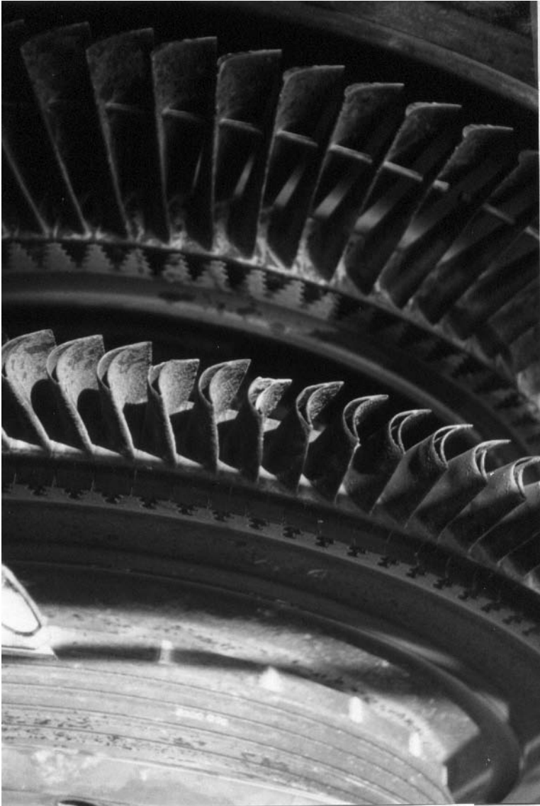
Figure 3-7. Courtesy of Power & Compression Systems. This is a 1970 vintage gas turbine designed with lacing wire to dampen the second stage turbine blades. Note the hollow 1st stage turbine blade indicating blade cooling and the corrosion on both the 1st and the 2nd-stage blades.
