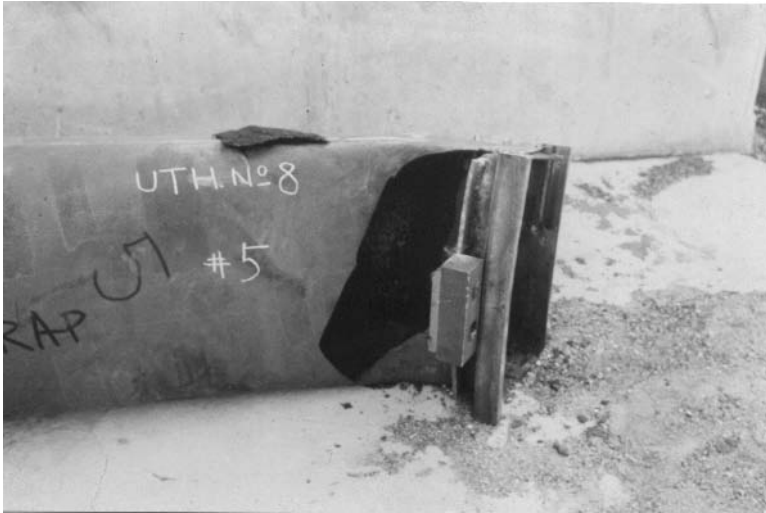
Figure 13-11. Can-annular combustor transition piece failure due to brittle fatigue due to fretting. 55,000 horsepower gas turbine-generator with less than 10,000 hours operation.
