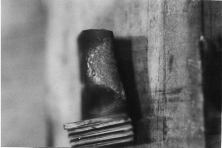
Figure 13-26. Sulfidation corrosion attack on first stage turbine blade. 4,500 horsepower gas turbine-generator drive unit with under 45,000 hours operation.
