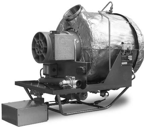
Figure 11-1. Courtesy of Capstone Turbine Corporation. The C30 & C60 microturbine systems are ultra-low-emission combined heat and power generator sets providing up to 30 kW and 60 kW of power, 85 kW and 150 kW of heat, at heat rates of 13,100 Btu/kW-Hr and 12,200 Btu/kW-Hr, respectively.
