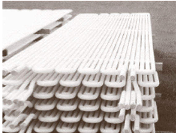
Fig. 16.41 Arrangement of a platen superheater
