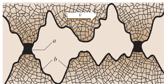
Fig. 5.15 Formation of a protective layer by EP active ingredients of sulfur compounds. a: metal-sulfide compound; b: metal surface (after [5.16])
