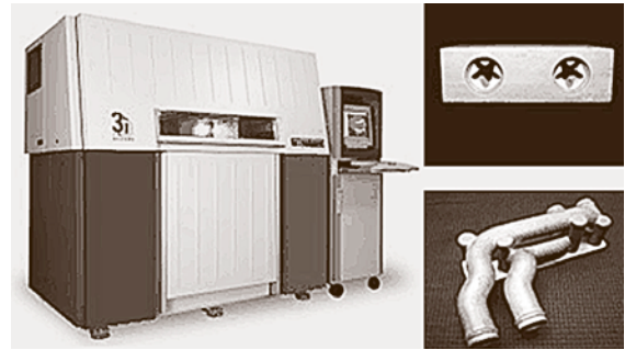
Fig. 7.327 Sinterstation HiQ System of 3-D Systems. Technical characteristics: materials: steels ST100, ST200 and A6; no full melting, infiltration required; layer thickness 70 \mu\text{m} ; accuracy 0.05–0.1 mm; build volume 330 \times 380 \times 457 mm; speed 50–80 \text{cm}^3/\text{h}
