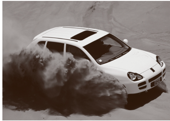
Fig. 13.81 Test with sports utility vehicle to verify performance in dry and dusty environment (courtesy of Dr. Ing. h.c. F. Porsche AG)
