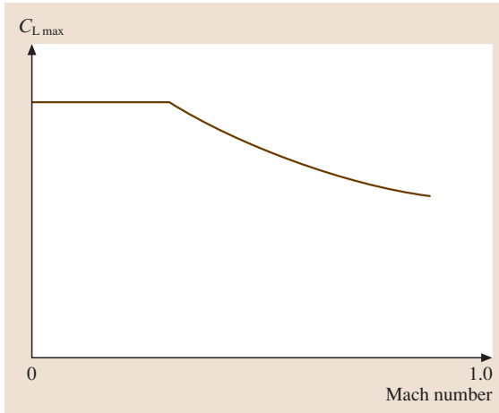
Fig. 13.169 Mach number effect on maximum lift coefficient at high subsonic speeds
