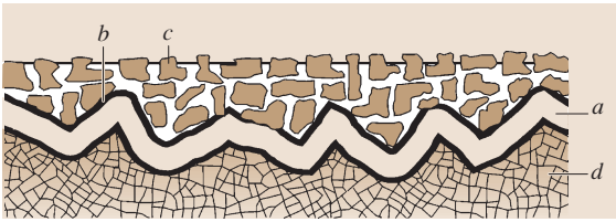
Fig. 5.16 Solid lubrication made of lubricating varnish: a: phosphate layer (3 \mu\text{m} ); b: binder; c: solid lubricant; d: base metal (after [5.16])
