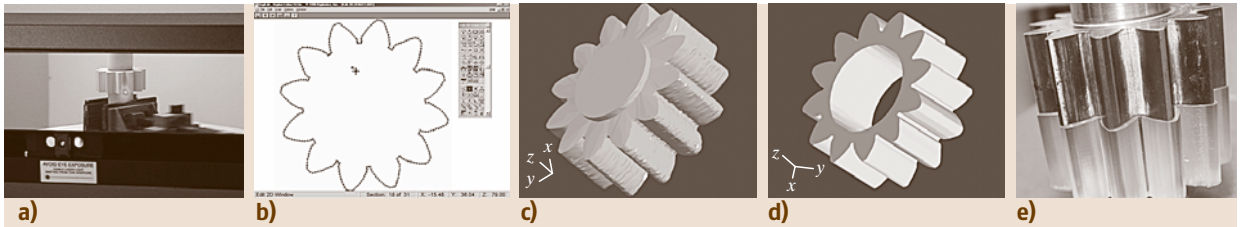
Fig. 7.345a–e Digitizing phases of a gear wheel: (a) placing on the scanner table and starting the digitizing process, (b) single contour obtained from the measurement, (c) geometrical STL model, (d) 3-D CAD model, (e) digitized gear and the gear made by SLA method after digitizing
