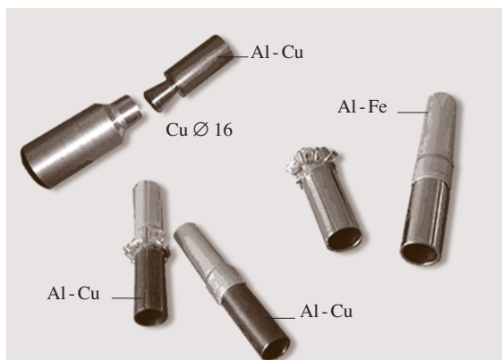
Fig. 7.302 Examples of hybrid structures of aluminum fabricated by magnetic pulse welding
