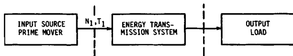
FIGURE 42.1 The energy transmission system is an interface between an input element such as a prime mover and an output element such as a load. The dashed lines indicate interfaces. (From Ref. [42.1].)
