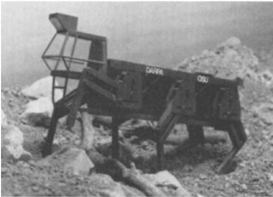
FIGURE 47.4 The adaptive suspension vehicle ( \frac{1}{10} -scale model). This is a vehicle for transportation in very rough terrain conditions which uses legged locomotion. ( The Ohio State University. )
