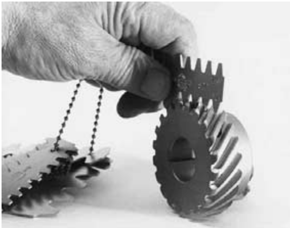
FIGURE 7.14 Measuring helical gears.
