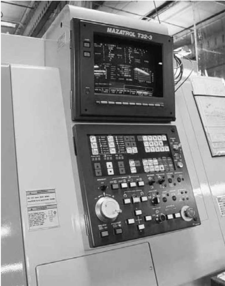
FIGURE 5.2b Turning center control panel.
