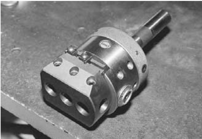
FIGURE 5.40 A modern removable insert boring head.
