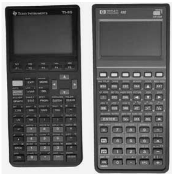
FIGURE 1.32 Programmable calculators with complex equation-solving ability and other advanced features. HP-48G on the right and the TI-85 on the left.
