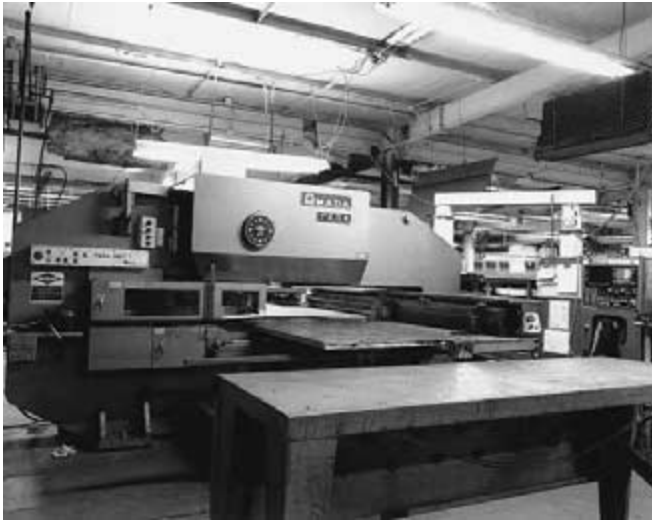
FIGURE 6.2 CNC multistation turret punch press.
