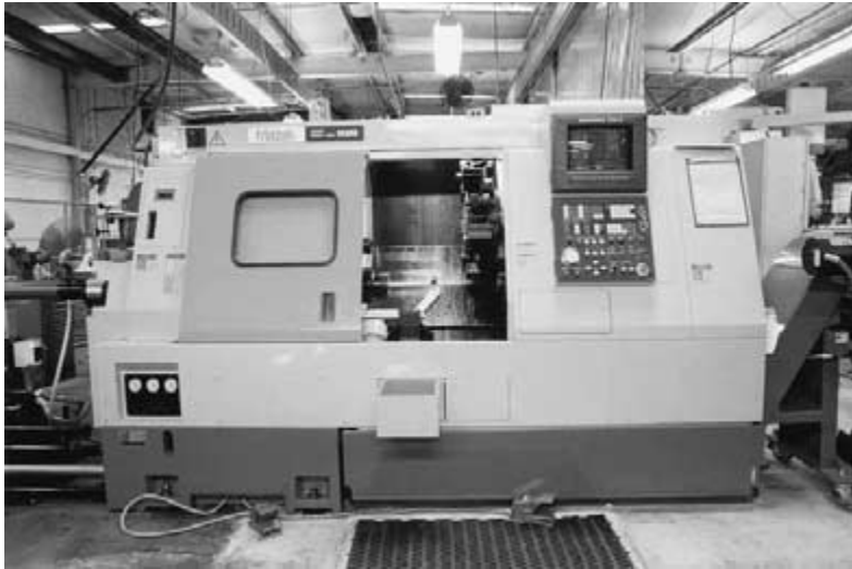
FIGURE 5.2a A modern CNC turning center.
