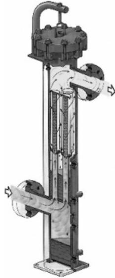
Figure 5-8. High-efficiency vertical liquid-gas coalescer system (Schlotthauer and Hashemi, 1991; Wines, 2004).
