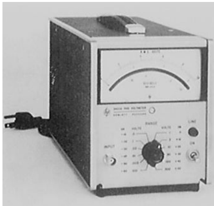
FIGURE 2.18 Electronic-type true rms meter. (Hewlett-Packard.)
