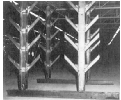
FIGURE 1.3 Plant-made racks for holding steel.
