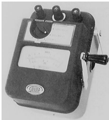
FIGURE 2.26 Portable megger. (James G. Biddle Company.)
