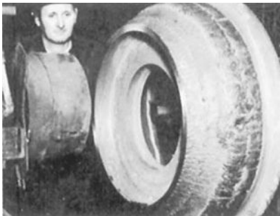
FIGURE 1.39 Cone used for uncoiling steel. Hardfacing material has been deposited on mild-steel base. Surface is ready for grinding.
