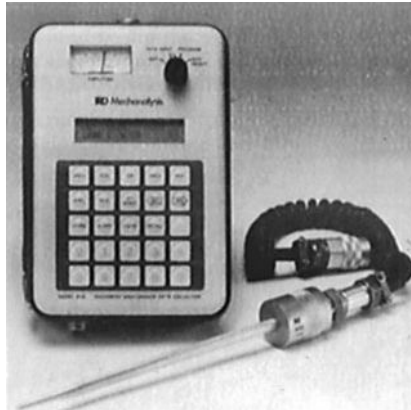
FIGURE 3.19 Hand-held vibration meter used for periodic vibration checks.
