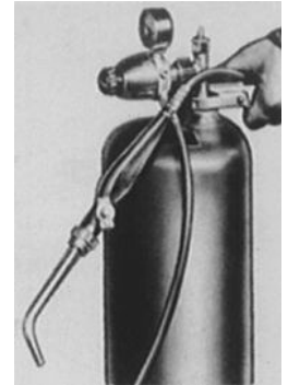
FIGURE 2.2 Connecting a typical air-acetylene outfit. The standard type of portable outfit is shown. Smaller tanks also are available.
