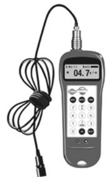
FIGURE 7.15 Sonic tension meter tensioning.
