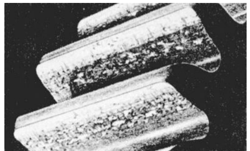
FIGURE 8.5 Severe pitting caused by overloading gear.
