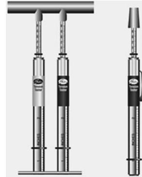
FIGURE 7.14 Pencil-type tension tester and pen method of tensioning.
