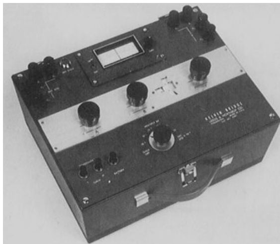
FIGURE 2.29 Portable Kelvin bridge. (Leads and Northrup.)
