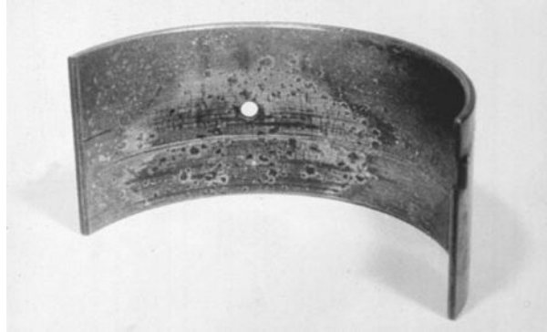
FIGURE 1.8 Bearing with severe dirt embedment.
