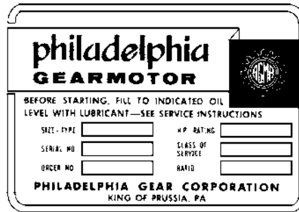
FIGURE 9.12 AGMA identification plate.
