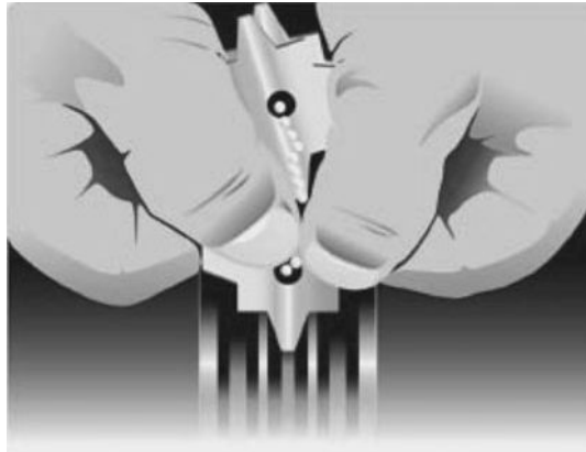
FIGURE 7.10 Sheave groove inspection.
