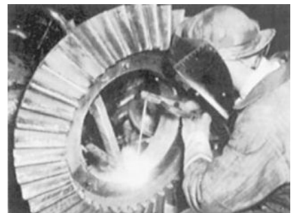
FIGURE 1.40 Using a mild-steel electrode to build up the inside diameter and all the teeth of a 25-year-old cast-steel gear that could not be replaced.
