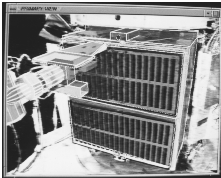
FIGURE 25.9B Status of predicted end point after motion execution from a tv camera view different from the view shown in Figure 25.9a .
