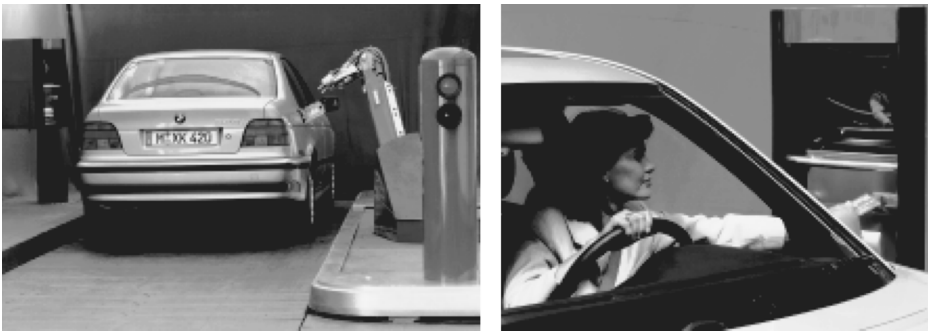
FIGURE 28.33 View of a prototype installation at Fraunhofer IPA. A car being refueled by a robot (left) and a touch-screen terminal for inserting credit card, entering refilling order and printing (right). (From Leondes, C.T., Mechatronic Systems Techniques and Applications , Vol. 2, Gordon & Breach, Amsterdam, 2000. With permission.)
