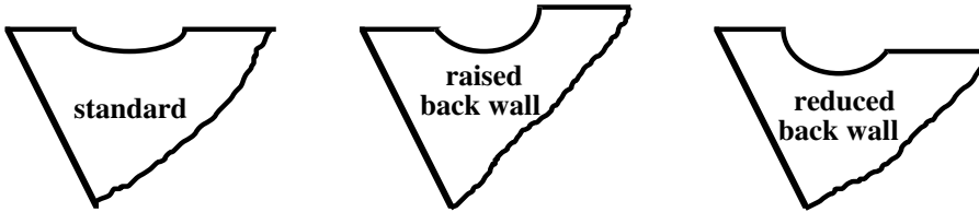
FIGURE 6.16 Illustration of common chip breakers.
