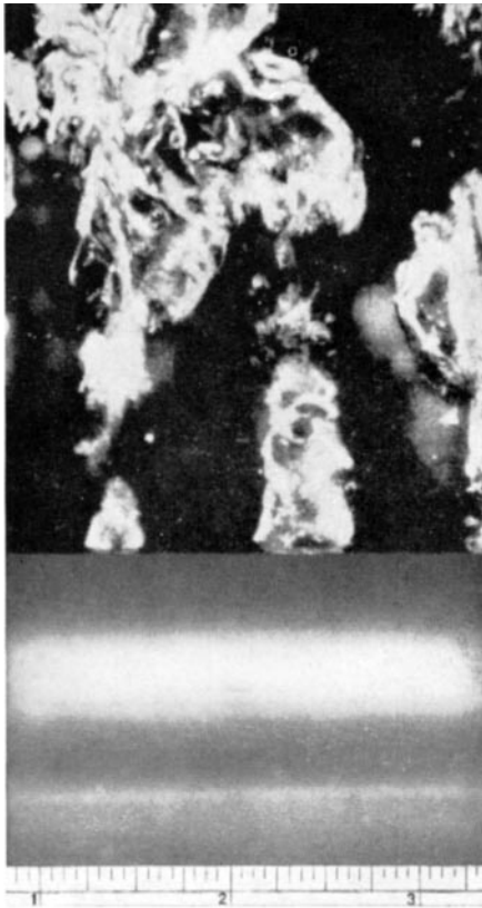
FIG. 14-95b Comparison of bubbles from a porous septum and from a perforated-pipe sparger. Air in water at 70°F. Karbate pipe perforated with 1/16-in holes on 1-in centers. (National Carbon Co.) To convert inches to centimeters, multiply by 2.54; °C = 5/9 (°F - 32).
