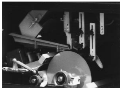
FIG. 19-60 Internal configuration of roll-type electrostatic separator, ionizing mode. (Courtesy Carpcop, Inc.)
