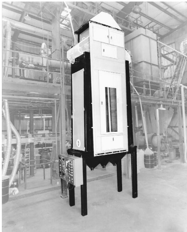
FIG. 19-57 Triboelectric separators. V-Stat electrostatic separator for silica removal from industrial minerals. (Courtesy of Carpco, Inc.)
