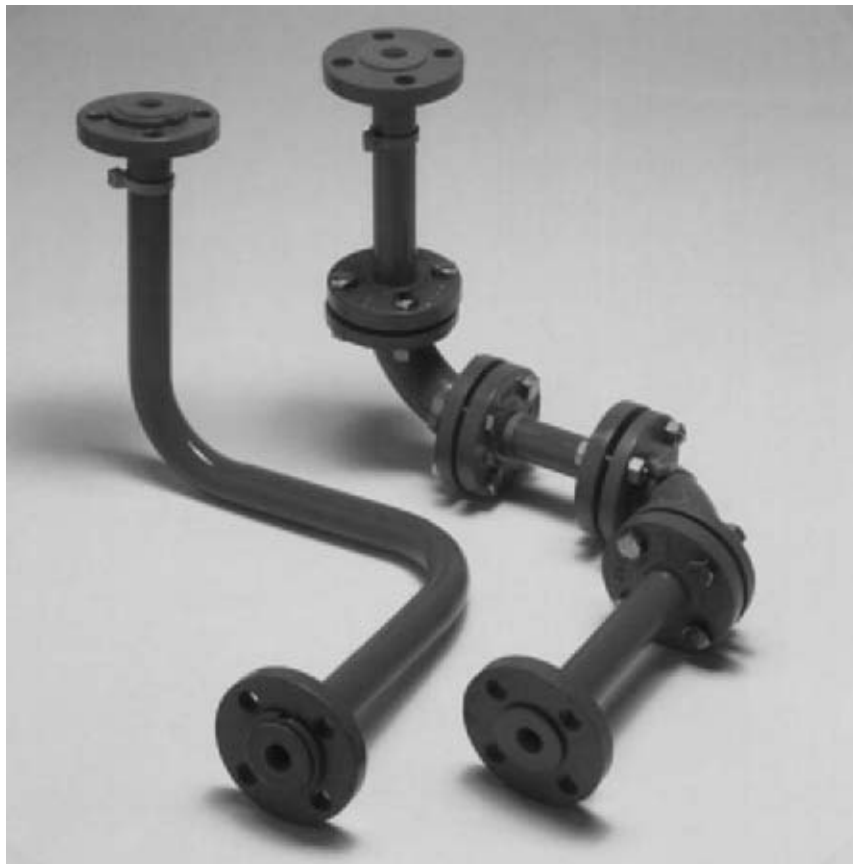
FIGURE B12.9 Illustration showing the flange-reduction possibilities of precision-bent plastic-lined pipe as compared with traditional flanged piping (Courtesy of Crane Resistoflex).
