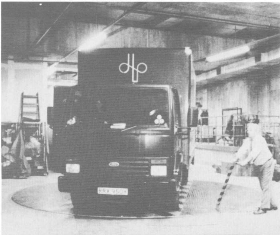
FIGURE 3 – Air film vehicle turntable. The turntable sits in a shallow pit, 150 mm deep, allowing up to 20 tonnes to be rotated by hand. ( Hovair Systems )
