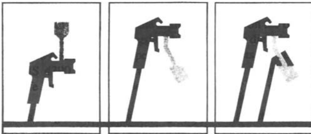
FIGURE 1 – Different paint feed. Left: gravity feed. Middle: suction feed. Right: pressure feed.
