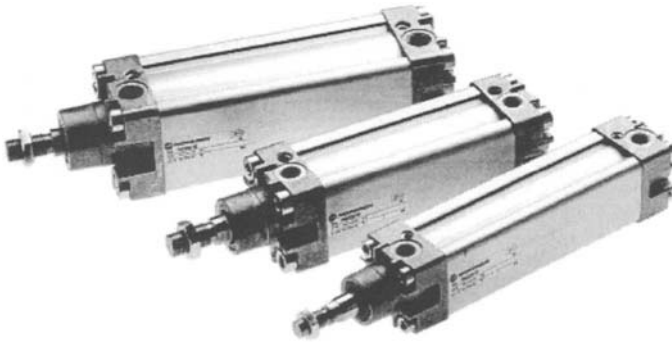
FIGURE 4 – Light duty cylinders to ISO 6431. Cylinder body in aluminium alloy, piston rod in stainless steel, die cast aluminium end caps. End caps attached by steel screws. ( Norgren )
