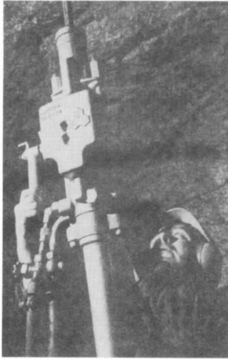
FIGURE 2 – Stoper drill. ( CompAir Holman )
