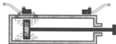
Magnetic sensors mounted on the cylinder
