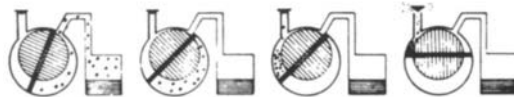
Vane pump working without gas ballast (condensed water vapour remaining over a certain level if partial evacuation is needed).
