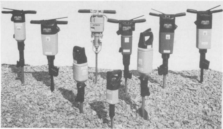
FIGURE 4 – A range of contractors' percussive tools. Left to right: 2 road breakers, a medium duty pick, a light weight rock drill with rotation, a light pick, a light road breaker, a road breaker with a 'D' handle, two road breakers. Note the numbers 108, 111 on the bodies, which are the sound power levels to satisfy EC regulations. ( CompAir Holman )
