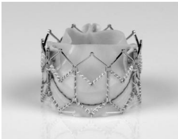
Figure 20.1 The SAPIEN XT is a balloon-expandable transcatheter heart valve. The valve incorporates bovine pericardial leaflets and a fabric sealing cuff sewn to a cobalt chromium tubular frame.
