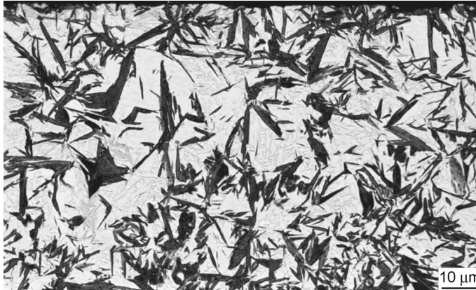
FIGURE 7.17 Plate martensite and retained austenite in the case (14NiCr18, 1.0% C, 60% retained austenite). (From O. Schwarz, J. Grosch, C. Genzel, W. Reimers, Härterei Techn. Mitt. 49:134, 1994.)
