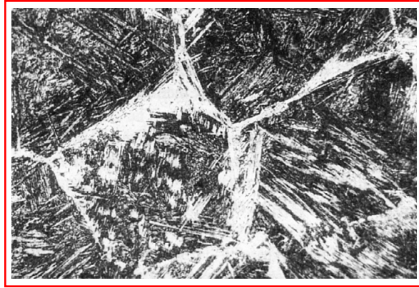
FIGURE 3.5 Steel microstructure of secondary cementite (needles) and pearlite, 500 \times .
