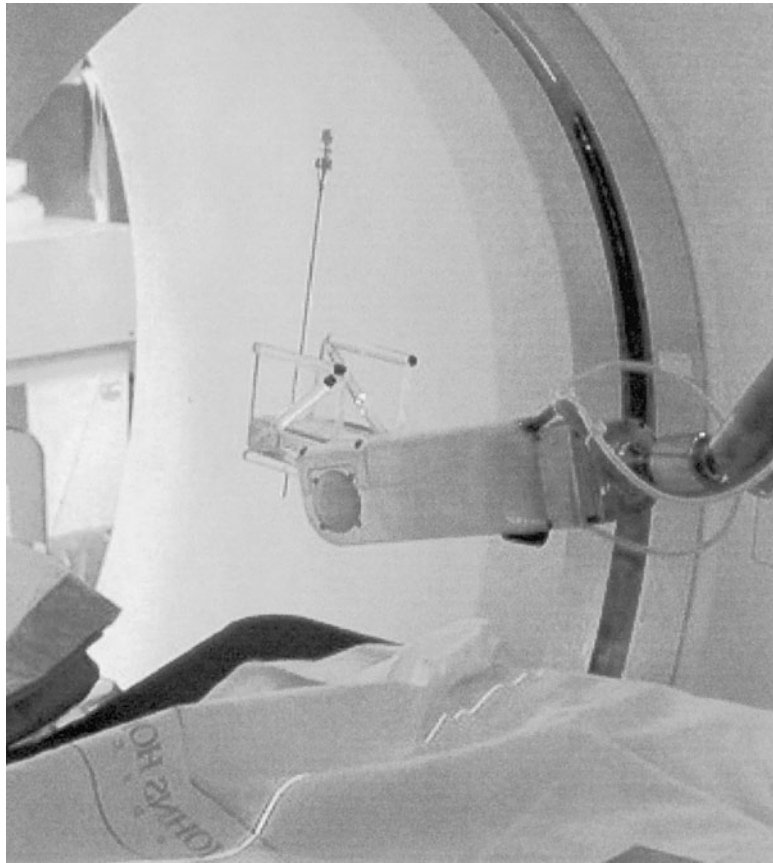
FIGURE 14.11 RCM robot with radiolucent CT-compatible needle driver. 42,44,45
