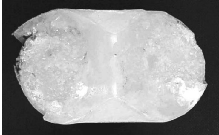
FIGURE 22.3 Severe wear of a total knee insert. 28
