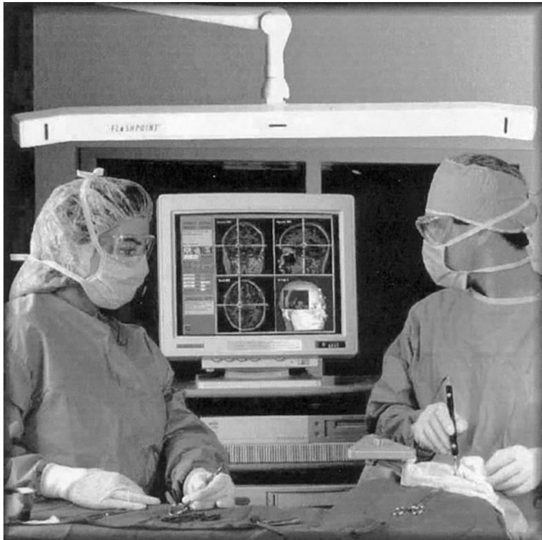
FIGURE 14.2 A CIS navigation system in action. The surgeon (left) is performing a brain tumor biopsy with the help of a navigation system. He is holding a pointer with light-emitting diodes whose position and orientation is precisely determined in real time by a stereo tracking camera (top). The computer display (center) shows the preoperative MRI and the current position of the pointer. The image shows three orthogonal cross sections and a three-dimensional reconstruction of the MRI data. The cross hair in each view shows the position of the pointer. The surgeon moves the pointer toward the desired position by watching the pointer location move on the screen.
