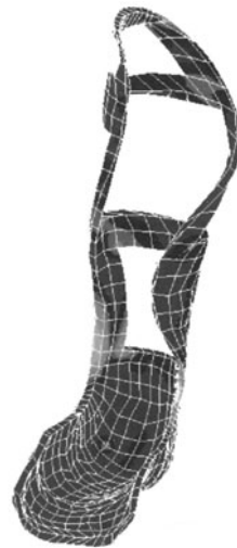
FIGURE 16.11 FEM of an ankle-foot orthotic after weight reduction. (Reprinted with permission of Khamis Abu-Hasaballah and the University of Hartford.)
