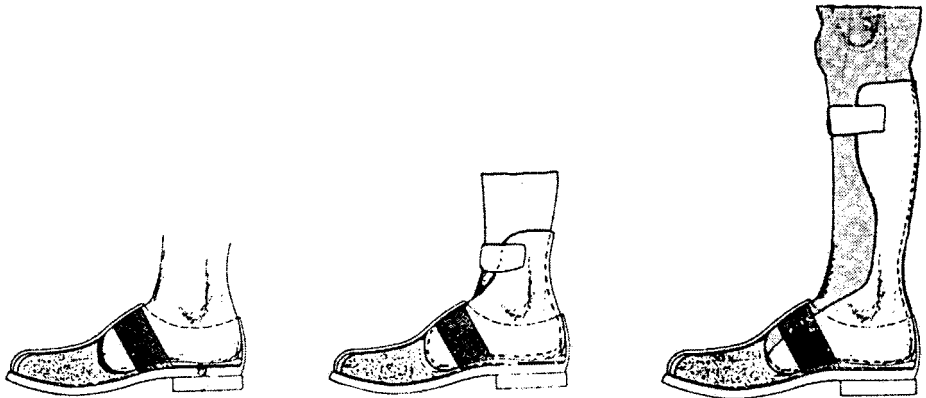
FIGURE 21.7 Prostheses for partial foot amputation: transmetatarsal amputation or amputations resulting in an intact functional ankle ( left ), Lisfranc or amputations resulting in an ankle requiring some support ( center ), and Chopart amputation or amputations resulting in an unstable ankle ( right ). (Adapted from Ref. 4, Fig. 4.3.)
