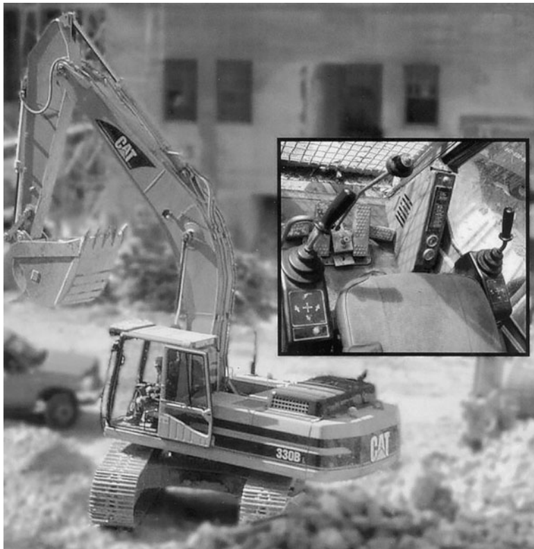
FIGURE 20.1 A digger, or backhoe, is essentially a large mechanical arm. To control this arm, an operator needs to use both hands (to operate the joysticks, see inset), both feet (to operate multiple pedals), both eyes, and almost all of their concentration (to watch what they are doing). These are the requirements for a “whole” individual to control just one artificial arm. Consider now the control problems experienced by a person who has lost both arms at the shoulder. These individuals do not have hands to help in the control of their artificial arms, their feet are needed for walking, and the mental burden placed on the person to control their prosthetic arms cannot be so great that controlling their prostheses takes more effort than it is worth. ( Many thanks to Mr. John Marbes of American Demolition for taking me on to the job site and allowing me to take these pictures. )
