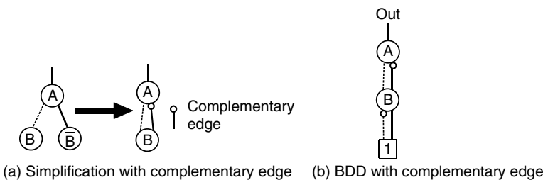
FIGURE 2.36 BDD with complementary edges for function in Fig. 2.35.
