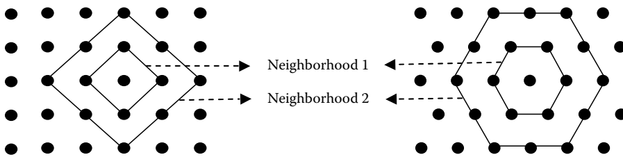
FIGURE 18.1 The SOM grid structure: (a) rectangular grid and (b) hexagonal grid.
