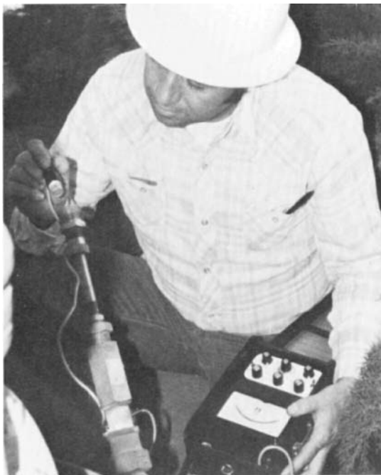
FIG. 20.22 Operator connecting a corrosion meter to a permanently installed probe to read corrosion rate of the probe material in the system. (Courtesy of Rohrbach Corporation.)
