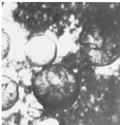
FIG. 12.31 Gel-type resin containing a large amount of loose precipitate, indicating improper backwash. This condition is responsible for most problems with ion exchange systems.
