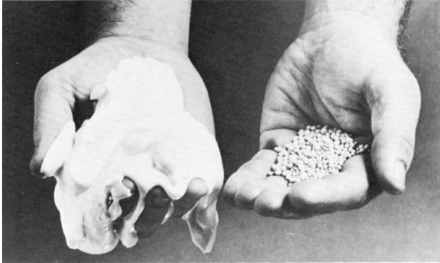
FIG. 10.8 (c) Left , typical lime softener sludge; right , pellets produced by granular bed softener. (Courtesy of the Permutit Company.)
