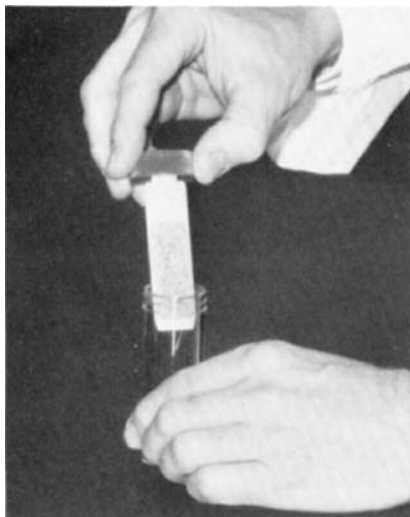
FIG. 7.28 Microbes are collected and cultured by pretreated elements which are easily incubated. The sampler has a fine grid printed on it to facilitate counting of colonies. (Courtesy Millipore Corporation.)
