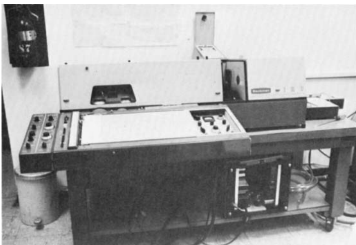
FIG. 7.40 The infrared analyzer differentiates the functional groups on organic molecules extracted from water.
