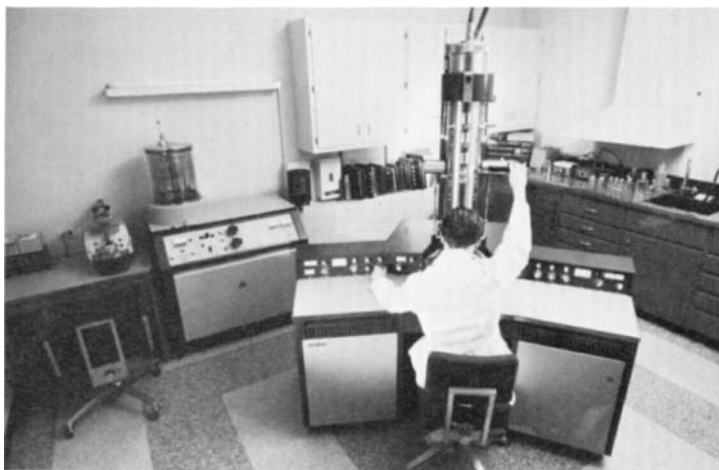
FIG. 7.35 A view of the components of a transmission electron microscope.
