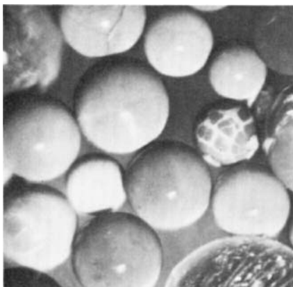
FIG. 12.33 Inorganically fouled gel-type resin showing both external and internal fouling. Barium and strontium frequently contribute to this problem in units regenerated with H_2SO_4 .
