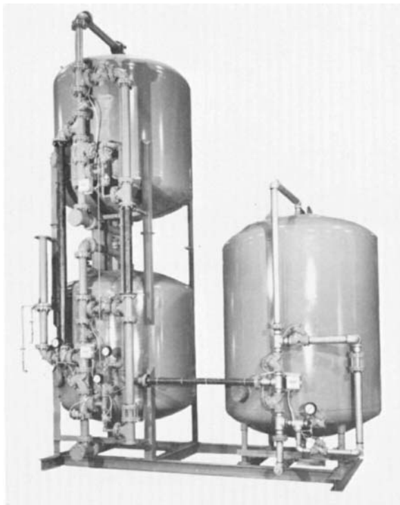
FIG. 17.6 This activated carbon filter ( right ) is used for the removal of organic matter and free chlorine. Two mixed media filters remove suspended solids to protect the carbon from fouling. ( Courtesy of Illinois Water Treatment Company. )
