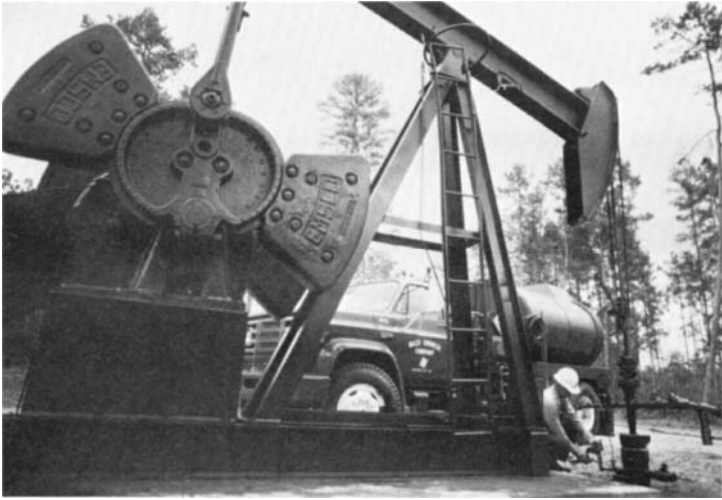
FIG. 43.6 This oil well pump is a walking beam unit. Submersible centrifugal units are also commonly used.
