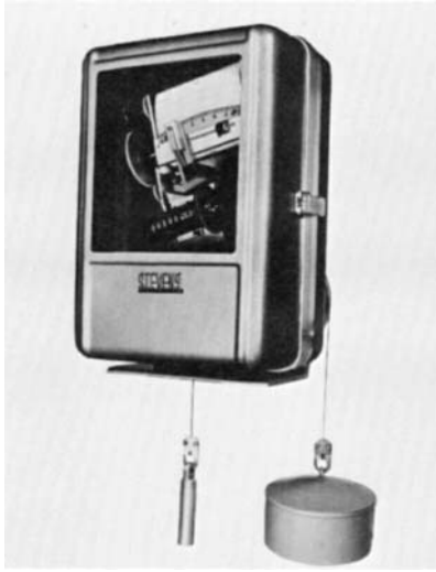
FIG. 7.16 Typical level measuring devices for measuring flows over weirs and flumes. (Courtesy Leupold & Stevens, Inc.)
