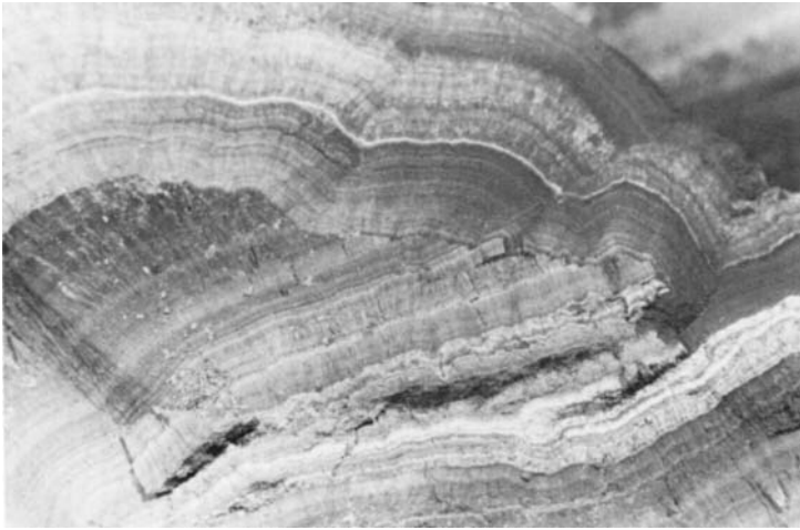
FIG. 21.1 Laminar nature typical of most deposits, indicating variations in the environment. Analysis of each layer is sometimes required to determine all of the reasons for deposit formation.
