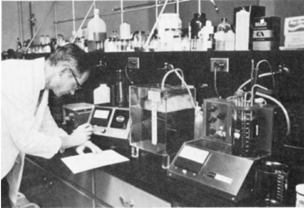
FIG. 40.9 Bench-scale biological studies require frequent attention to observation and recording of data during and following the period of acclimatization.
