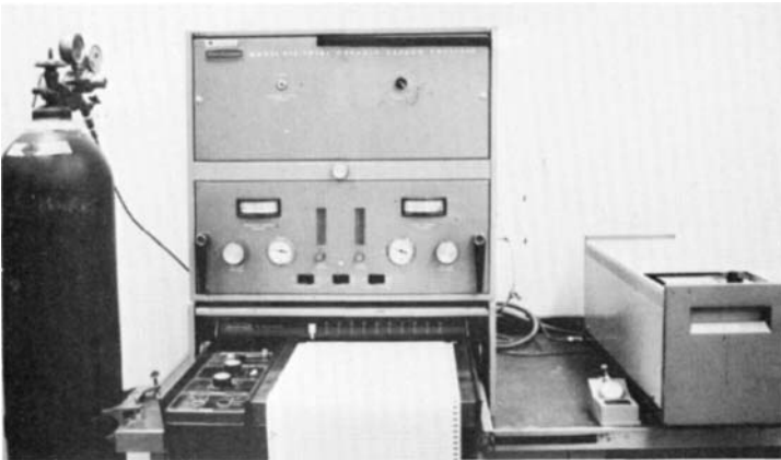
FIG. 7.39 Total carbon analyzer in use for determining organic matter in water.
