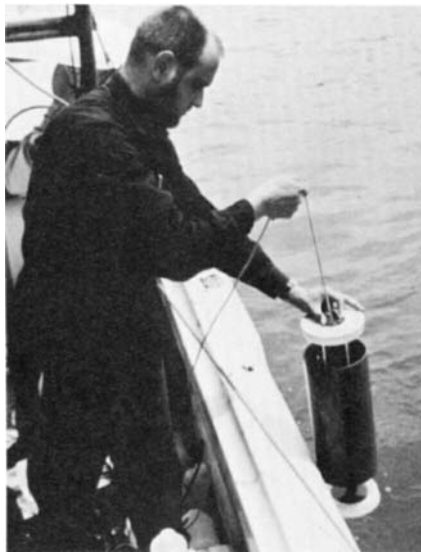
FIG. 7.23 The sampler used for surface water studies is tripped to close at predetermined depth.
