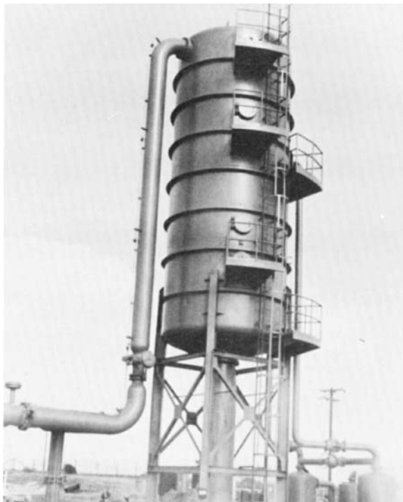
FIG. 14.7 Vacuum deaerator at an oil production operation. (Courtesy of L*A Water Conditioning Company.)
