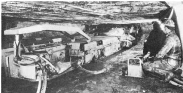
FIG. 29.1 This continuous coal-mining machine is equipped with water spray nozzles to suppress dust at the working surface. (Courtesy of Lee-Norse Company.)
