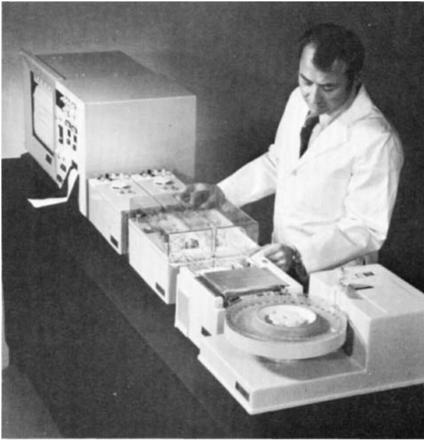
FIG. 7.38 An automatic device for wet analysis of a battery of samples. (Courtesy Technicon Instruments Corporation.)
