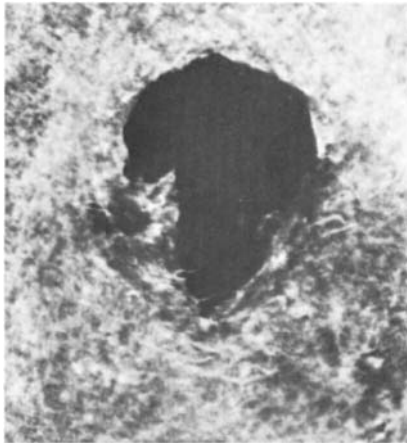
FIG. 30.27 Sheet imperfections are caused by sloughing of slime mass into machine system. In this photo, the removal of the slime mass during calendering left a hole in the sheet.
