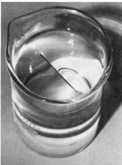
FIG. 1.2 A steel needle, with a density about 7 times that of water, can be made to float because of water's high surface tension.
