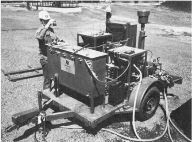
FIG. 23.21 Pilot plant designed for biological digestion studies on fresh wastewater at a plant site. This unit can be operated in a variety of modes, including extended aeration, step aeration, and contact stabilization.
