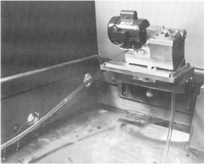
FIG. 11.17 Free oil is often collected from water surfaces in a separation tank by means of an endless belt or loop made of oil-wettab plastic. (Courtesy of Oil Skimmers Inc.)
