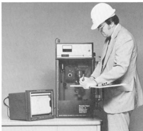
FIG. 39.6 This instrument is used to monitor corrosion-produced hydrogen concentrations in steam.
