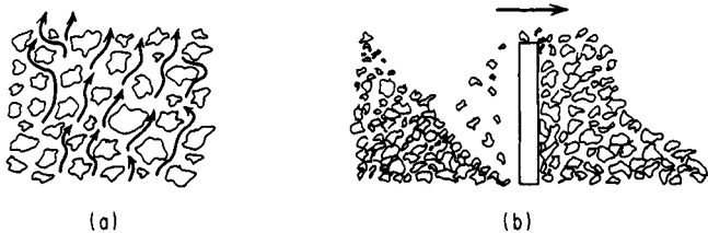
FIG. 9.6 (a) Hindered settling is reached as particulates become so close to each other that the passages between them restrict the ability of water to escape from the sludge. (b) Compaction occurs naturally, but slowly, by gravity and by dehydration of the particulates; it is aided by gently moving the sludge to develop crevices behind the moving pickets or scraper blades for water release.
