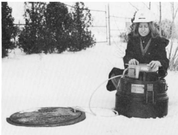
FIG. 7.25 A programmed sampler obtaining intermittent sewage samples.
