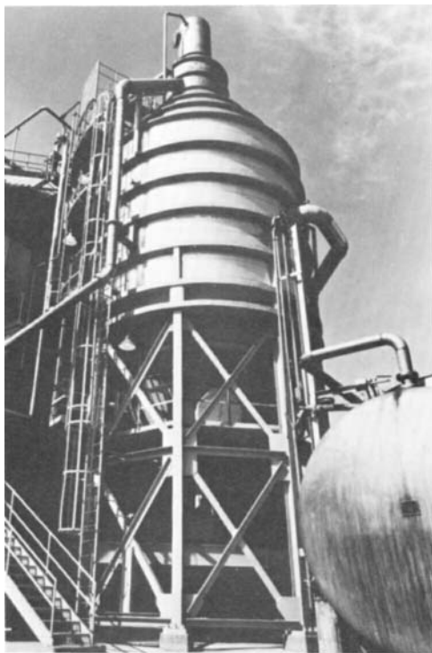
FIG. 26.3 Energy changes accompany many chemical separation processes, requiring heating or cooling of the process liquor. In this large crystallizer, ammonium sulfate is produced at a rate of 600 tons/day. (Courtesy of Whiting Corporation.)
