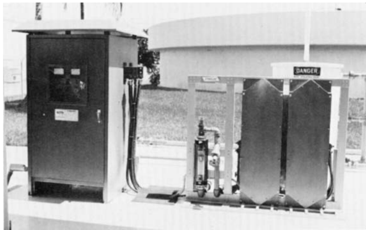
FIG. 22.9 An electrolytic cell designed to produce chlorine from brine. This unit is generating \text{Cl}_2 from seawater for chlorination of sewage plant effluent. (Courtesy of Electrolytic Systems Division, Diamond Shamrock.)
