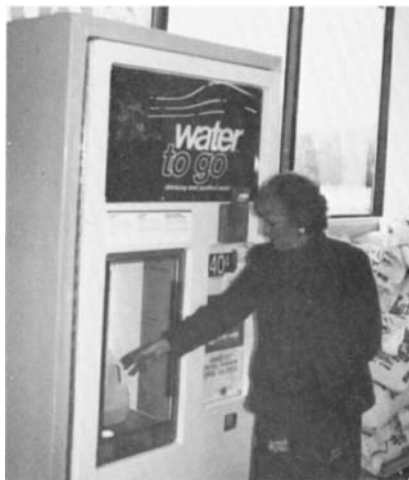
FIG. 35.8 Bottled water dispenser with integral treatment units, used in various combinations to produce potable water or low solids water comparable in many respects to distilled water.
