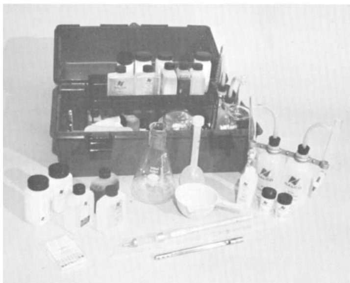
FIG. 7.26 One type of portable laboratory used for field and plant surveys and for monitoring services.
