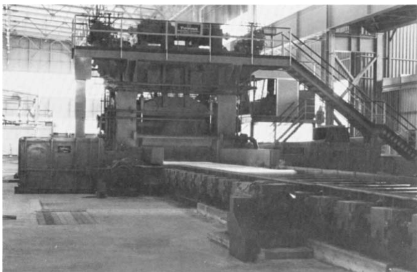
FIG. 32.12 Hot mill rolling plate for further reduction through a hot strip mill. (Courtesy of Tippins Machinery Company, Inc.)
