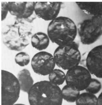
FIG. 12.32 Badly cracked gel-type resin. This may be caused by internal precipitate or osmotic shock, the latter being rather common in hot zeolite units if pressure is suddenly released.
