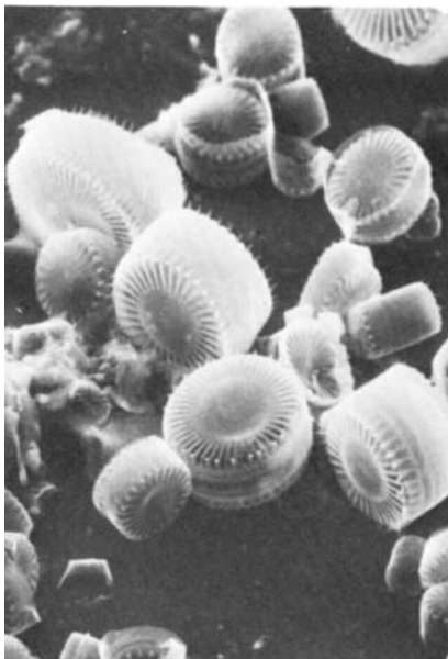
FIG. 7.36 Diatoms and silt observed by the scanning electron microscope at 1000 \times magnification.
