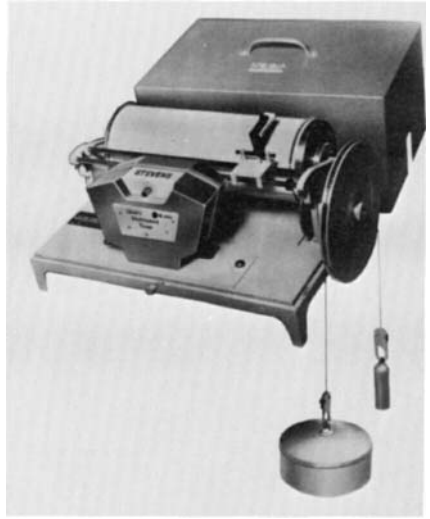
FIG. 7.16 Typical level measuring devices for measuring flows over weirs and flumes. (Courtesy Leupold & Stevens, Inc.)
