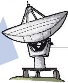
Local User Terminals (LUTs) receive signals from the satellites and alert mission control
