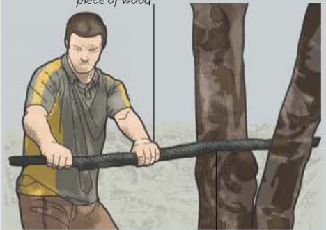
Place the wood between two trees—one is a stop or buffer, the other is a leverage point
