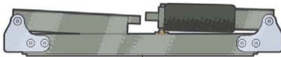
The tension frame and saw blade can usually be taken apart and stowed safely
