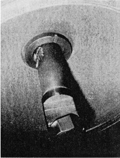
Figure 3-48. Bent Valve Stem with Damage to Stem Surface Resulting from Attempted Closure of Wedge Gate Valve with Wedge Rotated and Jammed in Valve Body, Size DN 300 (NPS 12) Class 150. (Courtesy of David Mair.)
