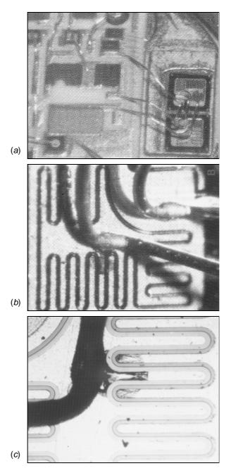
**Figure 3.28** Three views of a hybrid voltage regulator that failed because of a damaged pass transistor: (*a*) the overall circuit geometry; (*b*) a closeup of the damaged pass transistor area; (*c*) an enlarged view of the damage point.
