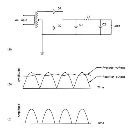
**Figure 4.12** Characteristics of a capacitive input filter circuit: (*a*) schematic diagram, (*b*) voltage waveshape across input capacitor, (*c*) waveshape of current flowing through diode.
