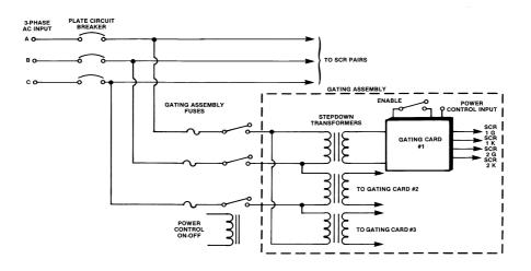
**Figure 4.24** Simplified block diagram of the gating circuit for a phase-control system using back-to-back SCRs.
