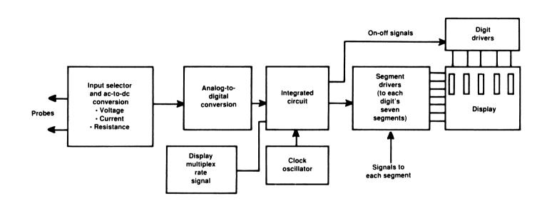
**Figure 1.76** Block diagram of a basic digital voltage and current measuring device. It should be noted that advances in integrated circuit technology have reduced most of the individual elements shown to single device.
