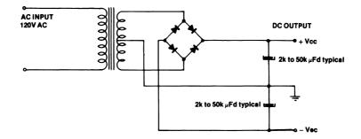
Figure 4.1 Conventional capacitor input filter full-wave bridge.
