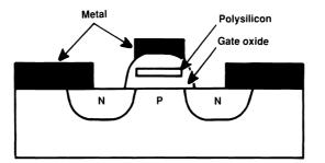
Figure 3.18 Construction of a silicon gate NMOS transistor. (After [1].)
