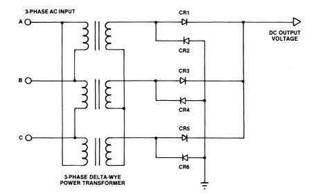
Figure 4.3 Three-phase, delta-connected high-voltage rectifier.
