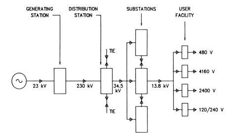
**Figure 1.7** A typical electrical power-generation and distribution system. Although this schematic diagram is linear, in practice power lines branch at each voltage reduction to establish the distribution network. (*From* [5]. *Used with permission*.)
