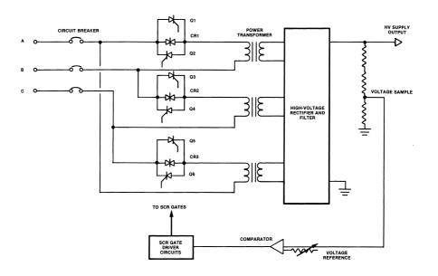
Figure 4.22 Thyristor-controlled high-voltage servo power supply.
