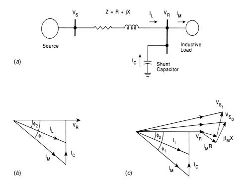
**Figure 1.66** Shunt-capacitor compensation: (*a*) schematic diagram; (*b*) current phasor diagram; (*c*) voltage phasor diagram. (*From* [17]. *Used with permission*.)
