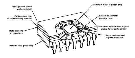
**Figure 3.25** Cutaway view of a DIP integrated circuit package showing the internalto-external interface. (*After* [1].)
