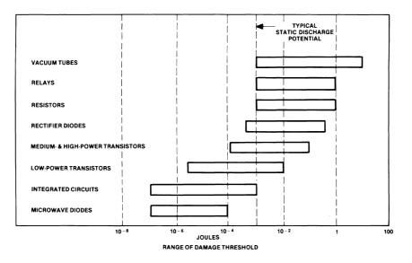
**Figure 2.37** An estimation of the susceptibility of common electric devices to damage from transient disturbances. The vertical line marked "discharge" represents the energy level of a discharge that typically can be generated by a person who touches a piece of equipment after walking across a carpeted floor.
