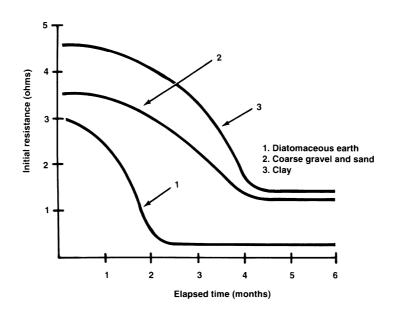
Figure 7.14 Measured performance of a chemical ground rod. (After [10].)
