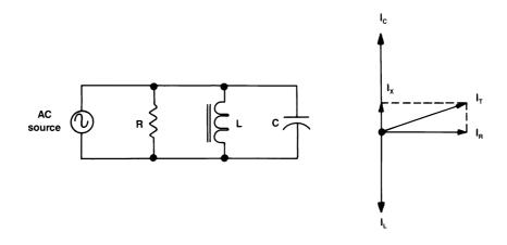
Figure 1.2 Current vectors in a parallel RLC circuit.
