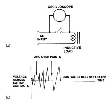
**Figure 2.22** The mechanics of contact bounce: (*a*) measurement configuration; (*b*) representative waveforms. The waveforms shown are exaggerated to illustrate the transient effects. For clarity, the modulating effect of the ac line voltage is not shown.
