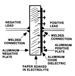
**Figure 4.34** The basic design of an aluminum electrolytic capacitor.
