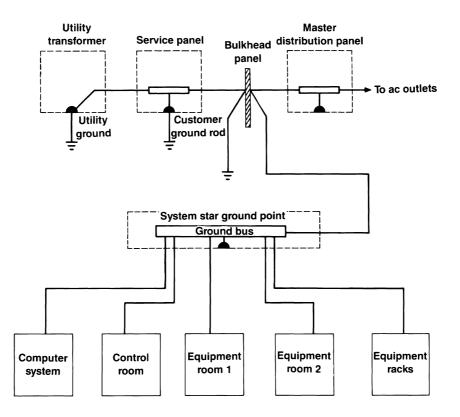
**Figure 7.62** Equivalent ground circuit diagram for a medium-sized commercial/industrial facility.
