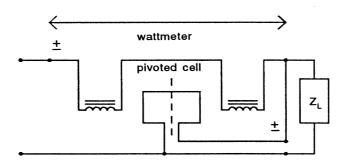
Figure 1.74 A wattmeter connected to a load. (From [17]. Used with permission.)
