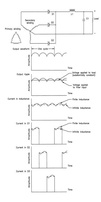
**Figure 4.11** Voltage and current waveshapes for an inductive input filter driven by a three-phase supply.
