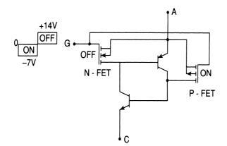
Figure 4.28 The equivalent circuit of the MCT device. (After [4] and [5].)
