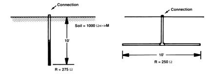
Figure 7.8 The effectiveness of vertical ground rods compared with horizontal ground rods. (*After* [10].)
