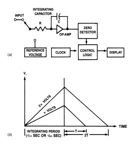
**Figure 1.77** The analog-to-digital conversion process: (*a*) the basic circuitry involved; (*b*) graph of  $V_c$  versus time. Because the slope of the discharge curve is identical regardless of the ultimate voltage reached by the integrator, the discharge period and, therefore, the number of counts recorded by the logic circuitry are proportional to the input voltage.
