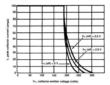
**Figure 3.2** Reverse bias safe operating area curve for a bipolar transistor (MJH10610A). (*Courtesy of Motorola*.)
