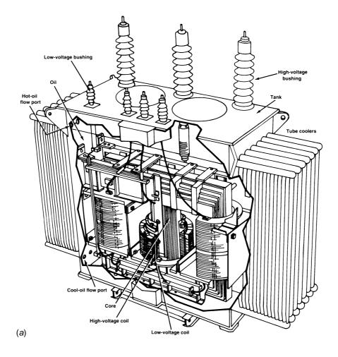
**Figure 1.11** Construction of an oil-filled three-phase power transformer used for commercial power distribution: (*a*) cutaway view; (*b*, next page) exterior view. (*Drawing* b from [14]. Used with permission.)
