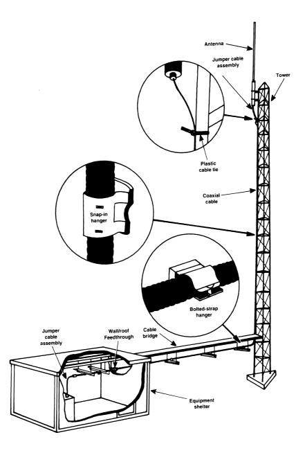
Figure 7.30 Transmission-line mounting and grounding procedures for a communications site.
