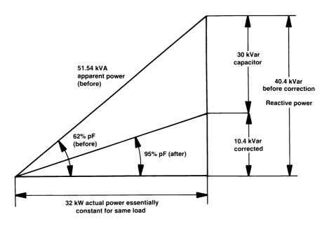
Figure 1.67 Illustration of the results of on-site power factor correction.
