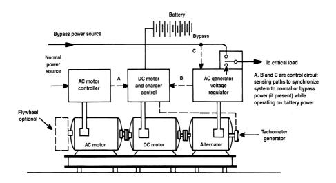
Figure 5.12 Uninterruptible m-g set with ac and dc motor drives. (After [2].)
