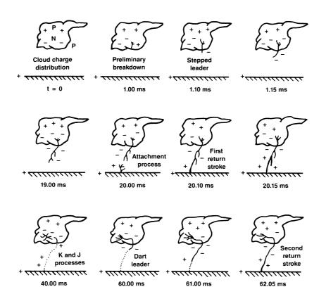
Figure 2.6 The mechanics of a lightning flash. (After [2].)
