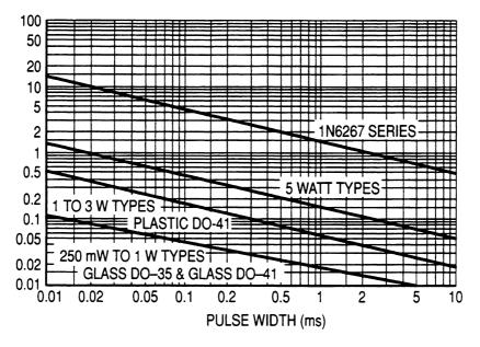
Figure 6.9 Peak power ratings of common zener diodes. (Courtesy of Motorola.)
