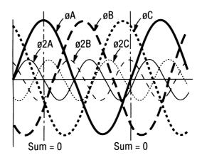
**Figure 2.29** Fundamental and 2<sup>nd-</sup>harmonic currents in a 3-phase, 4-wire circuit. At any point, the sum of the positive (+) and negative (–) currents equals zero for the fundamental current, the 2<sup>nd-</sup>harmonic current, and—in similar fashion—all even-harmonic currents. Therefore, for balanced loads on a 3-phase, 4-wire system, no 60 Hz or even-harmonic currents flow in the common neutral. (*From* [5]. *Used with permission*.)
