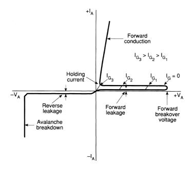
Figure 4.13 Volt-ampere characteristics of a thyristor. (After [4] and [5].)
