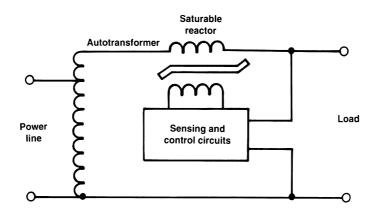
Figure 5.43 Autotransformer/saturable reactor voltage regulator.
