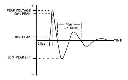
**Figure 2.38** The suggested ANSI/IEEE indoor-type transient overvoltage test waveform (0.5 µs–100 kHz ring wave, open-circuit voltage).
