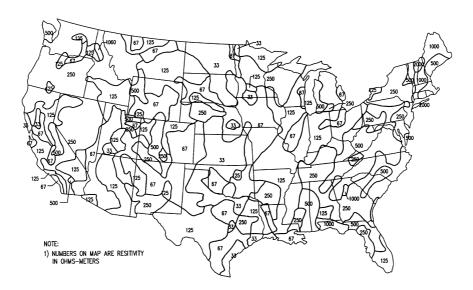
Figure 7.10 Typical soil resistivity map for the U.S. (From [11]. Used with permission.)
