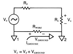
**Figure 7.65** An unbalanced system in which each piece of equipment has one of its connections tied to ground.
