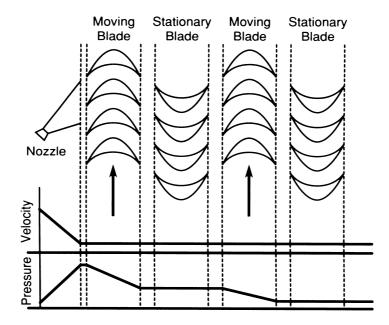
Figure 1.36 Velocity and pressure variation in an impulse turbine. (From [7]. Used with permission.)
