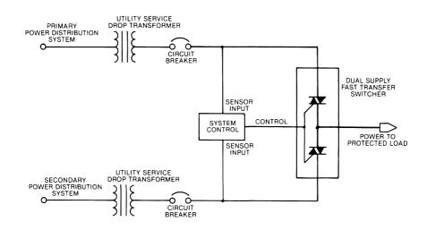
**Figure 8.3** The dual utility feeder system of ac power loss protection. An automatic transfer switch changes the load from the main utility line to the standby line in the event of a power interruption.
