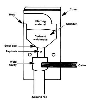
**Figure 7.21** Typical exothermic bonding mold for connecting a cable to a ground rod. (*After* [9].)
