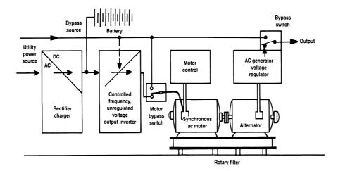
Figure 5.14 Uninterruptible m-g set using a synchronous ac motor. (After [2].)
