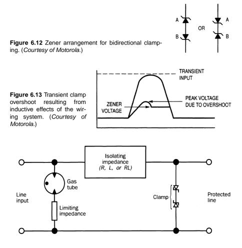
Figure 6.14 A two-stage hybrid protection circuit.
