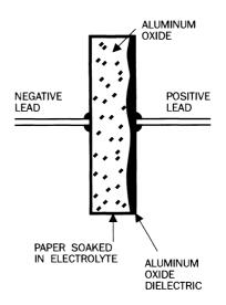
**Figure 4.36** Failure mechanism of a leaky aluminum electrolytic capacitor. As the device ages, the aluminum oxide dissolves into the electrolyte, causing the capacitor to become leaky at high voltages.
