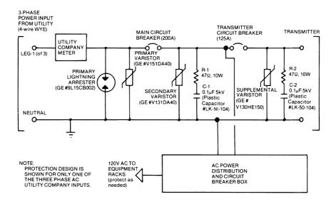
**Figure 6.27** The application of transient-suppression components in a systemwide protection plan. Install such hardware with extreme care, and only after consultation with the local utility company and an electrical contractor.
