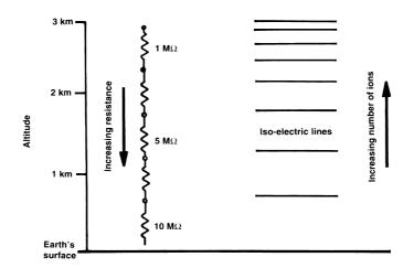
Figure 2.2 The effects of atmospheric conductivity.
