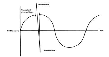
**Figure 2.25** The "iceberg" effect of many transient waveforms. The overshoot often is followed by an equally damaging undershoot before leveling off.
