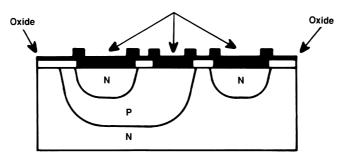
Figure 3.19 Construction of a bipolar transistor. (After [1].)
