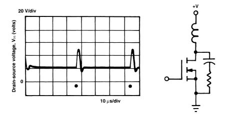
Figure 3.12 Drain-source transient with an *RC* snubber circuit. (*Courtesy of Motor-ola*.)
