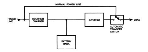
Figure 5.19 Forward-transfer UPS system.
