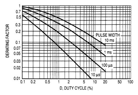
Figure 6.10 Typical derating factor for zener duty cycle. (Courtesy of Motorola.)
