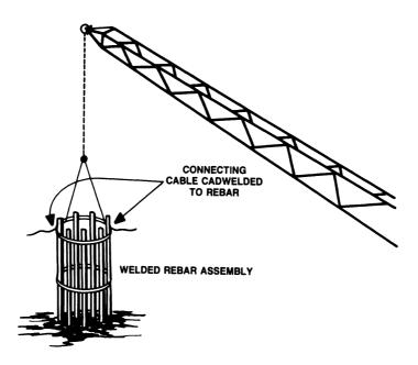
**Figure 7.18** The Ufer ground system as applied to a transmission-tower base or guywire anchor point. When using this type of ground system, bond all rebar securely to prevent arcing in the presence of large surge currents. (*After* [9].)
