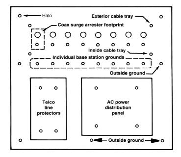
Figure 7.40 Mounting-hole layout for a communications site bulkhead subpanel.
