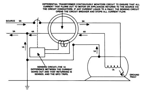
Figure 9.4 Basic design of a ground-fault current interrupter (GFCI).
