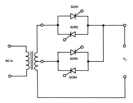
Figure 5.55 Secondary-side synchronous tap-changing transformer.
