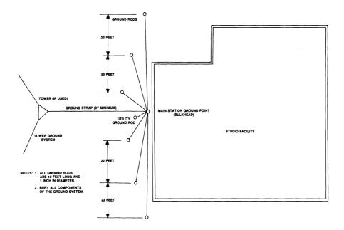
**Figure 7.33** A facility ground system using the hub-and-spoke approach. The available real estate at the site will dictate the exact configuration of the ground system. If a tower is located at the site, the tower ground system is connected to the building ground as shown.
