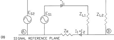
**Figure 7.70** The equipotential plane: (*a*) individual signal sources, (*b*) net effect on the signal reference plane. (*From* [5]. *Used with permission*.)
