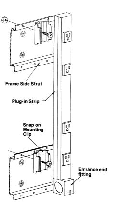
Figure 7.61 Rack mounting detail for an insulated-shell ac power strip.
