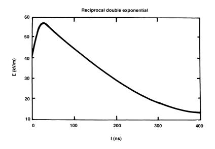
Figure 2.4 Discharge waveform for a typical lightning strike.
