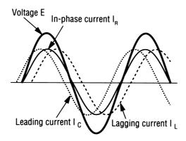
**Figure 2.26** The relationship of linear current waveforms:  $I_R$  is a purely resistive circuit current,  $I_L$  is a partially inductive (lagging) circuit current, and  $I_C$  is a partially capacitive (leading) circuit current. (*From* [5]. Used with permission.)
