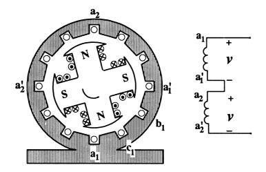
**Figure 1.29** A four-pole synchronous machine: (*a*) cross-section of the machine; (*b*) schematic diagram for the phase *a* windings. (*From* [5]. *Used with permission*.)
