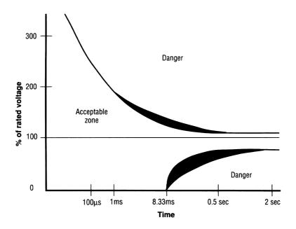
**Figure 5.5** A simplified version of the CBEMA curve. Voltage levels outside the *acceptable zone* results in potential system shutdown and hardware and software loss. (*From* [2]. *Used with permission*.)
