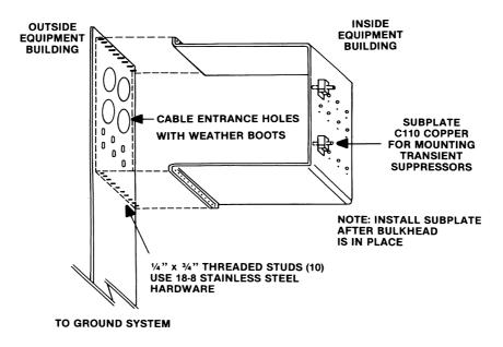
**Figure 7.39** The addition of a subpanel to a bulkhead as a means of providing a mounting surface for transient-suppression components. To ensure that the bulkhead is capable of handling high surge currents, use the hardware shown. (*After* [9].)
