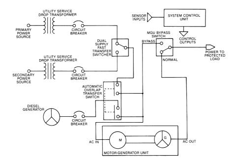
**Figure 8.7** A premium power-supply backup and conditioning system using dual utility company feeds, a diesel generator, and a motor-generator set. An arrangement such as this would be used for critical loads that require a steady supply of clean ac.
