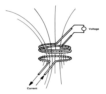
Figure 1.8 The basic principles of electromagnetic induction.
