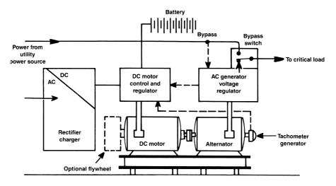
Figure 5.13 Uninterruptible m-g set using a single dc drive motor. (After [2].)
