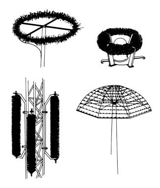
Figure 2.8 Various types static dissipation arrays.
