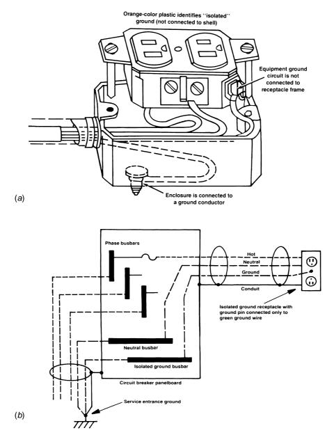
**Figure 6.26** Installation requirements for an orange receptacle ac outlet: (*a*) mechanical configuration (note that at least two ground conductor paths are required—one for the receptacle ground pin and one for the receptacle enclosure); (*b*) circuit arrangement for the isolated ground outlet; (*c*, next page) circuit arrangement for a conventional ac outlet. (*After* [1].)
