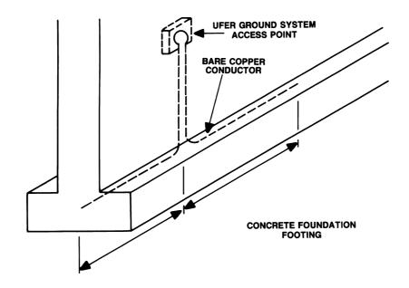
**Figure 7.17** The basic concept of a Ufer ground system, which relies on the moisture-retentive properties of concrete to provide a large earth-to-electrode interface. Design of such a system is critical. Do not attempt to build a Ufer ground without the assistance of an experienced contractor. (*After* [9].)
