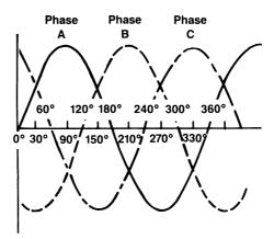
**Figure 1.27** Output waveform of a three-phase generator.
