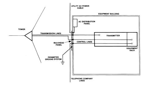
**Figure 7.38** The basic design of a bulkhead panel for a facility. The bulkhead establishes the grounding reference point for the plant.
