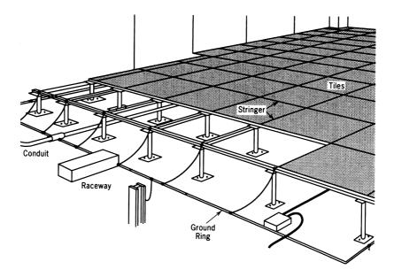
Figure 7.53 Grounding plan for a raised-floor support system.
