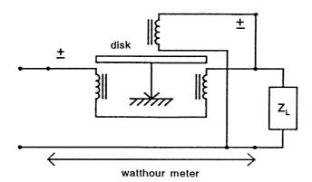
Figure 1.75 A watt-hour meter connected to a load. (From [17]. Used with permission.)
