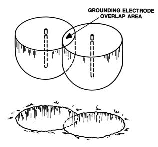
**Figure 7.6** The effect of overlapping earth interface hemispheres by placing two ground rods at a spacing less than 2.2 times the length of either rod. The overlap area represents wasted earth-to-grounding electrode interface capability. (*After* [10].)
