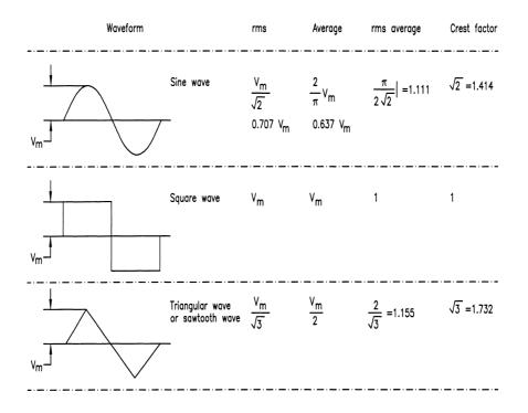
Figure 2.43 Comparison of rms and average voltage characteristics.
