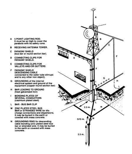
Figure 7.37 Grounding a small microwave transmission tower.
