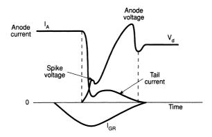
Figure 4.25 Turn-off characteristics of a GTO. (After [4] and [5].)
