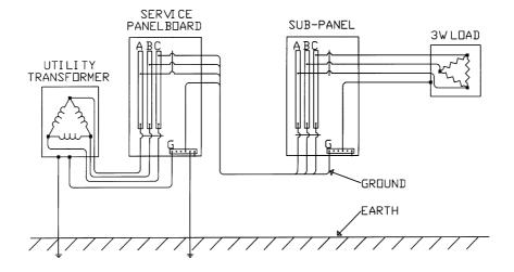
Figure 7.3 Ungrounded delta power system. (From [5]. Used with permission.)
