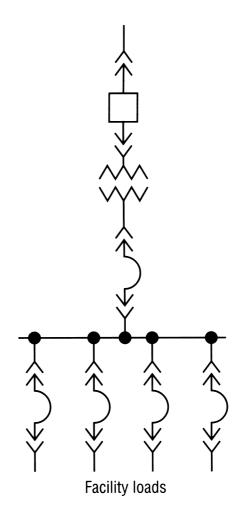
**Figure 8.15** Secondary plant distribution using a simple radial configuration. (*From* [5]. Used with permission.)
