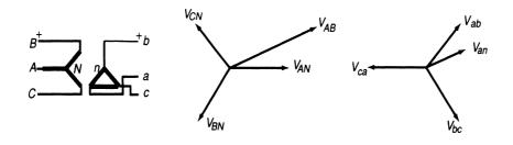
**Figure 1.20** Y- $\Delta$  transformer with the primary side lagging the secondary side by 30°. (*From* [3]. *Used with permission*.)
