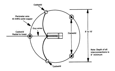
**Figure 7.26** Top view of proper guy-anchor grounding techniques. A properly dressed and installed ground wire prevents surge currents from welding turnbuckles and damaging safety loops. The perimeter ground connects to the tower base by way of a radial wire. (*After* [9].)
