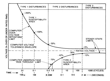
**Figure 5.1** The recommended voltage tolerance envelope for computer equipment. This chart is based on pioneering work done by the Naval Facilities Engineering Command. The study identified how the magnitude *and* duration of a transient pulse must be considered in determining the damaging potential of a spike. The design goals illustrated in the chart are recommendations to computer manufacturers for implementation in new equipment. (*After* [1].)
