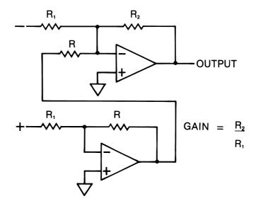
**Figure 7.76** An active-balanced input circuit using two op-amps; one to invert the positive input terminal and the other to buffer the difference signal. Without adjustments, this circuit will provide about 50 dB CMRR.
