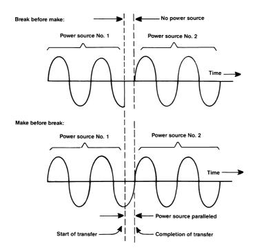
Figure 5.38 Static transfer switch modes.
