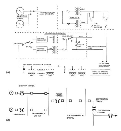
**Figure 1.47** Simplified block diagram of a basic utility company power distribution system: (*a*) Overall network. The devices shown as fuses could be circuit breakers or reclosers. All circuits shown are three-phase. The capacitors perform power factor correction duty. (*b*) System terminology. (*c*, next page) Distinction between the primary and secondary distribution systems. (b *and* c *from* [3]. Used with permission.)
