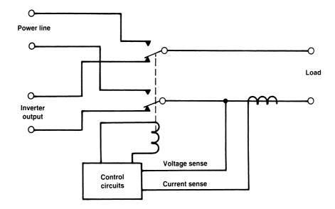
Figure 5.21 Electromechanical load-transfer switch.
