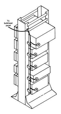
Figure 7.63 Ground bus for an open-frame equipment rack.
