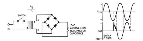
**Figure 2.19** Transient produced as a result of transformer capacitance during poweron condition. (*After* [4].)
