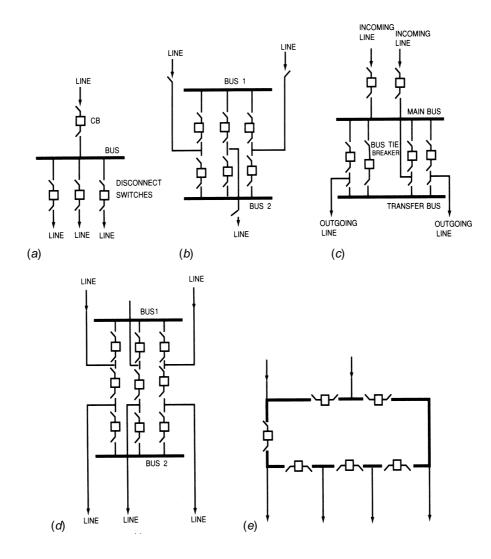
**Figure 1.52** Substation bus and breaker arrangements: (*a*) single-bus; (*b*) double-bus/double-breaker; (*c*) main-and-transfer bus; (*d*) breaker-and-a-half; (*e*) ring bus. (*From* [3]. *Used with permission*.)
