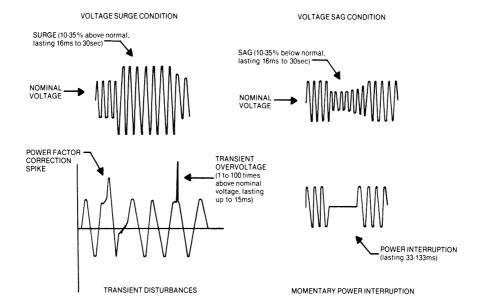
Figure 2.36 The four basic classifications of short-term power-line disturbances.
