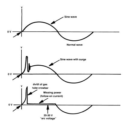
Figure 6.4 The power-follow effect of a crowbar device.
