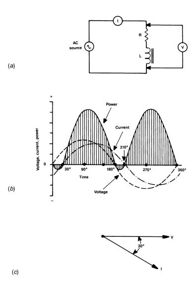
**Figure 1.13** Resistive-inductive circuit: (*a*) circuit diagram; (*b*) representative waveforms; (*c*) vector representations.
