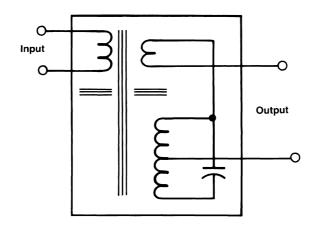
Figure 5.39 Basic design of a ferroresonant transformer. (After [2].)
