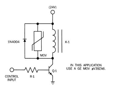
Figure 6.44 Transient suppression of a switched inductive load.
