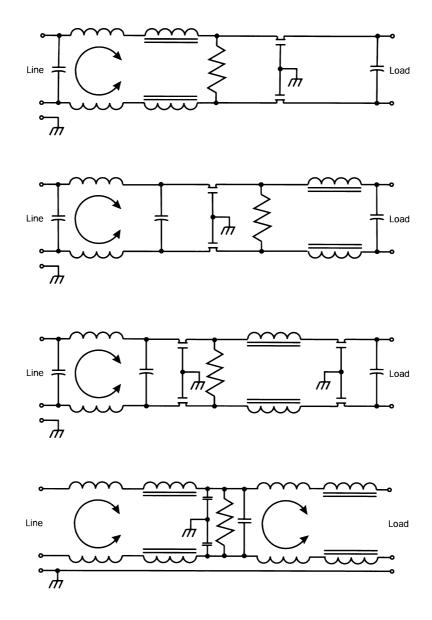
Figure 6.2 Power-line filter circuits of increasing complexity.
