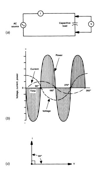
**Figure 1.43** A purely capacitive circuit: (*a*) circuit diagram; (*b*) representative waveforms; (*c*) vector representation.
