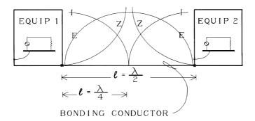
Figure 7.71 Standing waves on a bonding conductor resulting from the antenna effect. (*From* [5]. *Used with permission*.)
