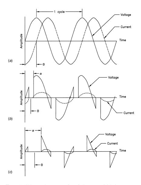
**Figure 4.17** Voltage and current waveforms for inverse-parallel thyristor power control with an inductive load: (*a*) full conduction; (*b*) small-angle phase reduction; (*c*) large-angle phase reduction.
