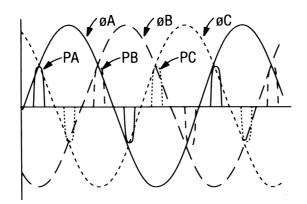
**Figure 2.31** Fundamental and pulsed currents. The sum of the pulses in the neutral equals three times the rms value of any one phase pulse because there is little or no overlap or cancellation. The rms current in the neutral depends on each single-phase pulse rms current, and the pulse shape, frequency, and duration. (*From* [5]. *Used with permission*.)
