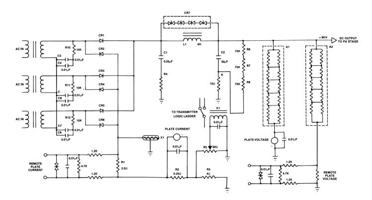
Figure 6.36 High-voltage power supply incorporating transient-suppression devices.
