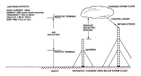
**Figure 2.1** The lightning effect and how it can be compared to a more familiar mechanism, the capacitor principle. Also shown are the parameters of a typical lightning strike.
