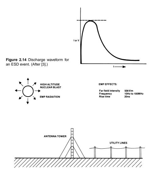
**Figure 2.15** The EMP effect and how it can induce damaging voltages onto utility company lines and antenna structures. The expected parameters of an EMP event also are shown.
