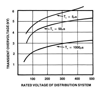
**Figure 2.21** The relationship (computed and measured) between utility company system voltage and switching transient peaks. Switching transients are plotted as a function of nominal operating voltages for three values of the transient tail time to half-potential. It can be seen that there is no direct linear increase in transient amplitude as the system voltage is increased.
