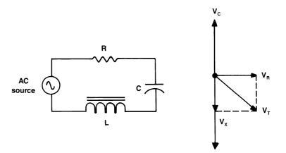
Figure 1.1 Voltage vectors in a series RLC circuit.
