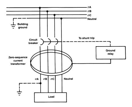
Figure 9.5 Ground-fault detection in a three-phase ac system.
