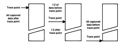
Figure 2.51 The use of a pre/post trigger function for waveform analysis.
