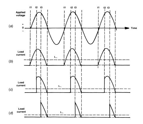
**Figure 4.20** The effect of varying the phase angle of a thyristor on the load current  $I_{avg}$ : (a) applied voltage, (b) thyristor switched on at the zero crossing, (c) thyristor switched on at approximately 60° after the zero crossing, (d) thyristor switched on at approximately 90° after the zero crossing.
