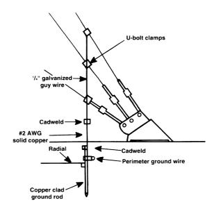
Figure 7.24 Recommended guy-anchor grounding procedure. (After [9].)
