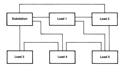
Figure 1.51 Network power-transmission system.
