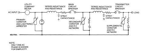
**Figure 6.28** The use of ac system series inductance and resistance to aid transient suppressors in controlling line disturbances. This technique is known as *staging*.
