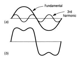
**Figure 2.28** The addition of 60 Hz fundamental and 3<sup>rd</sup> harmonic waveshapes: (a) individual waveforms, (b) resulting distorted waveshape. (*From* [5]. *Used with permission*.)
