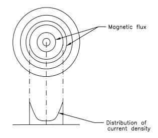
Figure 1.46 The skin effect on a conductor.
