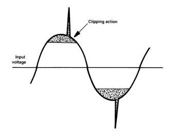
Figure 5.41 Clipping characteristics of a ferroresonant transformer.
