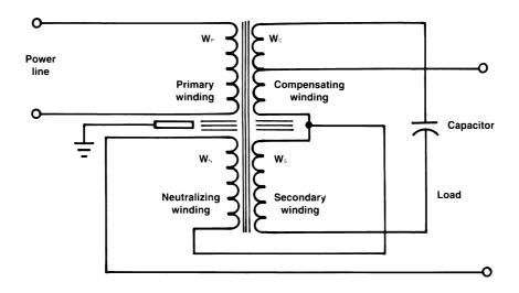
**Figure 5.40** Improved ferroresonant transformer design incorporating a compensating winding and a neutralizing winding. (Adapted from documentation provided by Dranetz Technologies.)
