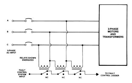
Figure 6.31 Phase-loss protection using relay logic.
