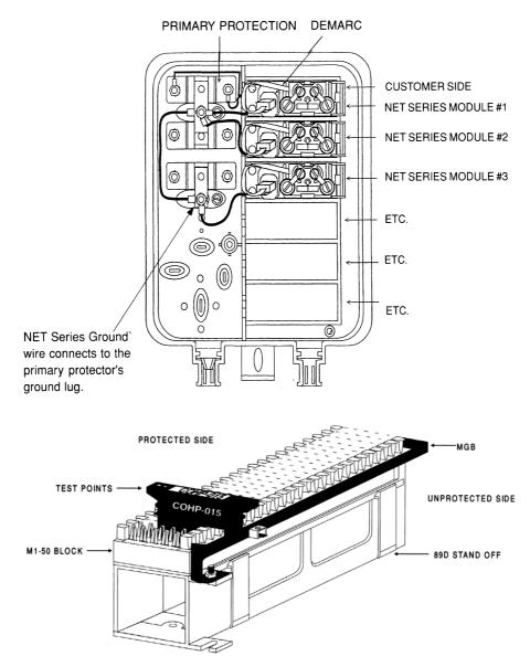
**Figure 6.43** Telco and low-voltage surge protection: (*a*) telco service entrance device, (*b*) connection block protection device. (*Courtesy of Control Concepts*.)
