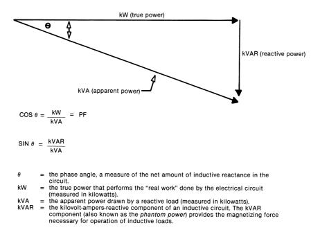
**Figure 1.59** The mathematical relationships of an inductive circuit as they apply to power factor (PF) measurements. Reducing the kVAR component of the circuit causes  $\theta$  to diminish, improving the PF. When kW is equal to kVA, the phase angle is zero and the power factor is unity (100 percent).
