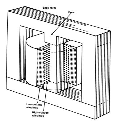
**Figure 1.9** Physical construction of an E-shaped core transformer. The low- and high-voltage windings are stacked as shown.
