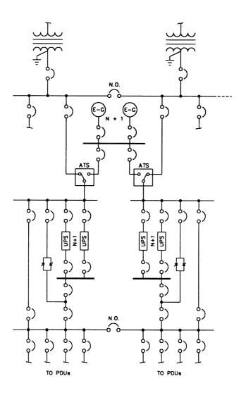
**Figure 8.11** Power distribution system featuring redundancy and high reliability. Of particular interest is the ability to parallel UPS systems as required by operational conditions. (*After* [4].)
