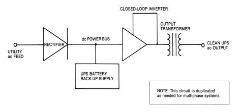
**Figure 5.23** Block diagram of an uninterruptible power system using ac rectification to float the battery supply. A closed-loop inverter draws on this supply and delivers clean ac power to the protected load.
