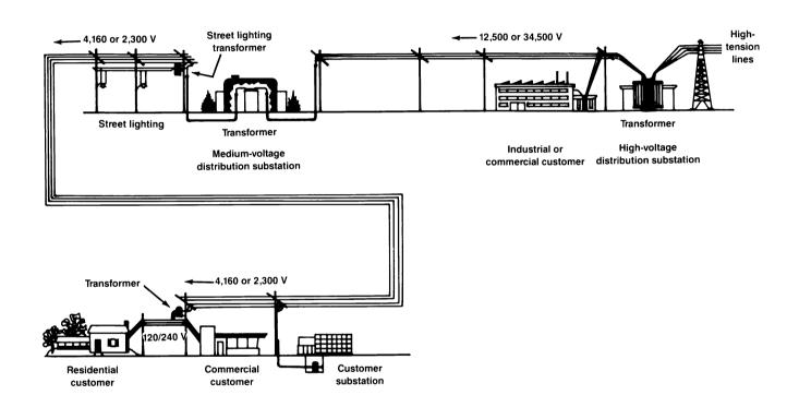
Figure 1.48 Simplified power-distribution architecture.
