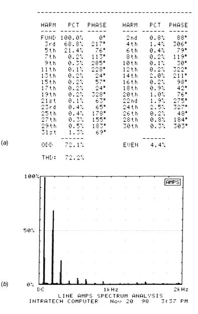
**Figure 2.54** Analysis of harmonic content at a monitored site: (*a*) recorded data, (*b*) graphical representation. (*After* [11].)
