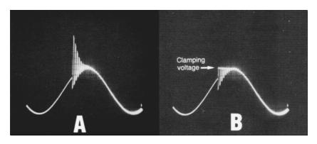
**Figure 6.7** The clamping action of an MOV: (*a*) an oscillatory transient on the ac waveform, (*b*) the same waveform clamped by an MOV on the ac circuit. (*From* [3]. *Used with permission*.)
