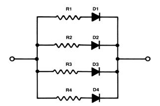
Figure 4.5 Using build-out resistances to force current sharing in a parallel rectifier assembly.
