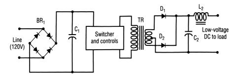
**Figure 2.32** Simplified block diagram of a switching-mode power supply. (*From* [5]. *Used with permission*.)
