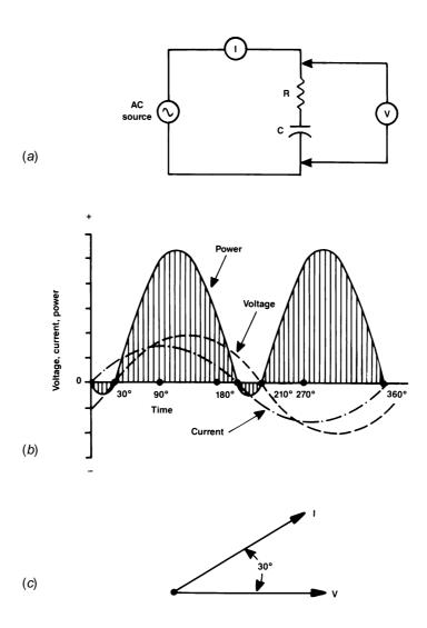
**Figure 1.44** A resistive-capacitive circuit: (*a*) circuit diagram; (*b*) representative waveforms; (*c*) vector representation.
