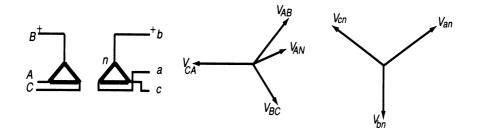
**Figure 1.23**  $\Delta$ - $\Delta$  transformer with 0° phase shift between the primary and the secondary sides. (*From* [3]. *Used with permission*.)
