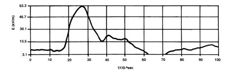
Figure 2.17 Discharge waveform for a nuclear EMP event.
