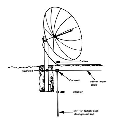
Figure 7.31 Grounding a satellite receiving antenna. (After [9].)
