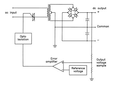
Figure 4.23 Phase-controlled power supply with primary regulation.
