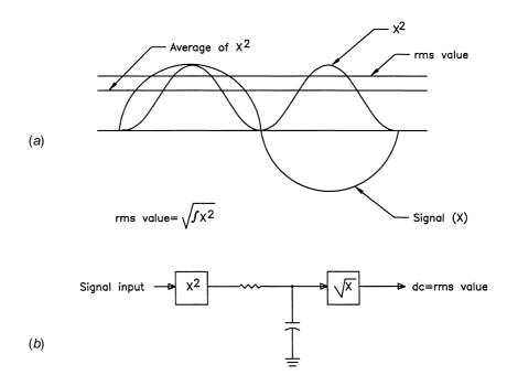
**Figure 2.41** Root-mean-square (rms) voltage measurements: (*a*) the relationship of rms and average values, (*b*) the rms measurement circuit.
