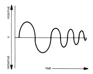
Figure 3.5 Waveshape of a typical transient disturbance. Note how the tail of the transient oscillates as it decays.
