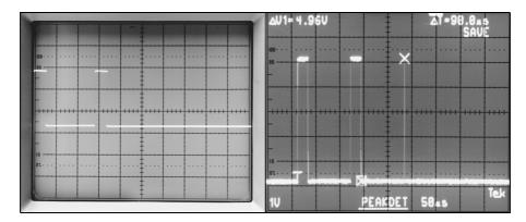
**Figure 2.52** The benefits of a DSO in capturing transient signals: (*a*, left) analog display of a pulsed signal with transient present, but not visible; (*b*, right) display of the same signal clearly showing the transient. (*Courtesy of Tektronix*.)
