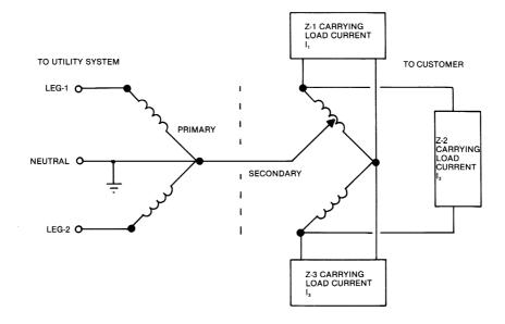
**Figure 1.73** The open-delta (or V-V) utility company service connection transformer. This configuration is not recommended because of its poor voltage regulation under varying load, high third-harmonic content, and transient disturbance propagation characteristics.
