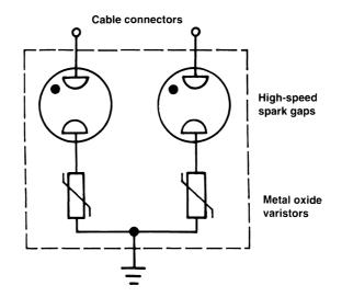
**Figure 6.30** A hybrid voltage-protection device incorporating a gas-tube spark-gap and varistor in each suppression element. The design goal is to extend the life of the varistors.
