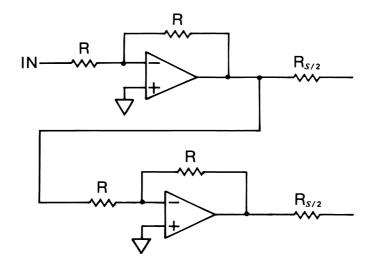
**Figure 7.78** A basic active-balanced output circuit. This configuration works well when driving a single balanced load.
