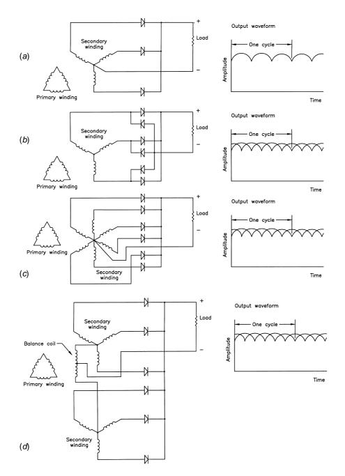
**Figure 4.10** Basic 3-phase rectifier circuits: (*a*) half-wave wye, (*b*) full-wave bridge, (*c*) 6-phase star, (*d*) 3-phase double-wye.
