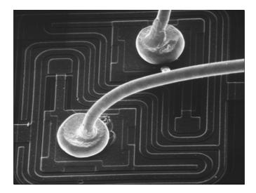
**Figure 3.20** A scanning electron microscope photo illustrating ESD damage to the metallization of a MOSFET device.
