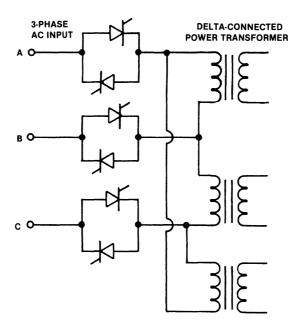
Figure 4.19 Modified full-thyristor three-phase ac control of an inductive delta load.
