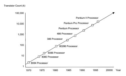
**Figure 3.24** Microcomputer transistor count per chip as a function of time. (*From* [2]. *Courtesy of Intel.*)
