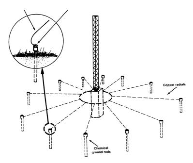
Figure 7.16 Tower grounding scheme using buried copper radials and chemical ground rods. (*After* [10].)
