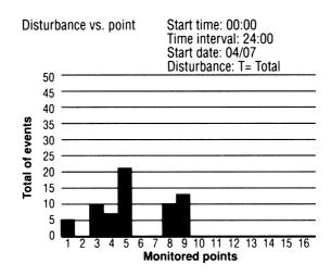
**Figure 2.55** Analysis of ac power line disturbances as a function of monitoring points over a 24-hr period. (*After* [11].)
