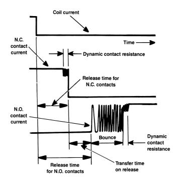
Figure 2.24 The mechanics of relay contact bounce during the de-energizing period.
