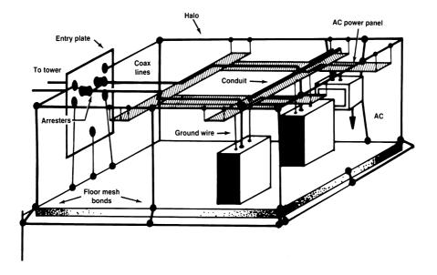
Figure 7.57 Bulkhead-based ground system including a grounding halo.
