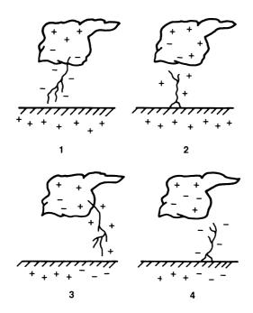
Figure 2.5 Four general types of lightning activity. (After [1].)
