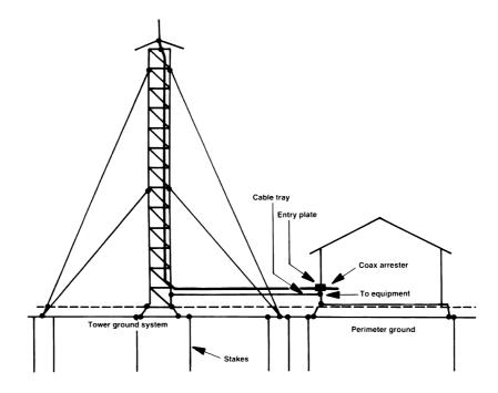
**Figure 7.45** The preferred grounding arrangement for a transmission facility using a bulkhead panel. With this configuration, all damaging transient overvoltages are stripped off the coax, power, and telephone lines before they can enter the equipment building.
