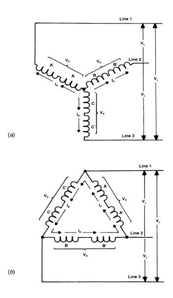
Figure 1.26 Generator circuit configurations: (a) wye; (b) delta.
