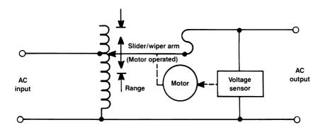
Figure 5.50 Variable ratio voltage regulator. (After [2].)
