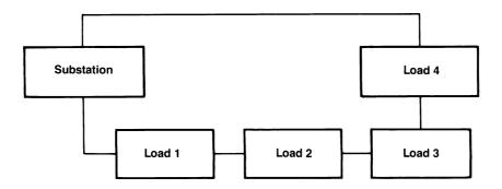
Figure 1.50 Ring power-transmission system.
