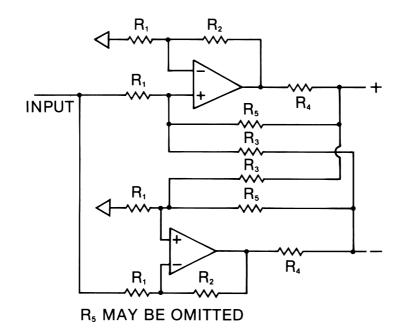
**Figure 7.79** An electronically balanced and floating output circuit. A stage such as this will perform well even when driving unbalanced loads.
