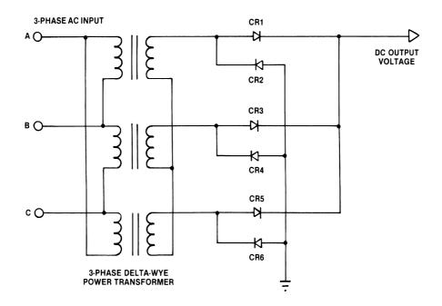
Figure 6.34 Three-phase full-wave bridge rectifier circuit.
