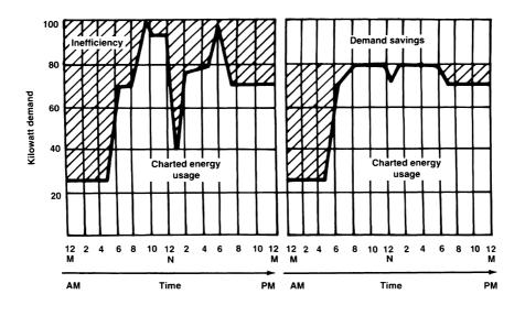
**Figure 8.18** An example of the successful application of a load-shedding program. Energy usage has been spread more evenly throughout the day, resulting in reduced demand, and consequently, a better rate from the utility company.
