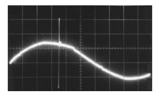
**Figure 6.21** The effect of adding a 100  $\Omega$  series resistor to the 0.25  $\mu$ F capacitor measured in Figure 6.20. Note that the resistor eliminates the oscillation, but it also reduces the transient-suppression effectiveness of the capacitor.
