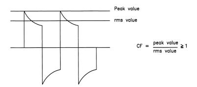
Figure 2.45 The crest factor of ac waveforms.
