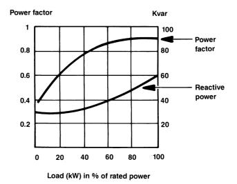
**Figure 1.63** The relationship of reactive power and power factor to percentage of load for a 100 kW, three-phase induction motor.
