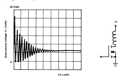
**Figure 3.8** Drain-source transient resulting from switching off an unclamped inductive load. (*Courtesy of Motorola.*)
