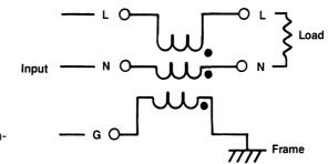
Figure 6.1 Balun commonmode filter. (*After* [1].)
