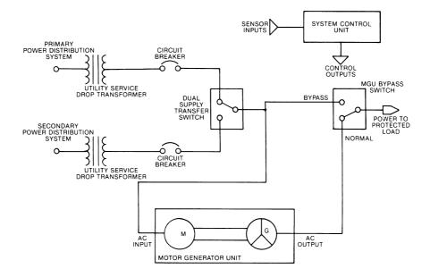
**Figure 8.6** A dual feeder standby power system using a motor-generator set to provide power fail ride-through and transient-disturbance protection. Switching circuits allow the m-g set to be bypassed, if necessary.
