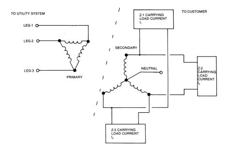
**Figure 1.72** Delta-wye transformer configuration for utility company power distribution. This common type of service connection transformer provides good isolation of the load from the high-voltage distribution-system line.
