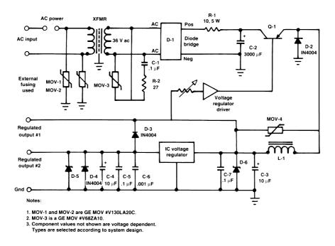
**Figure 6.33** Transient-overvoltage protection for a low-voltage power supply. A circuit such as this will survive well in the field despite frequent transient disturbances.
