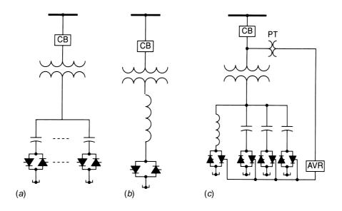
**Figure 1.71** Basic static VAR compensator configurations: (*a*) thyristor-switched shunt capacitors (TSC); (*b*) thyristor-switched shunt reactors (TSR); (*c*) combined TSC/TSR. (*From* [17]. *Used with permission*.)
