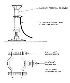
Figure 7.54 Bonding detail for the raised-floor support system.
