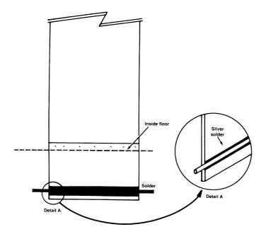
**Figure 7.42** The proper way to ground a bulkhead panel and provide a low-inductance path for surge currents stripped from cables entering and leaving the facility. The panel extends along the building exterior to below grade. It is silver-soldered to a no. 2/0 copper wire that interconnects with the outside ground system. (*After* [9].)
