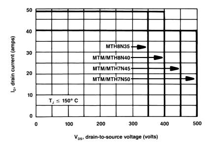
**Figure 3.7** Maximum rated switching safe operating area of the MTM8N40 MOSFET. (*Courtesy of Motorola*.)
