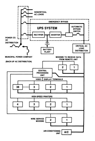
**Figure 8.12** An application of the critical-load power bus concept. In the event of a power failure, all equipment necessary for continued operation is powered by the UPS equipment. Noncritical loads are dropped until commercial ac returns.
