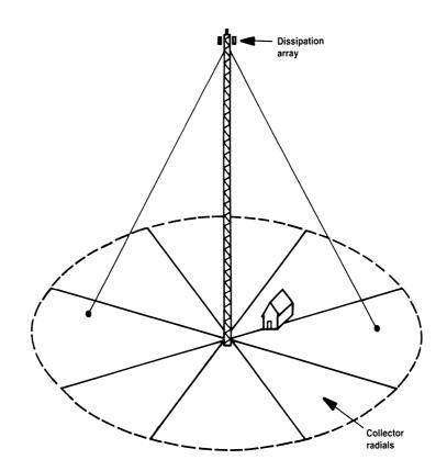
Figure 2.11 Intended protection area for a dissipation array.
