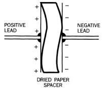
**Figure 4.37** Failure mechanism of an electrolytic capacitor exhibiting a loss of capacitance. After the electrolyte dries, the plates can no longer come in contact with the aluminum oxide. The result is a decrease in capacitor value.
