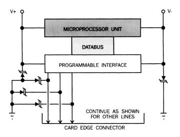
Figure 6.39 Application of transient-suppression devices to microcomputer circuits.
