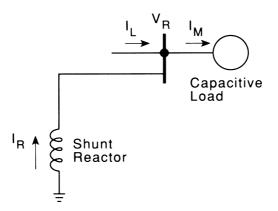
Figure 1.68 Shunt-reactor-compensated load. (From [17]. Used with permission.)
