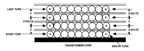
Figure 4.31 Voltage distribution between the layers of a typical layer-wound power transformer.
