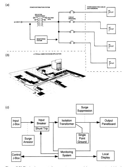
**Figure 7.58** The basic concept of a computer-room modular power center: (*a*) basic line drawing of system, (*b*) typical physical implementation, (*c*) functional block diagram. Both single- and multiphase configurations are available. When ordering an MPC, the customer can specify cable lengths and terminations, making installation quick and easy. (*After* [17].)
