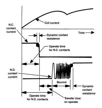
Figure 2.23 The mechanics of relay contact bounce during the energizing period.
