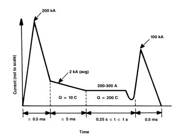
Figure 2.40 Lightning test current waveform specified in MIL STD-1757A. (After [7].)
