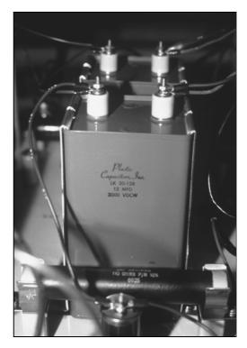
**Figure 4.33** An oil-filled, high-volt-age capacitor.
