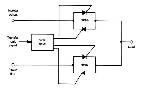
Figure 5.22 Static load-transfer switch.
