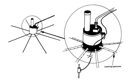
Figure 7.15 Hub and spoke counterpoise ground system. (After [10].)
