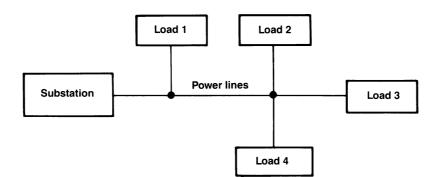
Figure 1.49 Radial power-transmission system.
