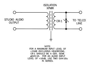
Figure 6.42 Application of a transient-suppression device to a telephone company audio or data line.
