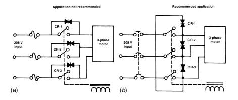
**Figure 6.46** Transient suppressor application considerations: (*a*) suppression circuit arrangement that should be avoided, (*b*) alternate configuration that provides fail-safe operation. The application of any transient-suppression component must be considered carefully, keeping in mind the various modes of operation and the possibility of protection-device failure.
