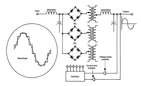
Figure 5.33 Step wave inverter and output waveform.
