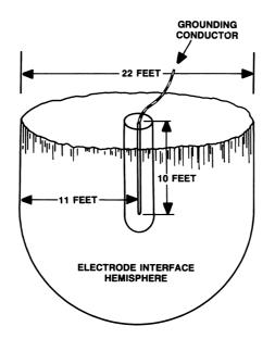
**Figure 7.5** The effective earth-interface hemisphere resulting from a single driven ground rod. The 90 percent effective area of the rod extends to a radius of approximately 1.1 times the length of the rod. (*After* [10].)
