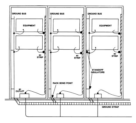
**Figure 7.60** Recommended grounding method for equipment racks. To make assembly of multiple racks easier, position the ground connections and ac receptacles at the same location in all racks.
