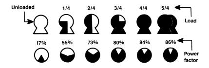
Figure 1.62 Changes in power factor for an induction motor as a function of motor loading.
