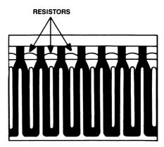
**Figure 3.3** Interdigited geometry of emitter resistors used to balance currents throughout a power device chip.
