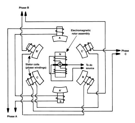
Figure 1.25 Simplified diagram of a three-phase ac generator.
