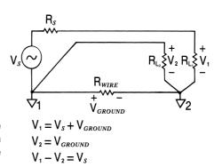
**Figure 7.66** Ground-loop noise can be canceled by amplifying both the high side and the ground side of the source and subtracting the two signals.
