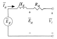
**Figure 1.30** The per-phase equivalent circuit of a round-rotor synchronous machine.  $\overline{E}_F$  is the internal voltage (phasor form) and  $V_t$  is the terminal voltage.
