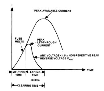
**Figure 4.41** The current let-through characteristics of a semiconductor fuse. Note that the clearing time of the device is less than 8.3 ms.
