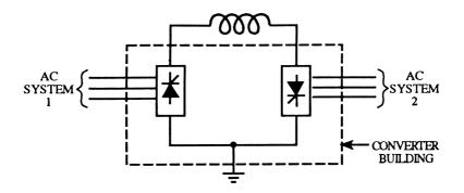
**Figure 1.53** The back-to-back system of dc transmission. (*From* [16]. *Used with per-mission*.)
