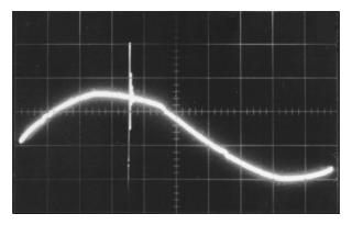
Figure 6.20 The transient-suppression performance of a 0.25  $\mu$ F capacitor. Although the spike is reduced substantially, a small amount of oscillation can be seen in the display.
