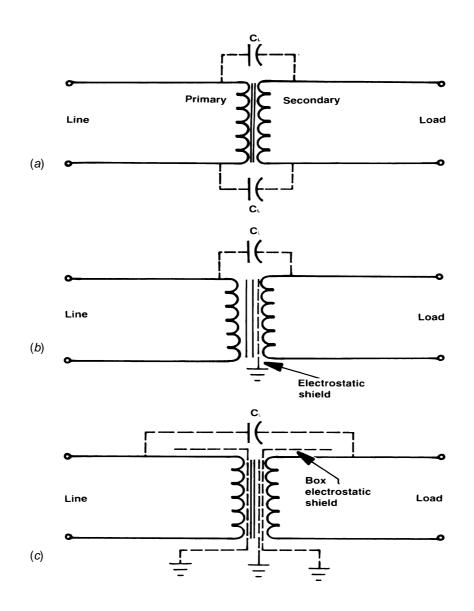
**Figure 5.45** The elements involved in a noise-suppression isolation transformer: (*a*) conventional transformer with capacitive coupling as shown; (*b*) the addition of an electrostatic shield between the primary and the secondary; (*c*) transformer with electrostatic box shields surrounding the primary and secondary windings.
