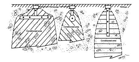
**Figure 7.13** An alternative approach to the chemically activated ground rod. Multiple holes are provided on the ground-rod assembly to increase the effective earth-to-electrode interface. Note that chemical rods can be produced in a variety of configurations. (*After* [10].)
