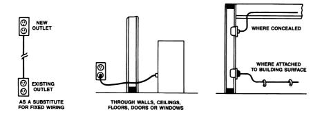
Figure 9.9 Flexible cord uses prohibited under NEC rules.
