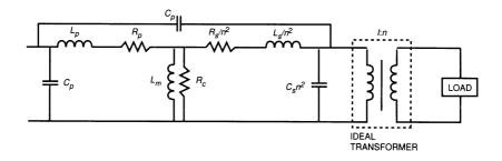
Figure 1.16 Transformer equivalent circuit. (From [4]. Used with permission.)
