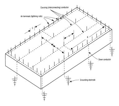
**Figure 7.47** Conduction lightning-protection system for a large building. (*From* [12]. *Used with permission.*)
