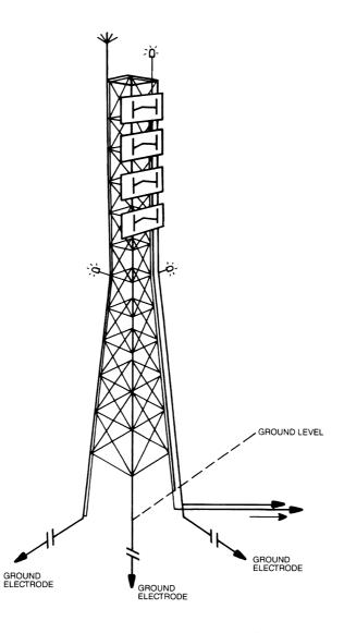
Figure 7.27 Interconnecting a self-supporting tower to the buried ground system.
