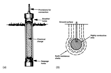
**Figure 7.12** An air-breathing chemically activated ground rod: (*a*) breather holes at the top of the device permit moisture penetration into the chemical charge section of the rod; (*b*) a salt solution seeps out of the bottom of the unit to form a conductive shell. (*After* [10].)
