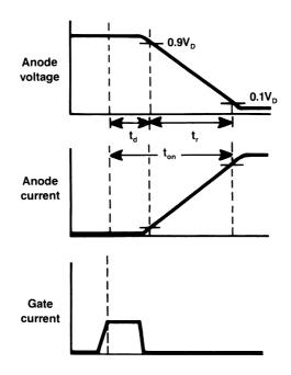
**Figure 3.14** Turn-on waveforms for an SCR device.  $T_d$  = delay time interval between a specified point at the beginning of a gate pulse and the instant at which the principal voltage drops to a specified value.  $T_r$  = rise time between the principal voltage dropping from one value to a second lower value when the thyristor turns from off to on.
