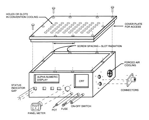
**Figure 2.34** Principal aperture leakage points in an electronics enclosure. (*From* [6]. *Used with permission.*)
