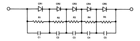
Figure 4.2 A portion of a high-voltage, series-connected rectifier stack.
