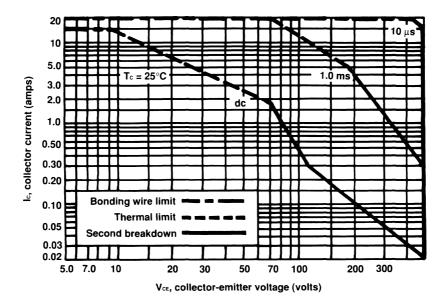
**Figure 3.1** Forward bias safe operating area curve for a bipolar transistor (MJH16010A). (*Courtesy of Motorola.*)
