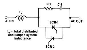
**Figure 3.15** The basic *RC* snubber network commonly used to protect thyristors from fast-rise-time transients.
