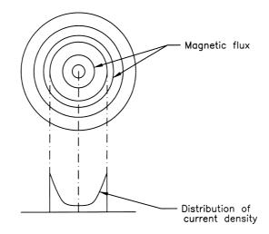
Figure 7.23 Skin effect on an isolated round conductor carrying a moderately high-frequency signal.
