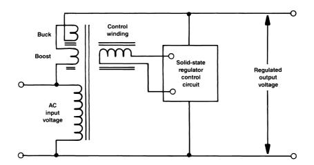
Figure 5.42 Block diagram of an electronic magnetic regulator. (After [2].)
