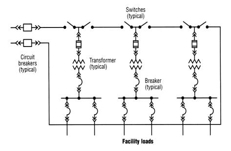
**Figure 8.16** A redundant, fault-tolerant secondary plant distribution system. (*From* [5]. *Used with permission.*)
