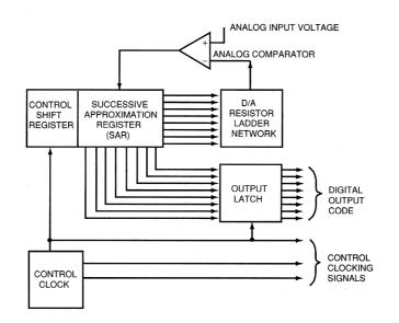
Figure 2.49 Successive approximation A/D converter block diagram. (After [9].)
