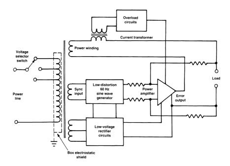
Figure 5.53 Power-line conditioner using linear amplifier correction.
