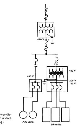
**Figure 7.59** Preferred power-distribution configuration for a data processing site. (*After* [15].)
