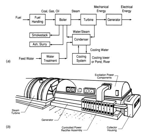
**Figure 1.33** Primary components of a fossil fuel power plant: (*a*) system block diagram; (*b*) common configuration of turbine/generator system. (*Drawing* a *from* [7]. *Used with permission. Drawing* b *from* [14]. *Used with permission.*)
