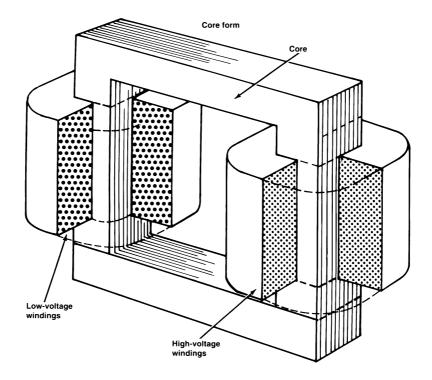
**Figure 1.10** Transformer construction using a box core with physical separation between the low- and high-voltage windings.
