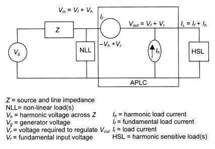
Figure 5.57 Basic conceptual diagram of the active power line conditioner. (After [7].)
