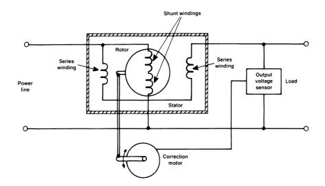
Figure 5.52 Rotary induction voltage regulator.
