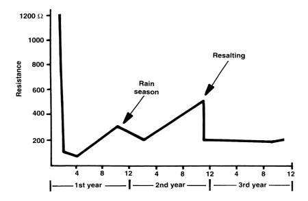
**Figure 7.11** The effect of soil salting on ground-rod resistance with time. The expected resalting period, shown here as 2 years, varies depending on the local soil conditions and the amount of moisture present. (*After* [10].)
