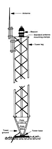
**Figure 7.25** Ground-conductor dressing for the base of a guyed tower. (*After* [9].)
