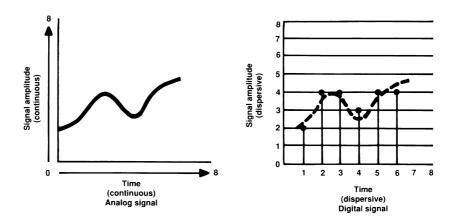
Figure 2.47 Illustration of the quantization process.
