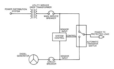
**Figure 8.1** The classic standby power system using an engine-generator set. This system protects a facility from prolonged utility company power failures.
