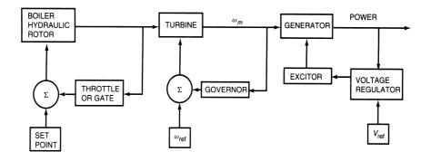
Figure 1.32 Block diagram of a generating control system. (*From* [5]. *Used with per-mission*.)
