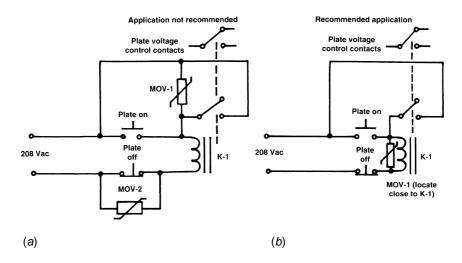
**Figure 6.47** Transient suppressor application considerations: (*a*) suppression circuit arrangement that should be avoided, (*b*) alternate configuration that provides fail-safe operation.
