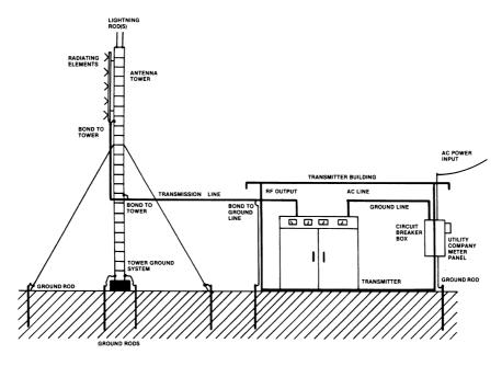
**Figure 7.43** A common, but not ideal, grounding arrangement for a transmission facility using a grounded tower. A better configuration involves the use of a bulkhead panel through which all cables pass into and out of the equipment building.
