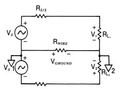
**Figure 7.67** A balanced source configuration where the inherent amplitude error of the system shown in Figure 7.66 is eliminated.
