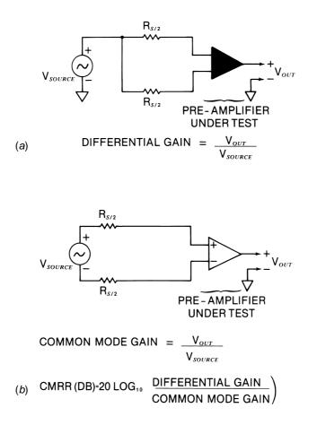
**Figure 7.74** The concept of common-mode rejection ratio (CMRR) for an active-balanced input circuit: (*a*) differential gain measurement; (*b*) calculating CMRR.
