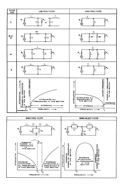
Figure 6.3 Common filter circuits, classified by function. (*From* [2]. *Used with permission*.)
