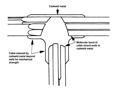
Figure 7.19 The exothermic bonding process. (After [9].)
