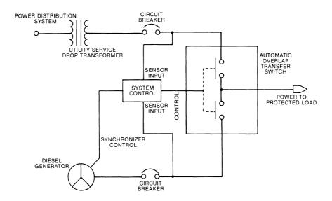
**Figure 8.5** The use of a diesel generator for standby power and peak power shaving applications. The automatic overlap (static) transfer switch changes the load from the utility feed to the generator instantly so that no disruption of normal operation is encountered.
