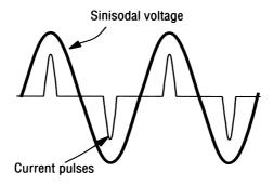
Figure 2.27 Typical waveforms of nonlinear load current. (From [5]. Used with permission.)
