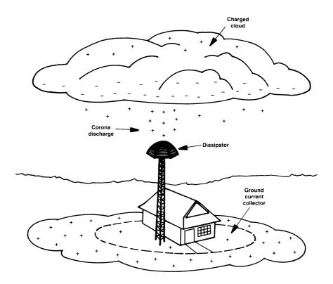
Figure 2.9 Umbrella-type dissipation array.
