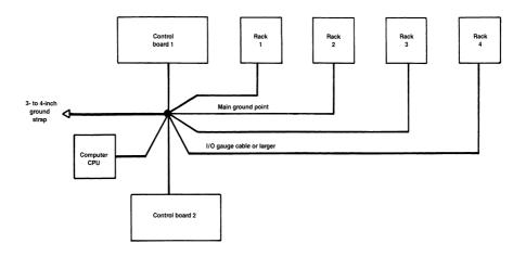
**Figure 7.48** Typical facility grounding system. The *main facility ground point* is the reference from which all grounding is done at the plant. If a bulkhead entrance panel is used, it will function as the main ground point.
