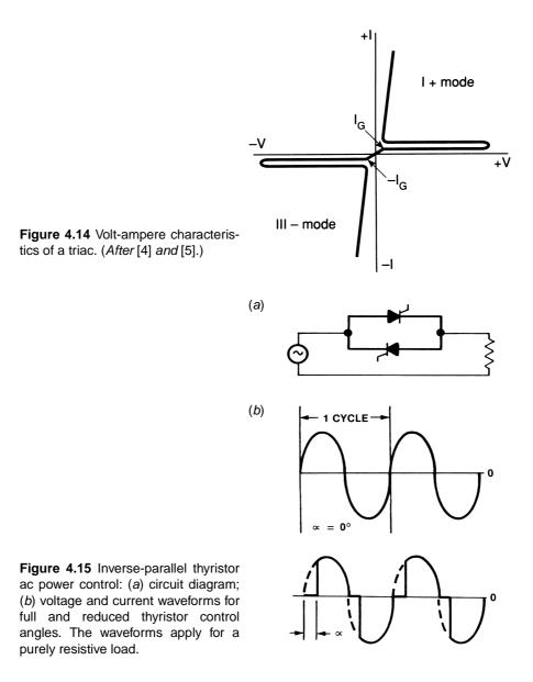
The circuit shown in Figure 4.15 requires a source of gate trigger pulses that must be isolated from each other by at least the peak value of the applied ac voltage. The two gate pulse trains must also be phased 180° with respect to each other. Furthermore, the gate pulse trains must shift together with respect to the ac supply voltage phase when power throughput is adjusted.
