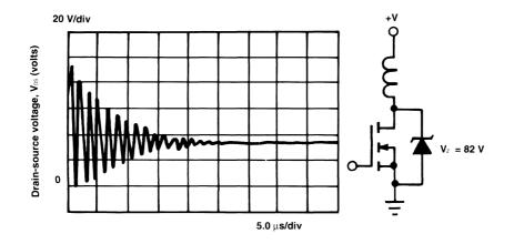
Figure 3.10 Drain-source transient with a clamping zener diode. (*Courtesy of Motor-ola.*)
