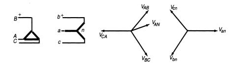
**Figure 1.22**  $\Delta$ -Y transformer with the primary side leading the secondary side by 30°. (*From* [3]. *Used with permission*.)
