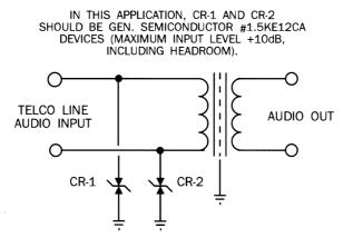
Figure 6.41 Application of transient-suppression devices to an audio distribution circuit.
