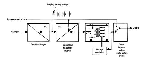
Figure 5.28 Static UPS system using saturable reactor voltage control. (After [2].)
