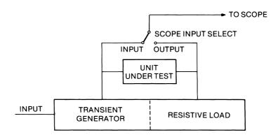
Figure 6.17 Test setup for measuring the performance of discrete transient-suppression devices.
