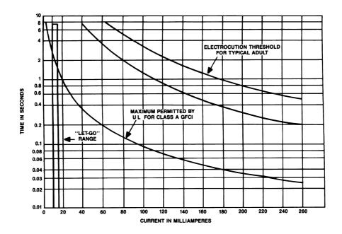
Figure 9.3 Effects of electric current and time on the human body. Note the "let-go" range.
