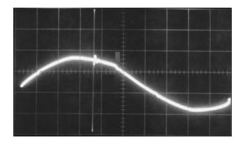
**Figure 6.16** A transient waveform used to check the performance of ac power isolation and transient-suppression components. The spike is 800 V P-P and is positioned just past the  $90^{\circ}$  point on the ac wave. The oscilloscope photo scale = 135 V/div.
