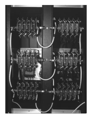
Figure 4.4 High-voltage rectifier assembly for a three-phase, delta-connected circuit.
