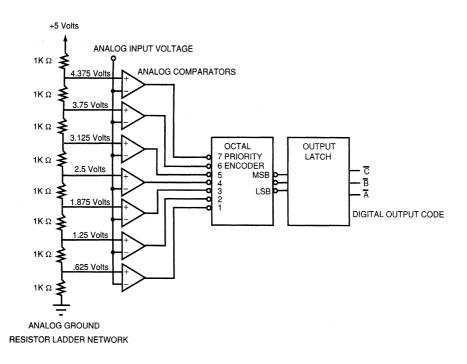
Figure 2.50 Block diagram of a flash A/D converter. (After [10].)
