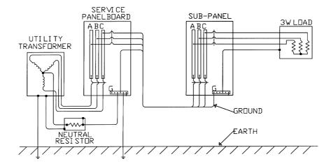
Figure 7.4 High-resistance grounded wye power system. (From [5]. Used with permission.)
