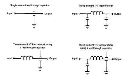
**Figure 2.33** Common radio frequency interference (RFI) networks. These filters, combined with tight mechanical assembly construction and printed wiring board ground plane shielding, will reduce significantly the possibility of noise-caused equipment disturbances.
