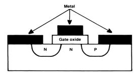
Figure 3.17 Construction of a metal gate NMOS transistor. (After [1].)
