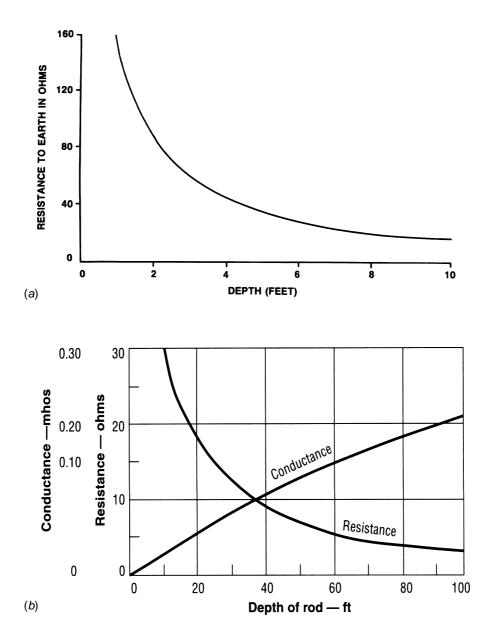
**Figure 7.7** Charted grounding resistance as a function of ground-rod length: (*a*) data demonstrating that ground-rod length in excess of 10 ft produces diminishing returns (1-in.-diameter rod) [10], (*b*) data demonstrating that ground system performance continues to improve as depth increases. (*Chart* b from [12]. Used with permission.)
