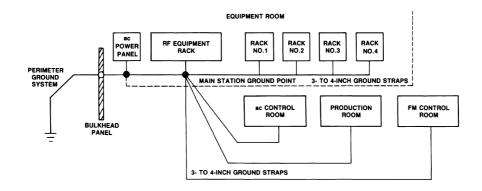
**Figure 7.55** Typical grounding arrangement for individual equipment rooms at a communications facility. The ground strap from the main ground point establishes a *local ground point* in each room, to which all electronic equipment is bonded.
