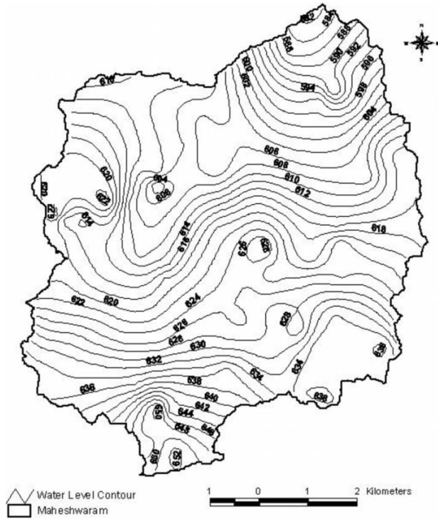
Figure 1. Piezometric map and pumping wells distribution in Maheshwaram watershed. Maheshwaram village (30 km south from Hyderabad) is at the centre of the map.
