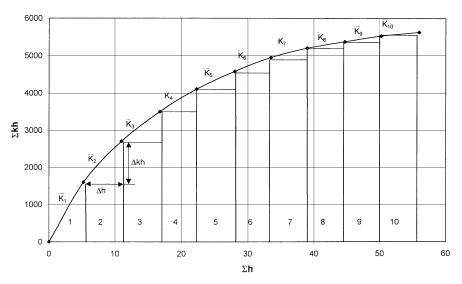
Figure 4-35. Cumulative kh vs. cumulative h (Example 4-21).
