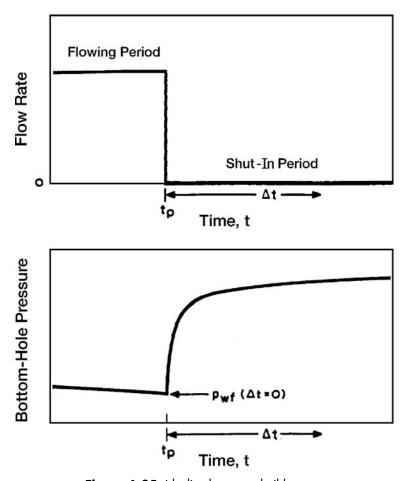
Figure 6-35. Idealized pressure buildup test.
