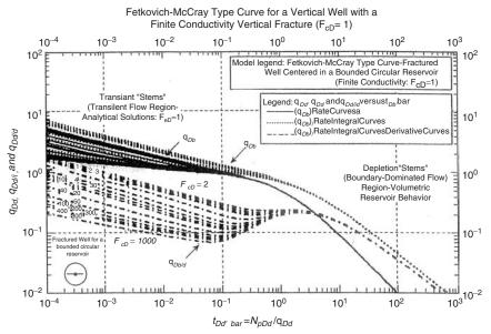
**Figure 16-29.** Fetkovich-McCray decline type curve—rate versus material balance time format for a well with a finite conductivity vertical fracture ( $F_{cD}=1$ ) (*Permission to copy by the SPE, 2003*).
