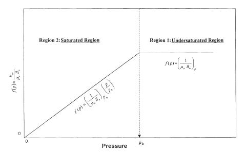
Figure 7-10. Pressure function concept.
