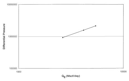
Figure 8-9. Back-pressure curve.
