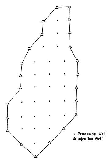
Figure 14-8. Typical peripheral waterflood. (After Cole, F., 1969.)
