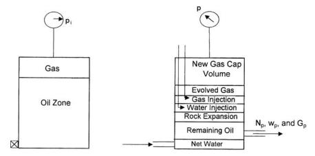
Figure 11-14. Tank-model concept.
