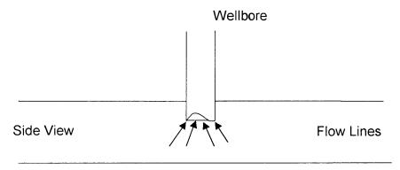
**Figure 6-8.** Hemispherical flow in a partially penetrating well.
