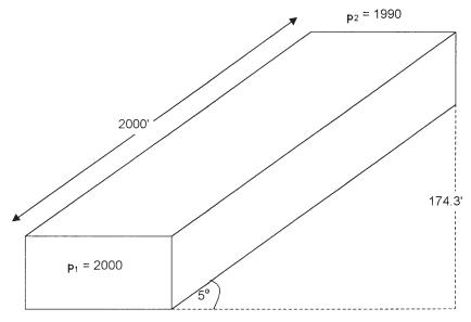
Figure 6-12. Example of a tilted layer.
