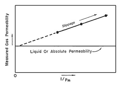
**Figure 4-21.** The Klinkenberg effect in gas permeability measurements.
