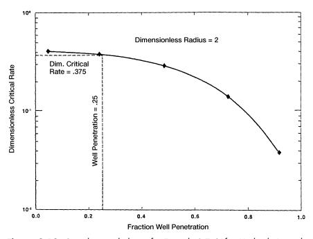
**Figure 9-18.** Critical rate calculation for Example 9-7. (After Hoyland, A. et al., courtesy SPE Reservoir Engineering, November 1989.)
