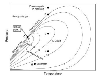
Figure 1-11. A typical phase diagram of a retrograde system.
