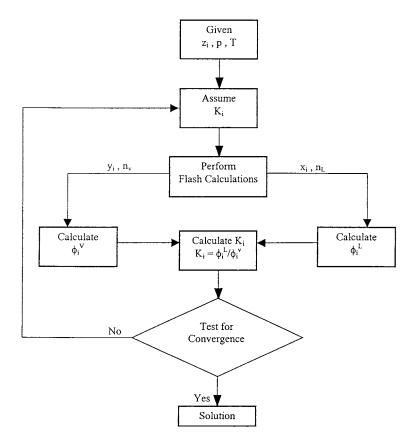
**Figure 15-14.** Flow diagram of the equilibrium ratio determination by an equation of state.
