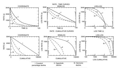
Figure 16-1. Classification of production decline curves. (After Arps, J.J. "Estimation of Primary Oil Reserves," Courtesy of Trans, AIME, vol. 207,1956).
