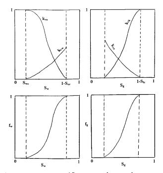
Figure 14-12. Fractional flow curves a function of saturations.
