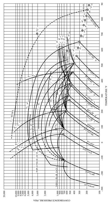
**Figure 15-3.** Convergence pressures for binary systems. (Courtesy of the Gas Processors Suppliers Association, Engineering Data Book, 10th Ed., 1987.)
