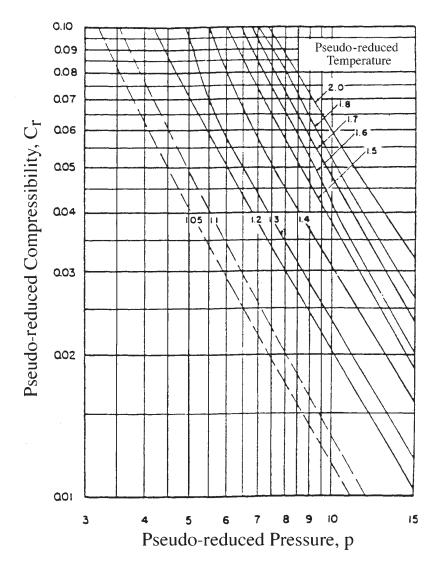
**Figure 2-4.** Trube's pseudo-reduced compressibility for natural gases. (*Permission to publish by the Society of Petroleum Engineers of AIME. Copyright SPE-AIME.*)
