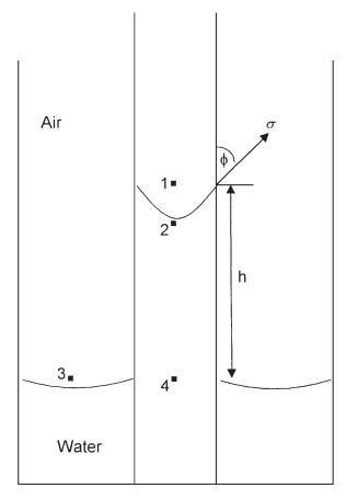
Figure 4-3. Pressure relations in capillary tubes.
