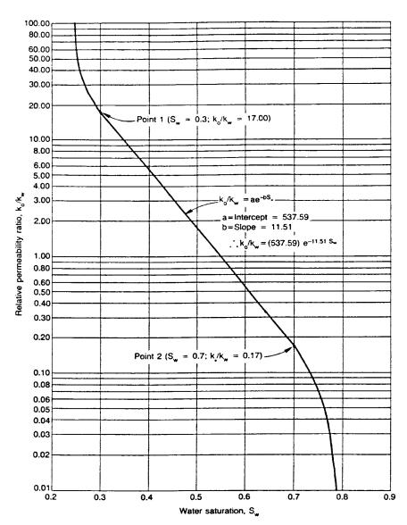
Figure 14-22. Relative permeability ratio.
