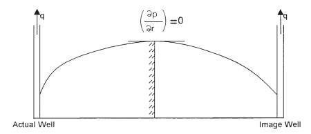
Figure 6-30. Method of images in solving boundary problems.
