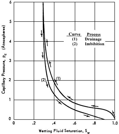
Figure 4-7. Capillary pressure hysteresis.
