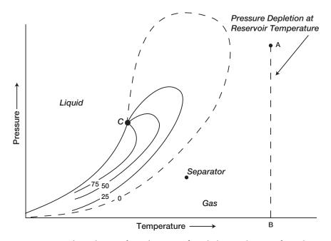
**Figure 1-16.** Phase diagram for a dry gas. (*After Clark, N.J.* Elements of Petroleum Reservoirs, *SPE, 1969.*)
