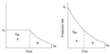
Figure 16-10. Estimation of the effect of restricting maximum production rate.
