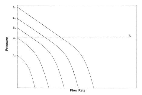
**Figure 7-7.** Effect of reservoir pressure on IPR.
