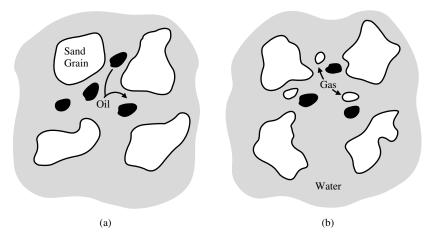
Figure 14-4. Effect of free gas saturation on S<sub>or</sub> (second theory). (After Cole, F., 1969.)
