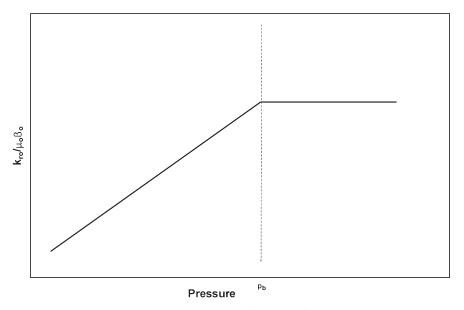
**Figure 7-6.**  $k_{ro}/\mu_o B_o$  as a function of pressure.
