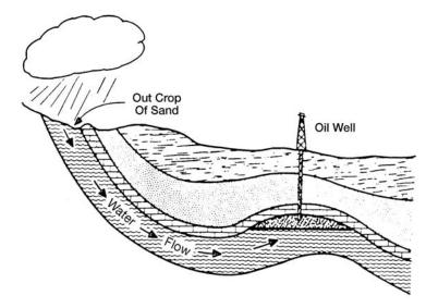
**Figure 11-7.** Reservoir having artesian water drive. (*After Clark, N. J., Elements of Petroleum Reservoirs, SPE, 1969.*)
