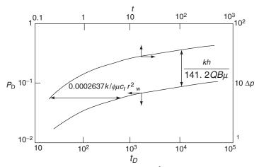
Figure 16-11. Concept of type curves.
