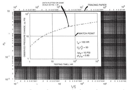
**Figure 16-13.** Illustration of type curve matching for an interference test using the type curve (After Earlougher, R. Advances in Well Test Analysis) (*Permission to publish by the SPE, copyright SPE, 1977*).
