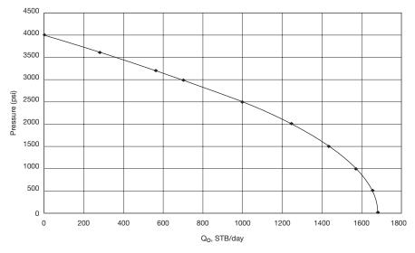
Figure 7-16. IPR using the Fetkovich method.
