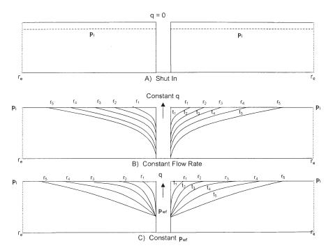
**Figure 6-17.** Pressure disturbance as a function of time.
