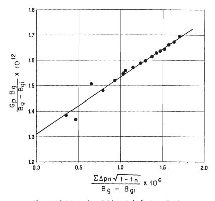
Figure 13-11. Havlena-Odeh MBE plot for Example 13-4.
