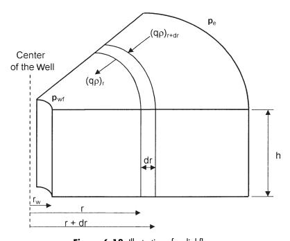
Figure 6-18. Illustration of radial flow.
