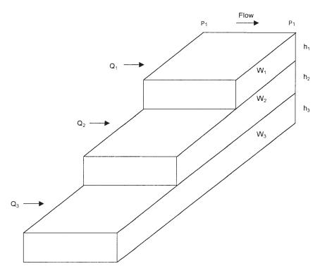
Figure 4-26. Linear flow through layered beds with variable area.
