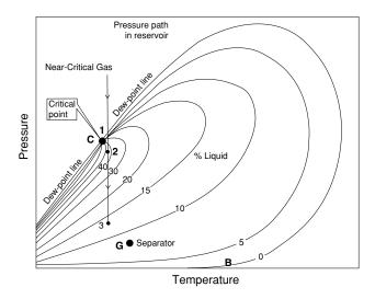
**Figure 1-13.** A typical phase diagram for a near-critical gas condensate reservoir.
