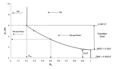
Figure 4-11. Capillary pressure saturation data.
