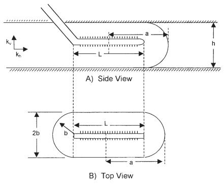
Figure 7-17. Horizontal well drainage area.
