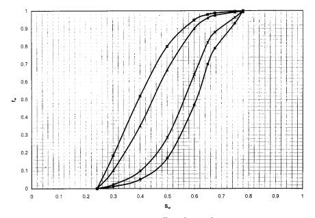
Figure 14-16. Effect of  $\mu_{\text{o}}$  on  $f_{\text{w}}.$
