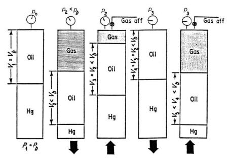
Figure 3-4. Differential vaporization test.
