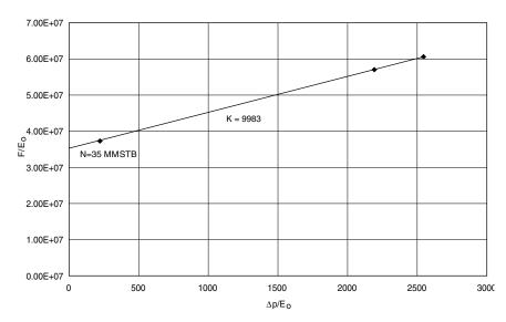
Figure 11-27.  $F/E_o$  versus  $\Delta p/E_o$ .
