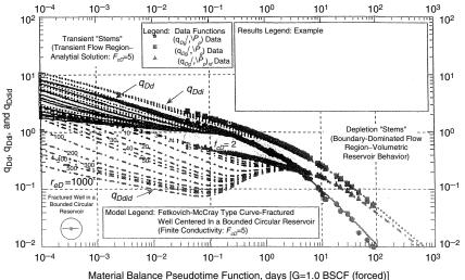
**Figure 16-33.** Match of production data for Example 1 on the Fetkovich-McCray decline type curve (pseudopressure drop normalized rate versus material balance time format) for a well with a finite conductivity vertical fracture (Fc<sub>D</sub>=5) (*Permission to copy the SPE, 2003*).
