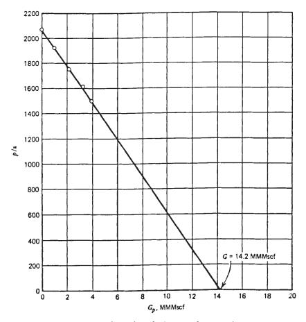
**Figure 13-3.** Relationship of p/z vs.  $G_p$  for Example 13-2.
