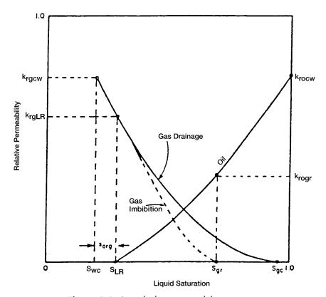
Figure 5-5. Gas-oil relative permeability curves.
