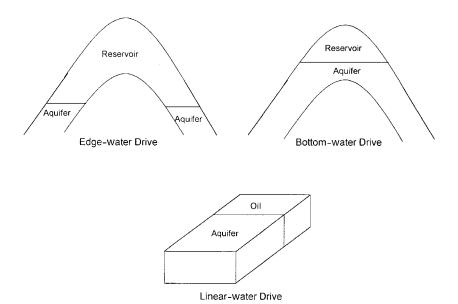
**Figure 10-1.** Flow geometries.
