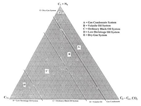
Figure 1-17. Compositions of various reservoir fluid types.
