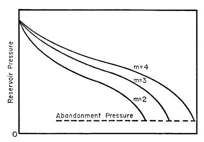
**Figure 11-5.** Effect of gas cap size on ultimate oil recovery. (After Cole, F., Reservoir Engineering Manual, Gulf Publishing Company, 1969.)
