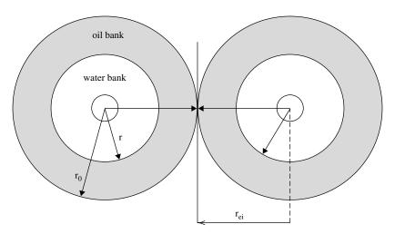
Figure 14-46. Interference of oil banks.
