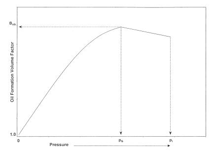
Figure 2-8. Oil formation volume factor versus pressure.
