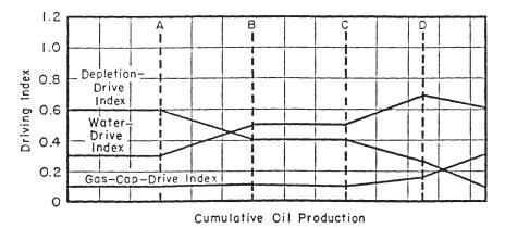
**Figure 11-15.** Driving indexes in a combination-drive reservoir. (After Clark, N. J., Elements of Petroleum Reservoirs, SPE, 1969.)
