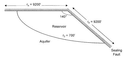
Figure 10-17. Aquifer-reservoir geometry for Example 10-10.
