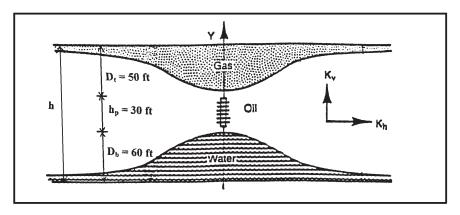
Figure 9-6. Gas and water coning problem (Example 9-3).
