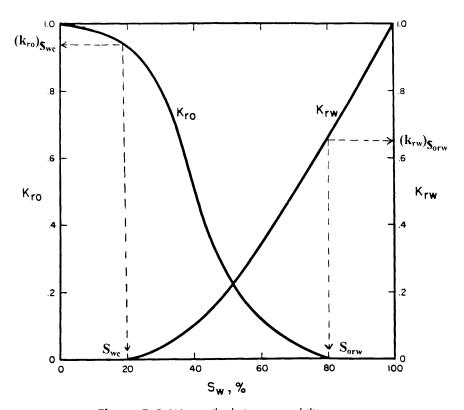
Figure 5-4. Water-oil relative permeability curves.
