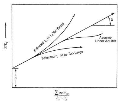
Figure 13-9. Havlena-Odeh MBE plot for a gas reservoir.
