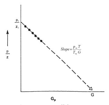
Figure 13-2. Gas material balance equation.
