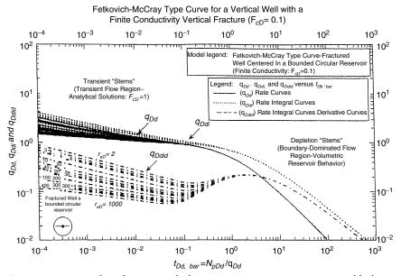
**Figure 16-28.** Fetkovich-McCray decline type curve—rate versus material balance time format for a well with a finite conductivity vertical fracture (F<sub>cD</sub>=0.1) (*Permission to copy by the SPE, 2003*).
