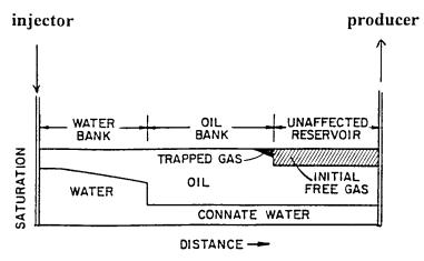
Figure 14-2. Water saturation profile during a waterflood.
