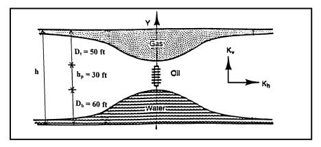
Figure 9-15. Gas and water coning problem (Example 9-5).
