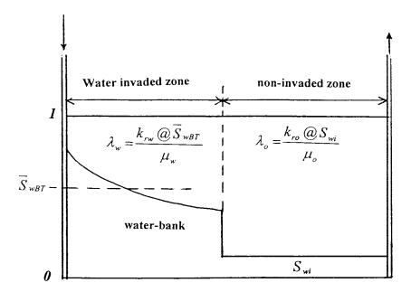
Figure 14-32. Oil and water mobilities to breakthrough.
