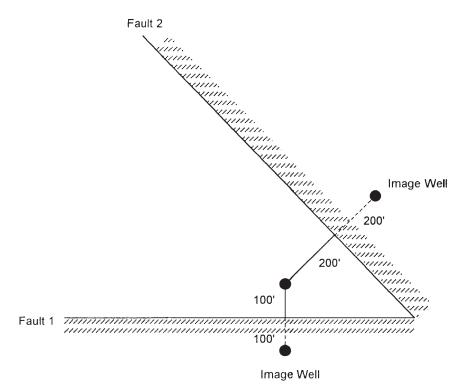
Figure 6-31. Well layout for Example 6-31.
