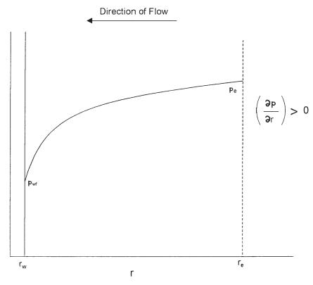
Figure 6-10. Pressure gradient in radial flow.
