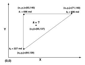
Figure 4-37. Triangulation Method
