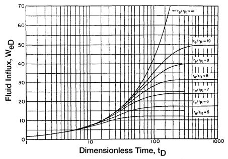
**Figure 10-9.** Dimensionless water influx  $W_{eD}$  for several values of  $r_e/r_R$ , i.e.  $r_o/r_e$ . (Van Everdingen and Hurst  $W_{eD}$ . Permission to publish by the SPE.)
