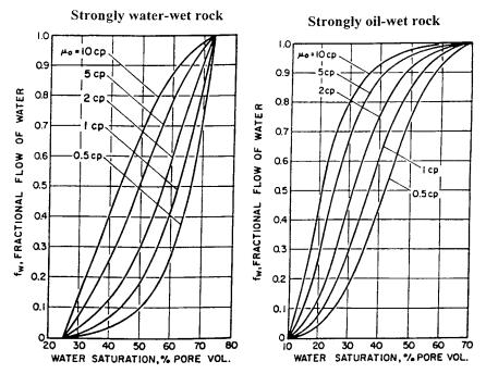
Figure 14-13. Effect of oil viscosity on f<sub>w</sub>.
