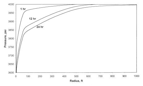
Figure 6-20. Pressure profiles as a function of time.
