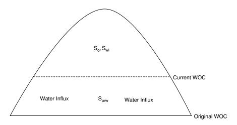
Figure 12-4. Oil saturation adjusted for water influx.
