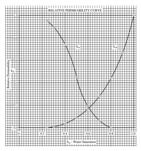
Figure 14-15. Relative permeability curves for Example 14-5.
