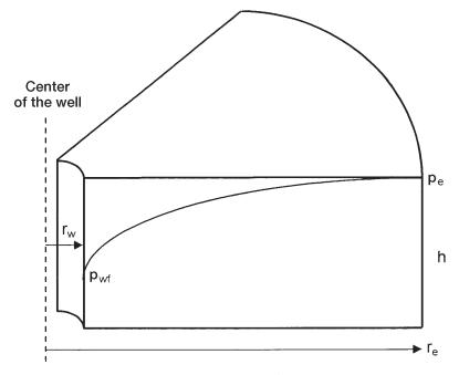
Figure 4-24. Radial flow model.
