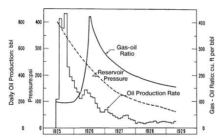
**Figure 11-2.** Production data of a solution-gas-drive reservoir. (*After Clark, N. J.,* Elements of Petroleum Reservoirs, *SPE, 1969.*)
