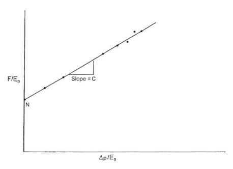
Figure 11-24. Graphical determination of N and C.
