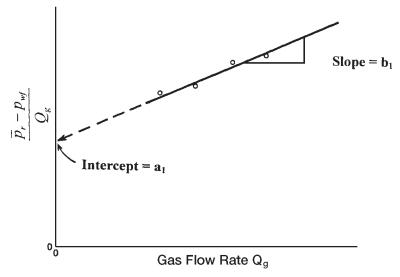
**Figure 8-5.** Graph of the pressure-method data.
