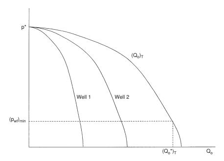
**Figure 12-10.** Overall field IPR at current pressure.
