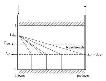
**Figure 14-27.** Average water saturation before breakthrough.
