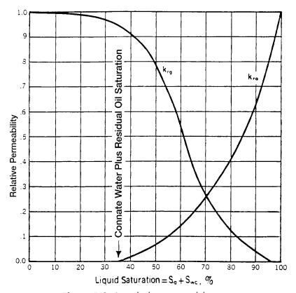
Figure 5-2. Gas-oil relative permeability curves.
