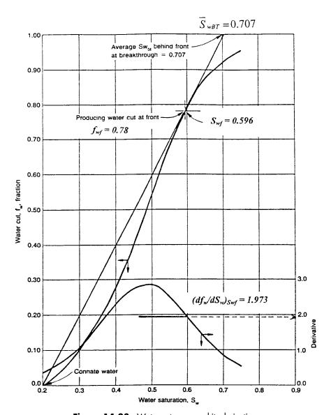
Figure 14-23. Water cut curve and its derivative.
