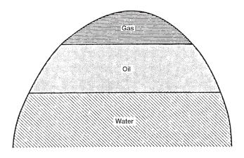
**Figure 11-11.** Initial fluids distribution in an oil reservoir.
