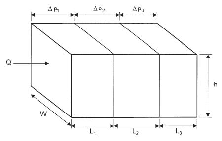
Figure 4-27. Linear flow through series beds.
