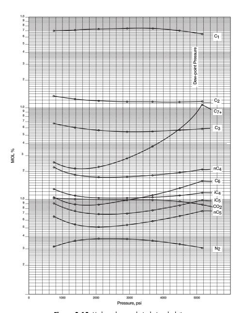
Figure 3-13. Hydrocarbon analysis during depletion.
