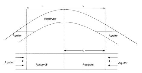
Figure 10-7. Idealized radial flow model.
