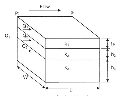
Figure 4-25. Linear flow through layered beds.
