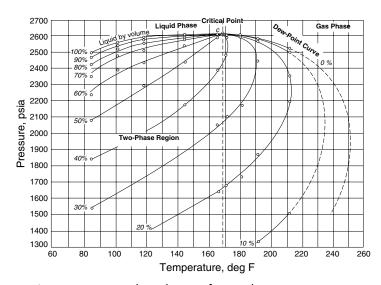
**Figure 1-1.** Typical p-T diagram for a multicomponent system.
