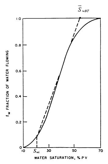
Figure 14-26. Tangent from  $S_{wi}$ .
