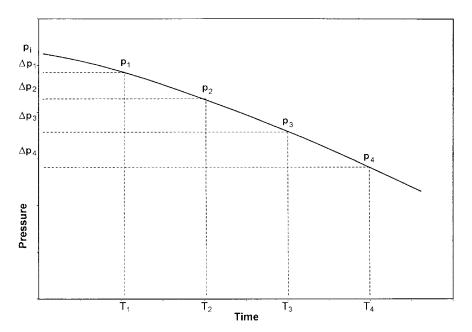
Figure 10-13. Boundary pressure versus time.
