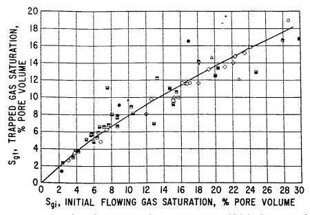
**Figure 14-5.** Relation between  $S_{gi}$  and  $S_{gt}$ . (Permission to publish by the Society of Petroleum Engineers.)
