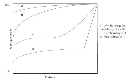
Figure 1-10. Liquid shrinkage for crude oil systems.
