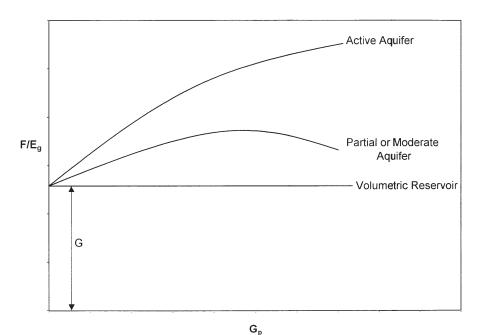
Figure 13-8. Defining the reservoir-driving mechanism.
