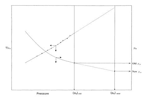
**Figure 3-10.** Extrapolating  $\mu_o$  to new  $p_b$ .
