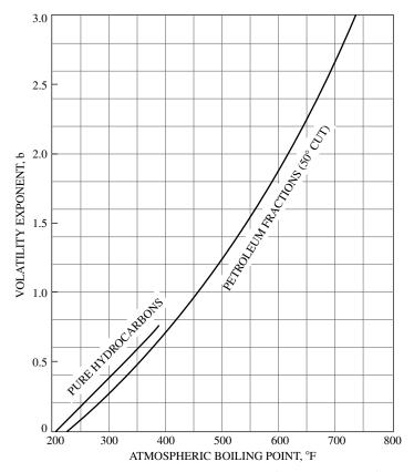
Figure 15-5. Volatility exponent. (Courtesy of the Petroleum Refiner.)
