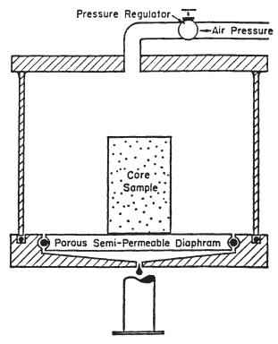
Figure 4-4. Capillary pressure equipment. (After Cole, F., 1969.)
