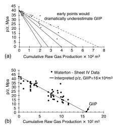
**Figure 13-15.** (a) Real-life example of pIZ plot from Sheet IVc in the Waterton Gas Field (b) Real-life example of pIZ plot from Sheet IV in the Waterton Gas Field.
