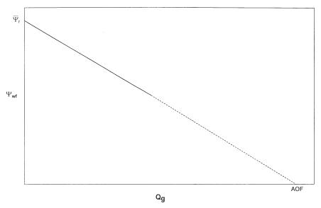
Figure 8-1. Steady-state gas well flow.
