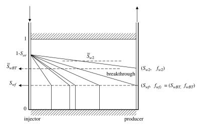
Figure 14-28. Average water saturation after breakthrough.
