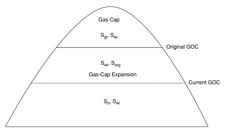
Figure 12-5. Oil saturation adjustment for gas-cap expansion.
