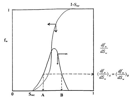
Figure 14-18. The f<sub>w</sub> curve with its saturation derivative curve.
