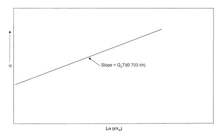
Figure 6-15. Graph of  $\Psi$  vs. ln (r/r<sub>w</sub>).
