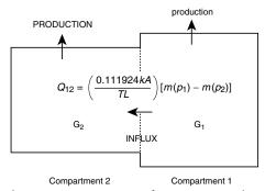
**Figure 13-16.** Schematic representation of compartmented reservoir consisting of two reservoir compartments separated by a permeable boundary.
