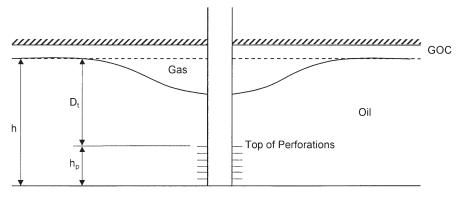
Figure 9-3. Gas coning.
