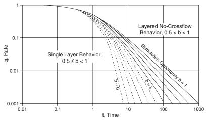
**Figure 16-18.** Depletion decline curves (After Fetkovich, 1997, copyright SPE 1997).
