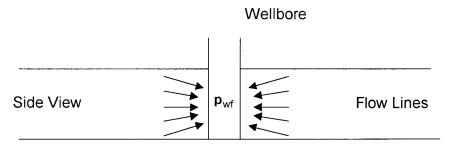
**Figure 6-7.** Spherical flow due to limited entry.
