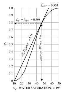
**Figure 14-37.** The  $f_{\rm w}$  curve for Example 14-11. (Permission to publish by the Society of Petroleum Engineers.)
