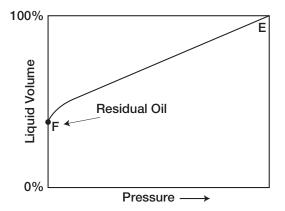
Figure 1-3. Liquid-shrinkage curve for black oil.
