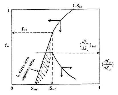
**Figure 14-19.** Effect of the capillary term on the f<sub>w</sub> curve.
