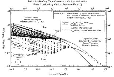
**Figure 16-30.** Fetkovich-McCray decline type curve—rate versus material balance time format for a well with a finite conductivity vertical fracture (Fc<sub>D</sub>=10) (*Permission to copy by the SPE, 2003*).
