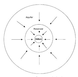
Figure 10-6. Water influx into a cylindrical reservoir.
