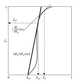
Figure 14-21. Fractional flow curve.
