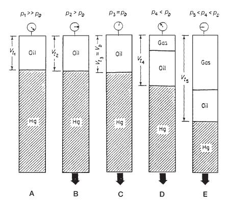
Figure 3-1. Constant-composition expansion test.
