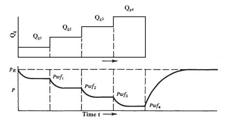
Figure 8-7. Conventional back-pressure test.
