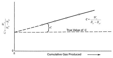
Figure 13-7. Effect of water influx on calculating the gas initially in place.
