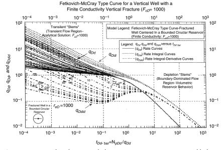
**Figure 16-32.** Fetkovich-McCray decline type curve—rate versus material balance time format for a well with a finite conductivity vertical fracture ( $F_{cD}$ =1000) (*Permission to copy by the SPE, 2003*).
