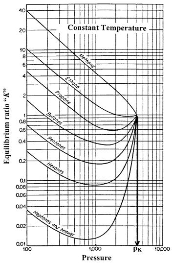
Figure 15-2. Equilibrium ratios for a hydrocarbon system.
