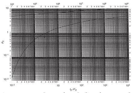
**Figure 16-12.** Dimensionless pressure for a single well in an infinite system, no well-bore storage, no skin. Exponential-integral solution (After Earlougher, R. Advances in Well Test Analysis) (*Permission to publish by the SPE, coyright SPE, 1977*).
