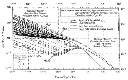
**Figure 16-31.** Fetkovich-McCray decline type curve—rate versus material balance time format for a well with a finite conductivity vertical fracture ( $F_{cD}$ =100) (*Permission to copy by the SPE, 2003*).
