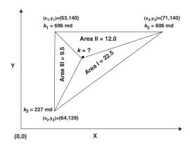
Figure 4-38. Delaunay Triangulation Method.
