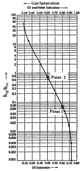
**Figure 5-6.**  $k_{\rm rg}/k_{\rm ro}$  as a function of saturation.
