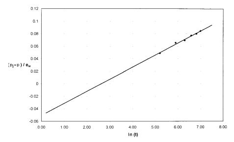
Figure 10-5. Determination of C and n for Example 10-5.
