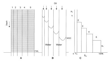
Figure 4-10. Relationship between saturation profile and pore-size distribution.
