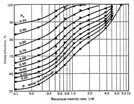
**Figure 14-36.** Areal sweep efficiency as a function of 1/M and f<sub>w</sub>. (Permission to publish by the Society of Petroleum Engineers.)
