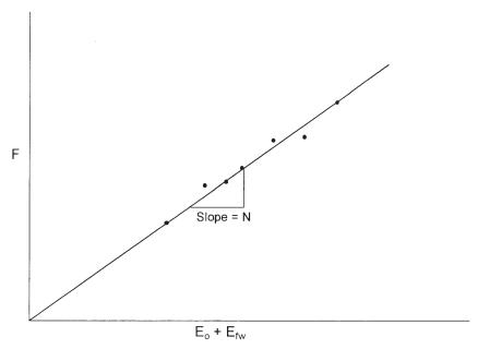
**Figure 11-17.** Underground withdrawal vs.  $E_o + E_{fw}$ .
