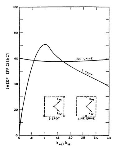
**Figure 14-41.** Effect of directional permeability on E<sub>A</sub>. (*Permission to publish by the Society of Petroleum Engineers.*)
