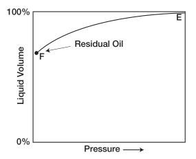
Figure 1-5. Oil-shrinkage curve for low-shrinkage oil.
