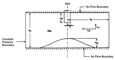
**Figure 9-16.** Illustration of the boundary condition for analytical solution. (After Hoyland, A. et al., courtesy SPE Reservoir Engineering, November 1989.)
