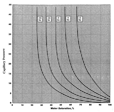
Figure 4-6. Variation of capillary pressure with permeability.
