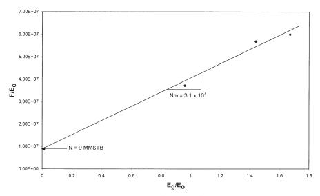
Figure 11-22. Calculation of m and N for Example 11-4.
