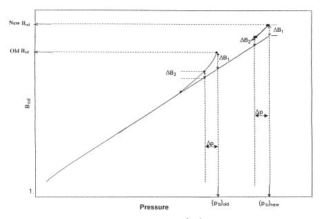
Figure 3-9. Correcting Bod for the new pb.
