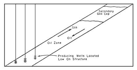
**Figure 11-12.** Gravity-drainage reservoir. (After Cole, F., Reservoir Engineering Manual, Gulf Publishing Company, 1969.)
