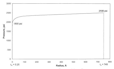
Figure 6-14. Pressure profile around the wellbore.
