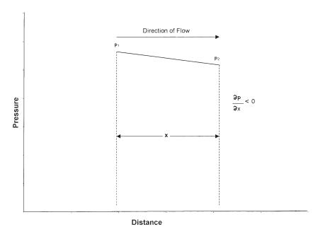
**Figure 6-9.** Pressure vs. distance in a linear flow.
