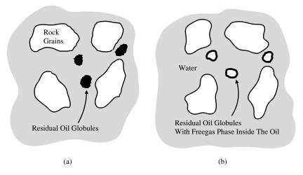
Figure 14-3. Effect of free gas saturation on S<sub>or</sub> (first theory). (After Cole, F., 1969.)
