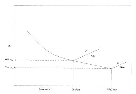
Figure 3-11. Extrapolating oil viscosity above new pb.
