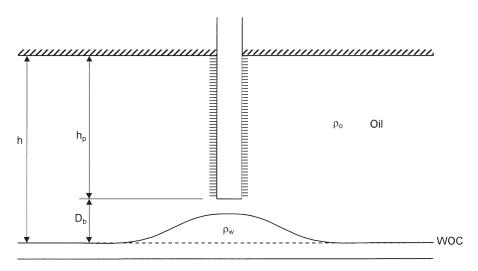
Figure 9-4. Water coning.
