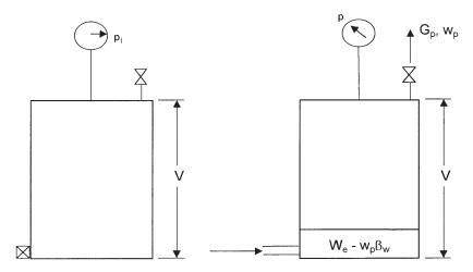
Figure 13-1. Idealized water-drive gas reservoir.
