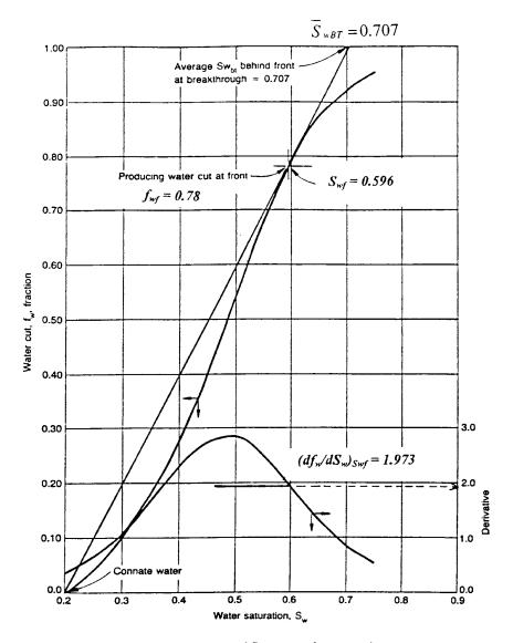
Figure 14-30. Fractional flow curve for Example 14-10.
