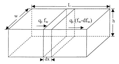
Figure 14-17. Water flow through a linear differential element.
