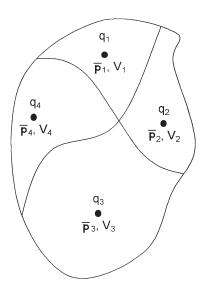
Figure 6-24. Volumetric average reservoir pressure.
