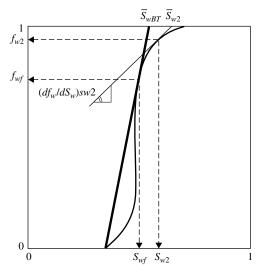
Figure 14-29. Determination of average water saturation after breakthrough.
