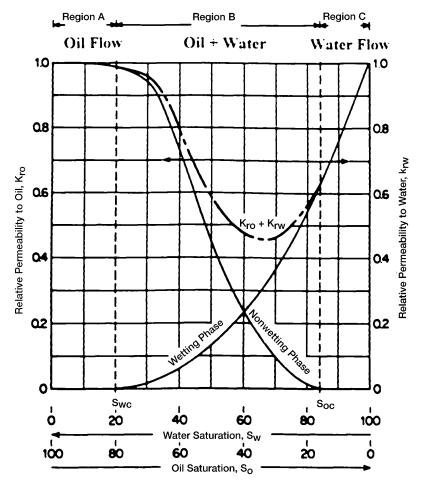
Figure 5-1. Typical two-phase flow behavior.
