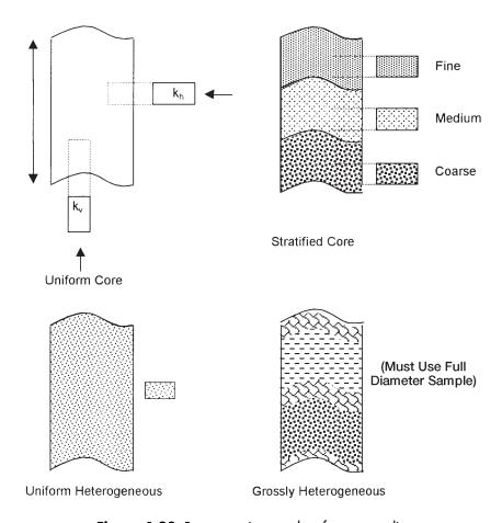
Figure 4-20. Representative samples of porous media.
