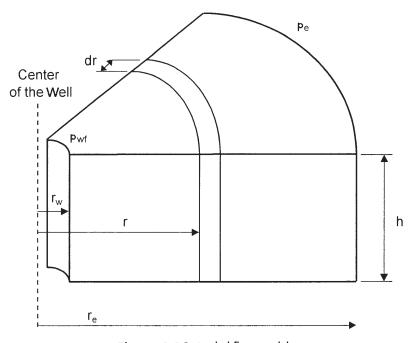
Figure 6-13. Radial flow model.
