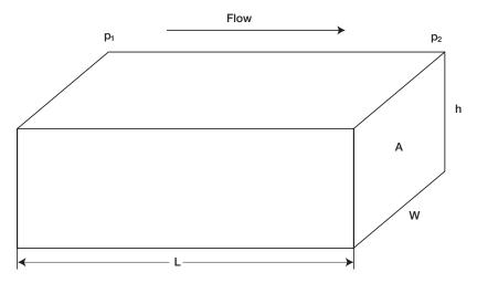
Figure 4-19. Linear flow model.
