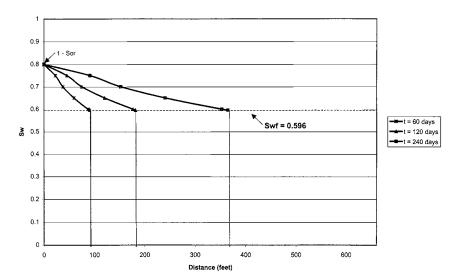
Figure 14-24. Water saturation profile for Example 14-7.
