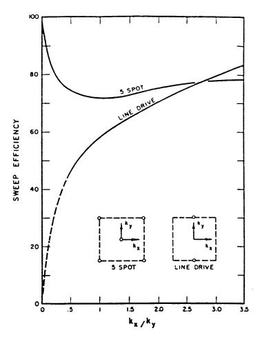
**Figure 14-40.** Effect of directional permeability on  $E_A$ . (*Permission to publish by the Society of Petroleum Engineers.*)
