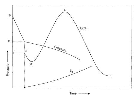
Figure 12-1. Characteristics of solution-gas-drive reservoirs.
