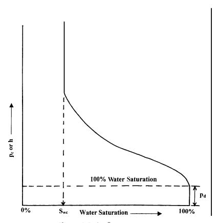
Figure 4-5. Capillary pressure curve.
