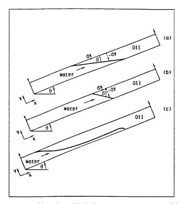
**Figure 14-48.** Stable and unstable displacement in gravity segregated displacement: (a) stable: G > m-1, M > 1, and  $\beta < \theta$ ; (b) stable: G > M-1, M < 1,  $\beta > \theta$ ; and (c) unstable: G < M-1. (Courtesy of Elsevier.)
