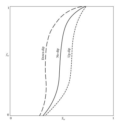
Figure 14-14. Effect of dip angle on fw.
