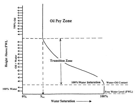
Figure 4-8. Water saturation profile.
