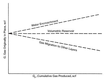
Figure 13-6. Graphical determination of the gas initially in place G.
