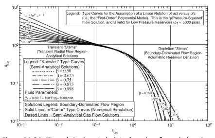
**Figure 16-24.** "First-order" polynominal solution for real-gas flow under boundary-dominated flow conditions. Solution assumes a  $\mu$  c<sub>t</sub> profile that is linear with P<sub>D</sub> (Permission to copy by the SPE, 2000).
