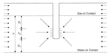
Figure 9-1. Original reservoir static condition.
