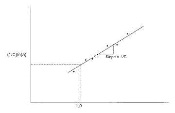
Figure 10-4. Graphical determination of C and a.
