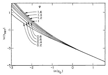
**Figure 9-25.** Dimensionless time for two-cone case. (After Paptzacos, P. et. al., courtesy SPE, 1989.)
