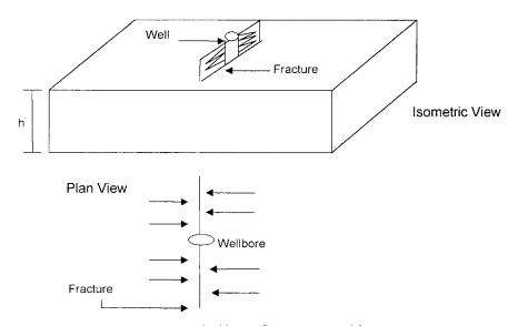
Figure 6-6. Ideal linear flow into vertical fracture.
