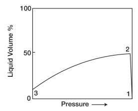
Figure 1-14. Liquid-shrinkage curve for a near-critical gas-condensate system.
