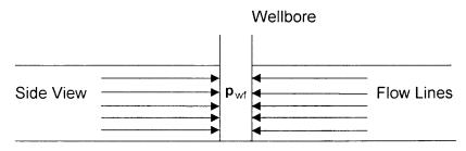
Figure 6-4. Ideal radial flow into a wellbore.
