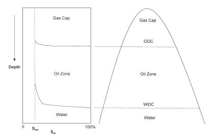
Figure 4-9. Initial saturation profile in a combination-drive reservoir.
