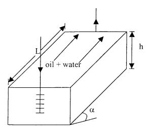
Figure 14-11. Linear displacement in a tilted system.
