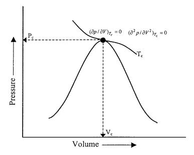
Figure 15-12. An idealized pressure-volume relationship for a pure compound.
