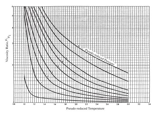
**Figure 2-6.** Carr's viscosity ratio correlation. (Permission to publish by the Society of Petroleum Engineers of AIME. Copyright SPE-AIME.)
