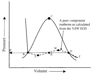
**Figure 15-13.** Pressure-volume diagram for a pure component.
