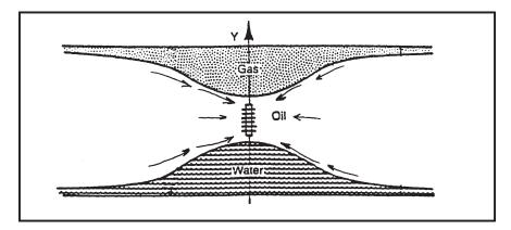
**Figure 9-2.** Gas and water coning.
