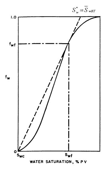
Figure 14-25. Average water saturation at breakthrough.
