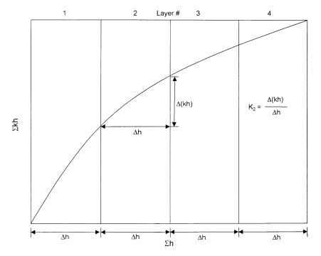
Figure 4-34. Cumulative permeability capacity vs. cumulative thickness.
