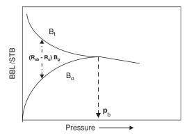
Figure 2-10. B<sub>t</sub> and B<sub>o</sub> vs. Pressure
