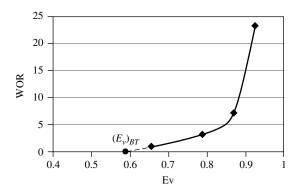
**Figure 14-55.** WOR versus E<sub>V</sub> relationship.
