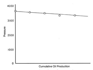
Figure 11-9. Pressure-production history for a water-drive reservoir.
