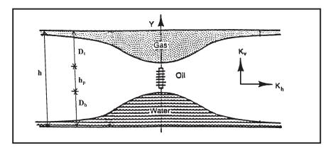
Figure 9-5. The development of gas and water coning.
