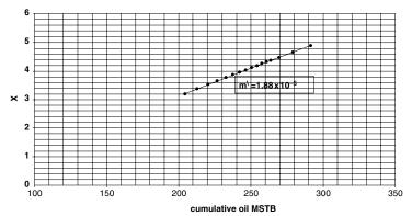
Figure 14-59. X-plot of a simulated waterflood.
