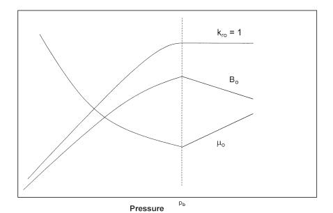
**Figure 7-5.** Effect of pressure on  $B_o$ ,  $\mu_o$ , and  $k_{ro}$ .
