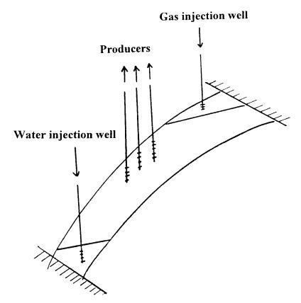
Figure 14-10. Well arrangements for dipping reservoirs.
