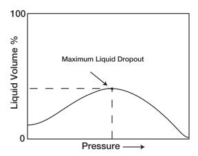
Figure 1-12. A typical liquid dropout curve.
