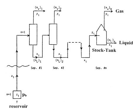
Figure 15-8. Schematic illustration of n separation stages.
