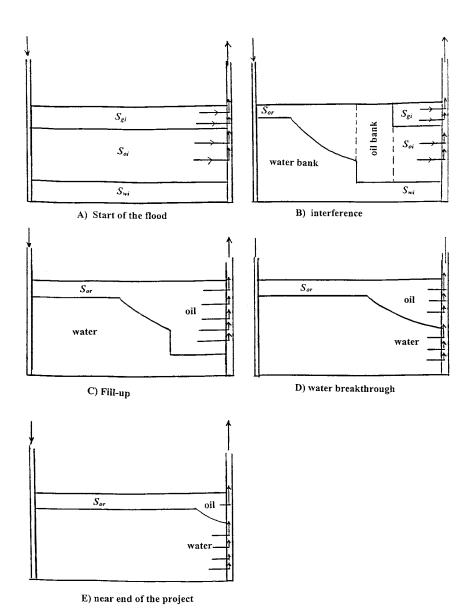
Figure 14-44. Stages of waterflooding.
