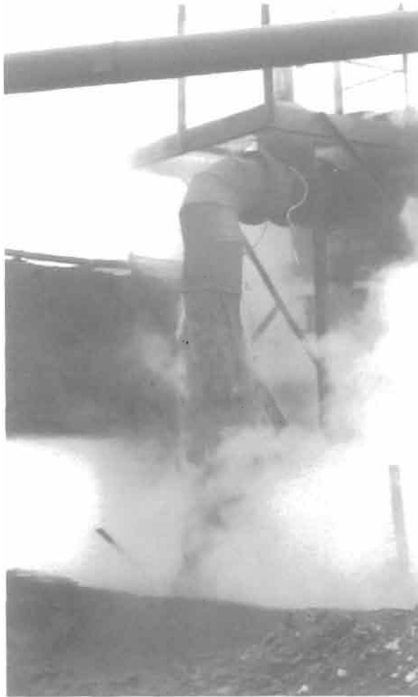
Figure 12. Air emissions from sludge water generated from scrubbing blast furnace off-gases.
