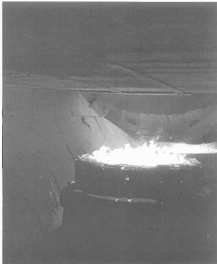
Figure 9. Shows BOF pouring molten steel into ladles.
