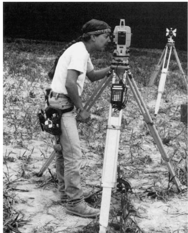
FIGURE 15.5 Total station (on foreground tripod), data collector (attached to leg of tripod), and prism (on background tripod). (Courtesy of Ray Root)
