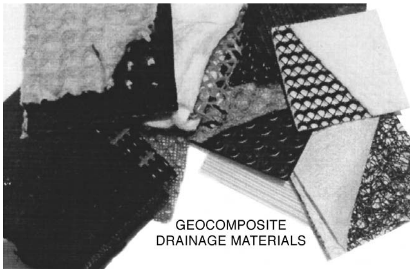
FIGURE 27.14 Typical geocomposite sheet drains.
