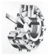
Fig. 6.5 Orifice flowmeter.
