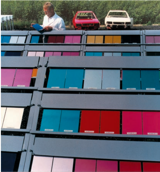
Fig. 3.3.31 Weathering station in Münster, D
