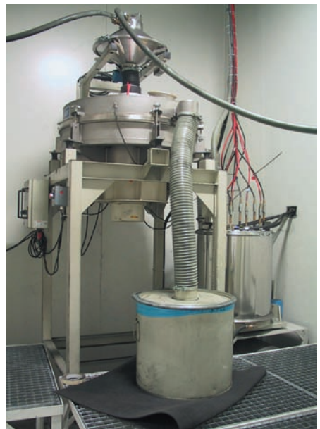
Fig. 4.2.129 Ultrasonic screen for powder regeneration
