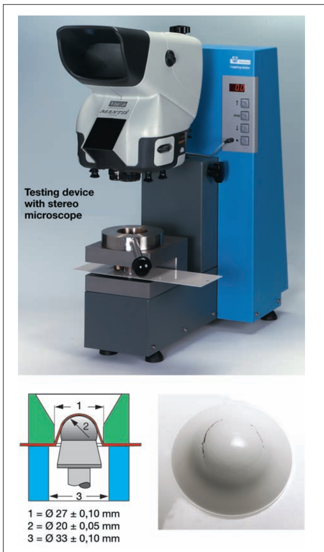
Fig. 3.2.71 Erichsen cupping test device according to DIN EN ISO 1250
