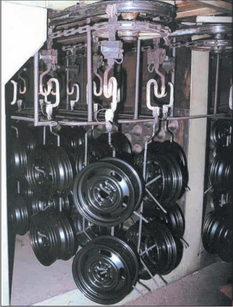
Fig. 7.3.3 Steel wheels primed by cathodic electro-deposition process
