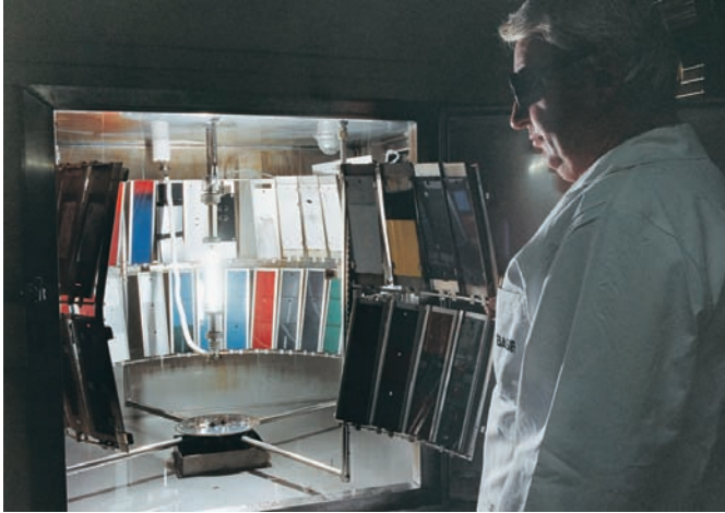
Fig. 3.3.22 Test cycles and test chamber of weather-o-meter equipment
