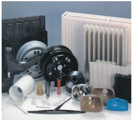
Fig. 4.2.15 Examples of industrially by electrodeposition process coated products
