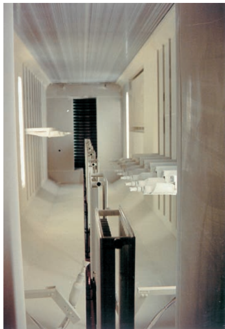
Fig. 4.2.130 Picture of a powder application unit for industrial coating
