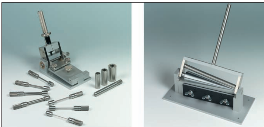
Fig. 3.2.70 Cylindrical mandrel test according to DIN EN ISO 1519 and conical mandrel test according to DIN EN ISO 6860
