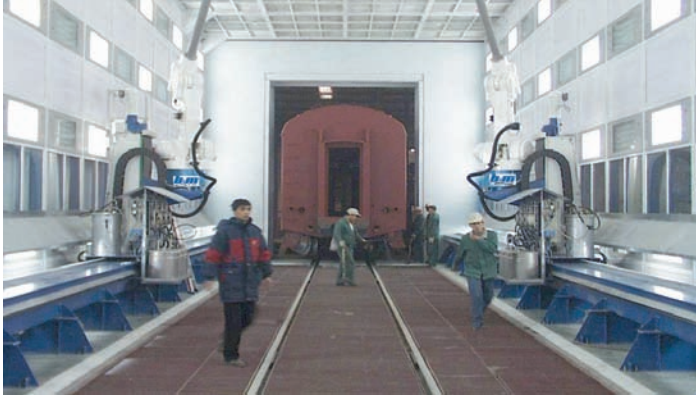
Fig. 7.9.1 Coating of rail vehicles in huge automated cabins
