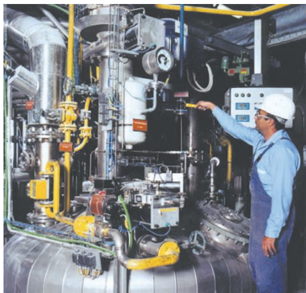
Fig. 2.1.47 Vessel for manufacturing alkyd resins
