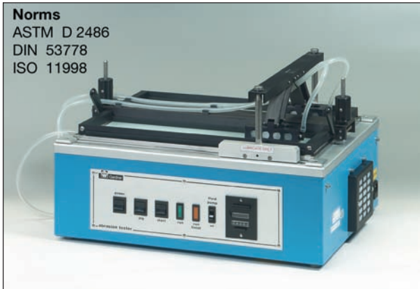
Fig. 3.2.87 Equipment for determination of abrasive resistance according to DIN EN ISO 11998
