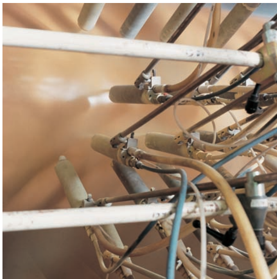
Fig. 7.11.1 Powder coating of pipe lines
