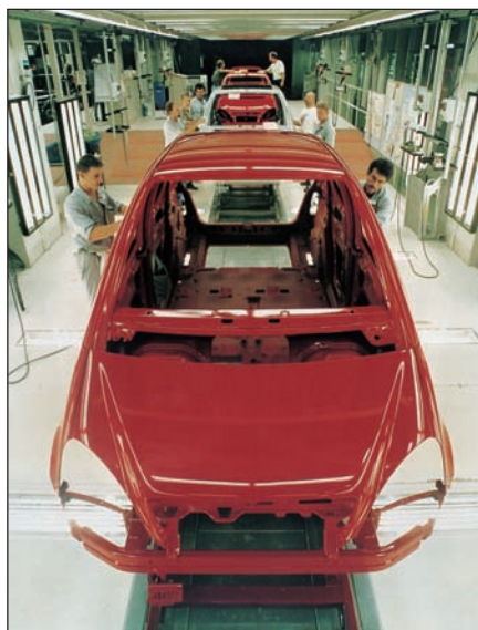
Fig. 7.1.17 Inspection line of coated automotive bodies
