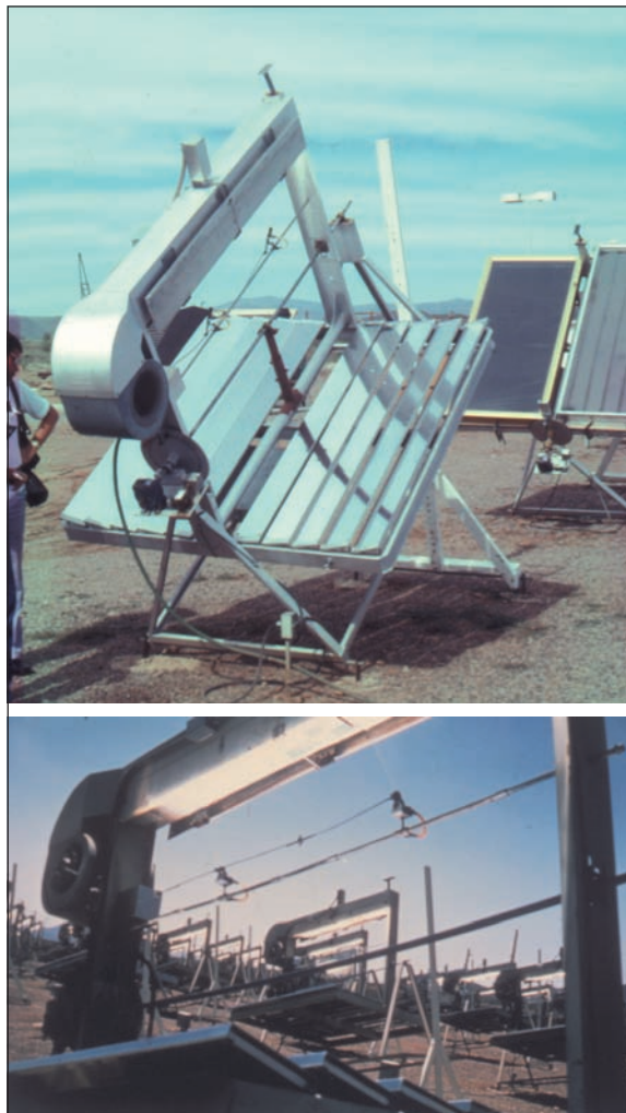
Fig. 3.3.20 EMMAQUA equipment for accelerated weather tests in Arizona
