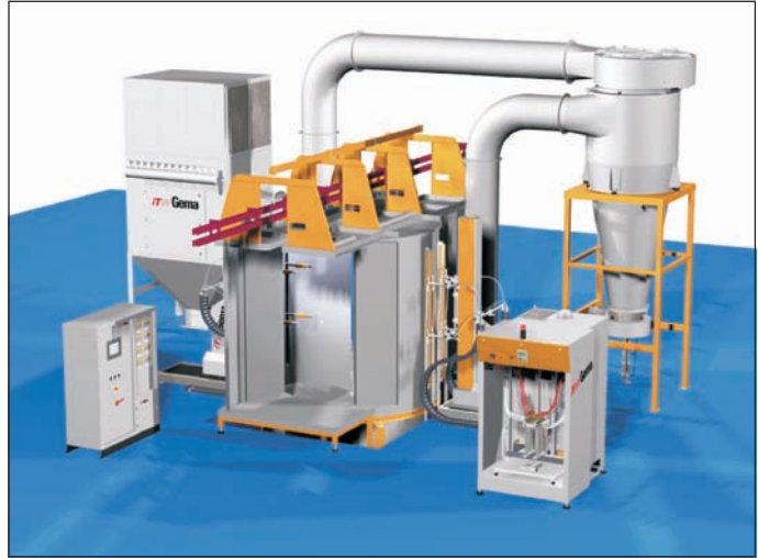
Fig. 4.2.128 Multicyclone for powder recovery
