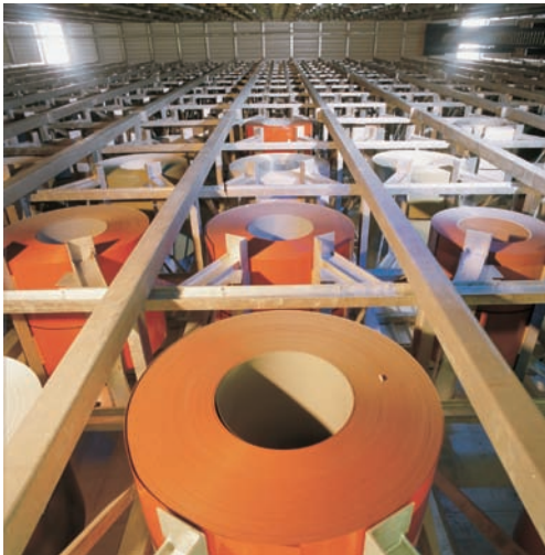
Fig. 7.4.3 Storage of coated coils
