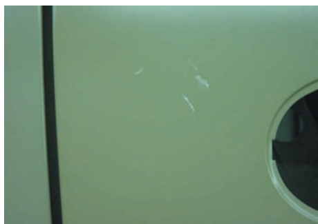
Fig. 6.2.5 Overlooked rests of a PVC sealer on a body surface
