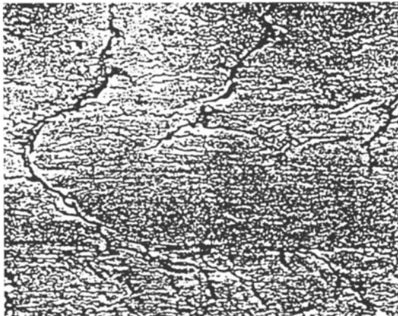
Figure 2.32 Microcracks in the initial failure phase (electron micrograph, two-stage surface replica, magnification 17,500 \times ).
