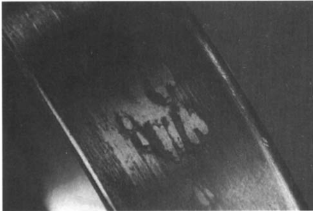
Figure 12.79 Fretting corrosion on the outer surface of a rolling element bearing. (Courtesy of Caterpillar, Inc., Peoria, IL.)
