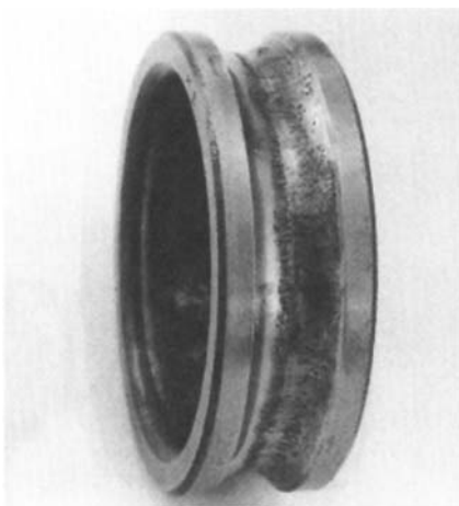
Figure 2.81 The appearance of the working surface in the final phase of fatigue wear.
