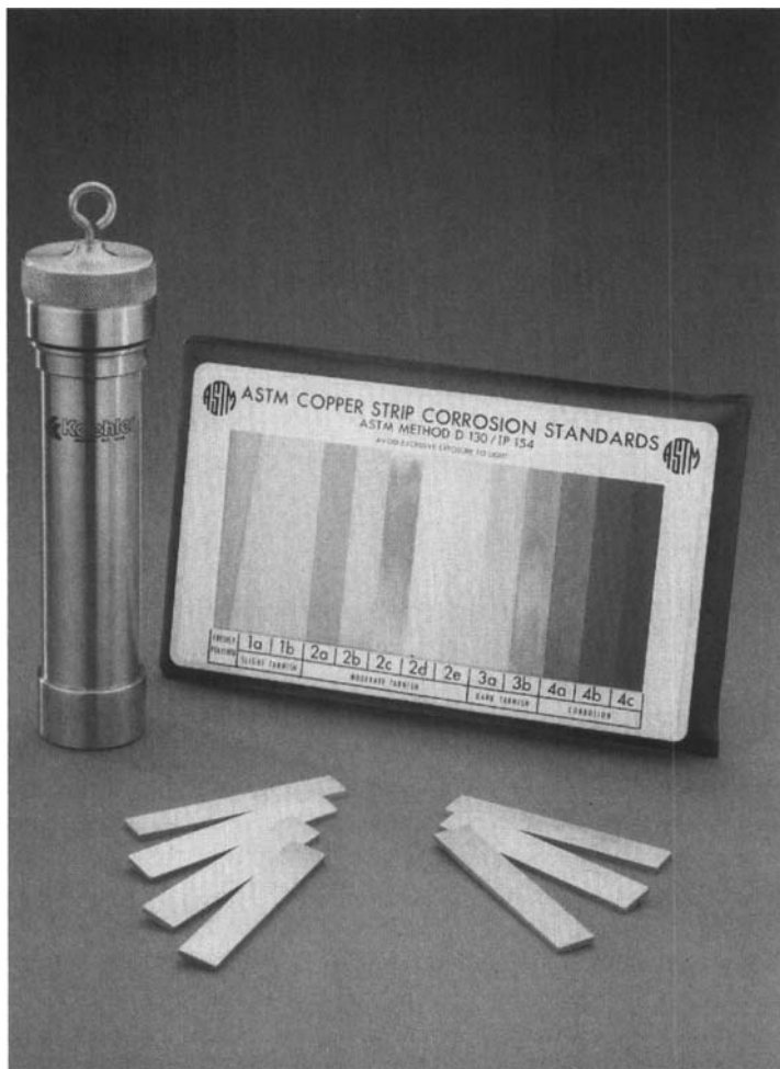
Figure 14.20 Illustration of the ASTM Copper Strip corrosion Standards. (Courtesy of Koehler Instruments Inc.)
