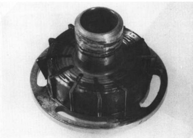
Figure 12.14 Rotor, vanes, and bushing covered with fluid oxidation deposits. (Courtesy of DMT-Gesellschaft für Forschung and Prüfung mbH, Essen, Germany.)
