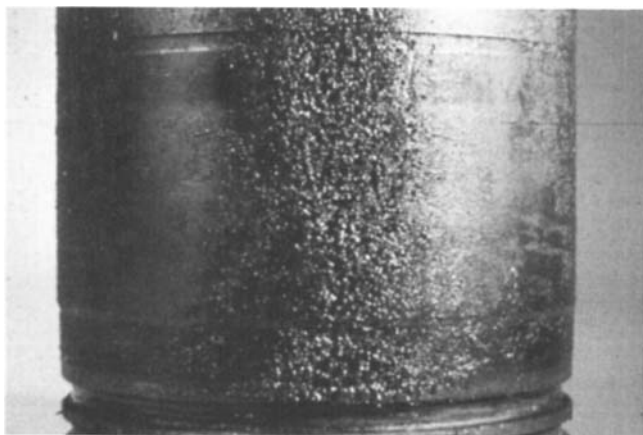
Figure 12.41 Illustration of cavitation surface damage. (Courtesy of IFAS, Aachen, Germany.)
