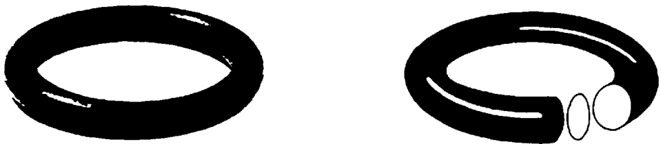
Figure 9.8 An O-ring profile.
