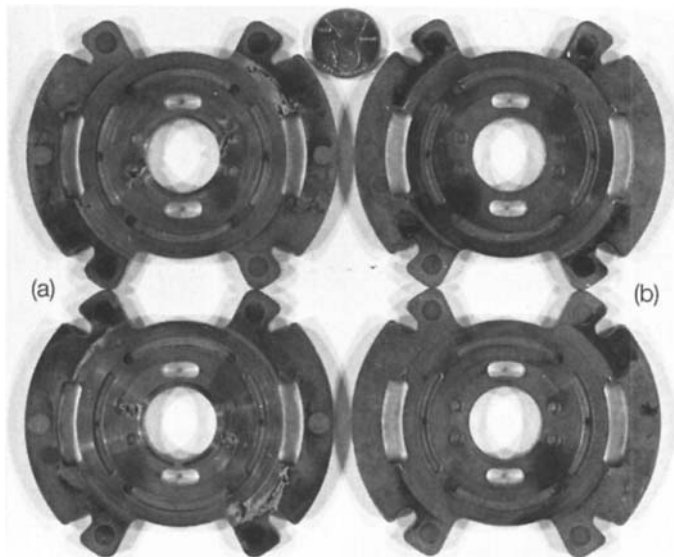
Figure 10.37 Comparison of 20VQ5 bushing wear (by cavitation) obtained at two speeds (A) 1200 rev/min and (B) 2400 rev/min at 3000 psi using a fluid that exhibited very low wear on the ring and vanes (12 and 10 mg total wear, respectively after 100 h).
