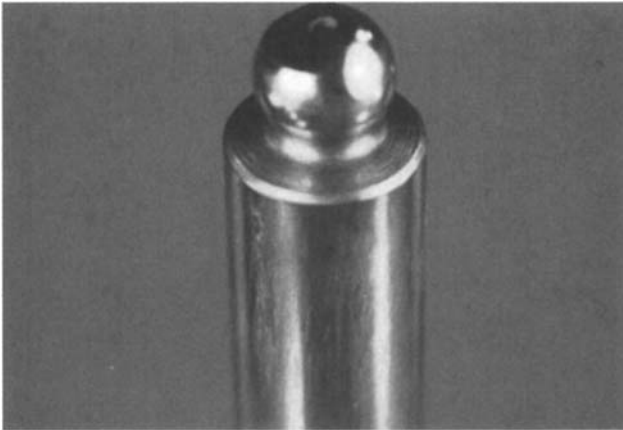
Figure 12.32 This hydraulic pump piston has undergone polishing due to smearing. (Courtesy of Caterpillar Inc., Peoria, IL.)
