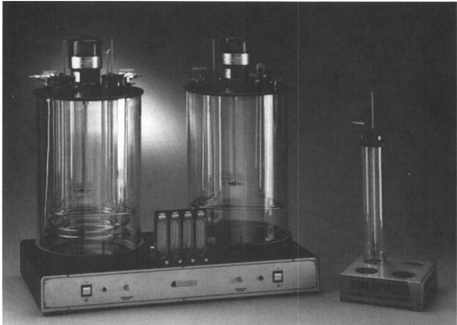
Figure 23.14 ASTM D-892 apparatus. (Courtesy of Koehler Instrument Co.)
