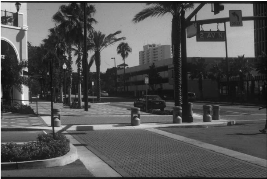
FIGURE 21.4 Corner bulb-out on arterial street.
