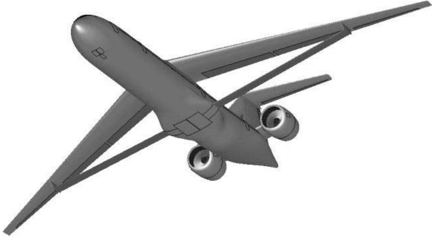
FIGURE 26.3 The strut-braced wing concept.
