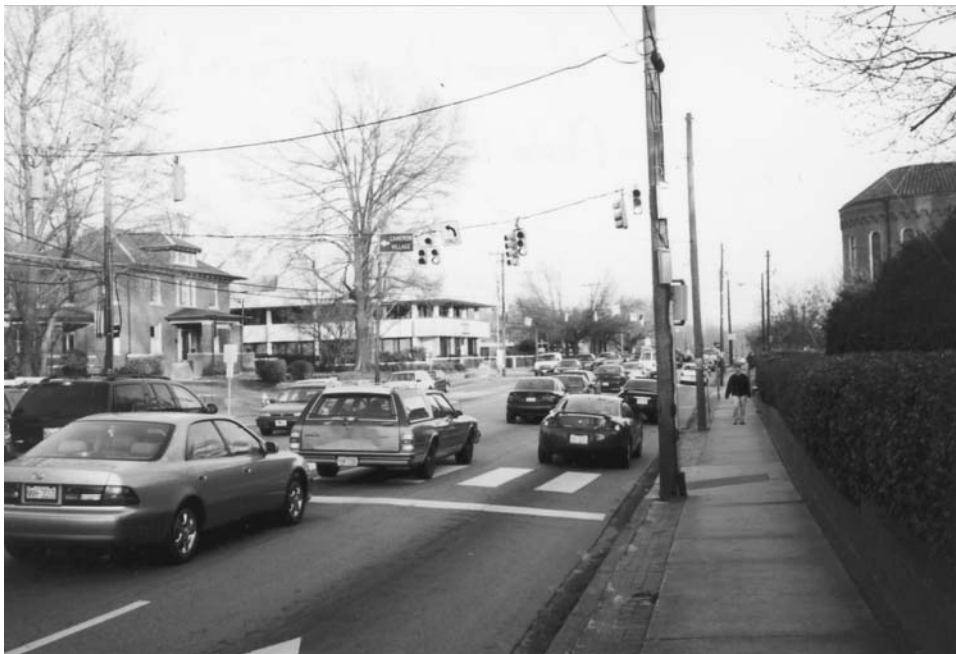
FIGURE 14.1 Traffic queuing at one intersection spills back to block another intersection, adding to delay and causing potential safety problems. (Source: Daniel L. Carter.)
