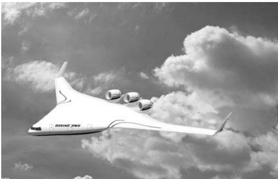
FIGURE 26.2 The blended wing body concept (courtesy Boeing).
