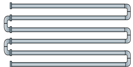
Fig. 6.1.12 Zig-zag holding tube.
