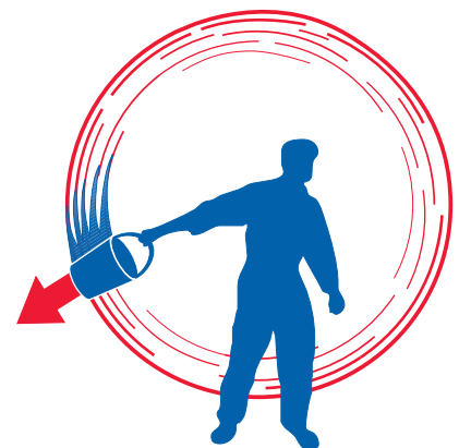
Fig. 6.2.13 Centrifugal force is generated in a rotating vessel.
