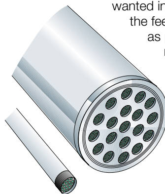
Fig 6.4.7 The filter elements, 1, 7 or 19 (shown) in parallel, are installed in a stainless steel module.
