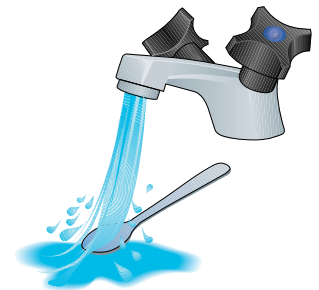
Fig. 6.1.4 Heat transfer by convection. Example: The spoon is rinsed in running cold water. Heat is absorbed by the water and the spoon gets cooler, until the spoon and the water are at the same temperature.
