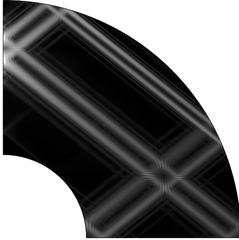
Fig. 7.3. The kinetic energy of an axisymmetric inertial mode at frequency \omega = 0.7822 associated with an attractor where the shear layers are clearly visible. The fluid is viscous and incompressible. In this numerical solution, \eta = 0.35 is the ratio of the shell radii, L = 1000 is the number of spherical harmonics used, N_r = 400 is the number of radial grid points, and the Ekman number measuring viscosity is E = 1.0 \times 10^{-9} . Stress-free boundary conditions have been used.
