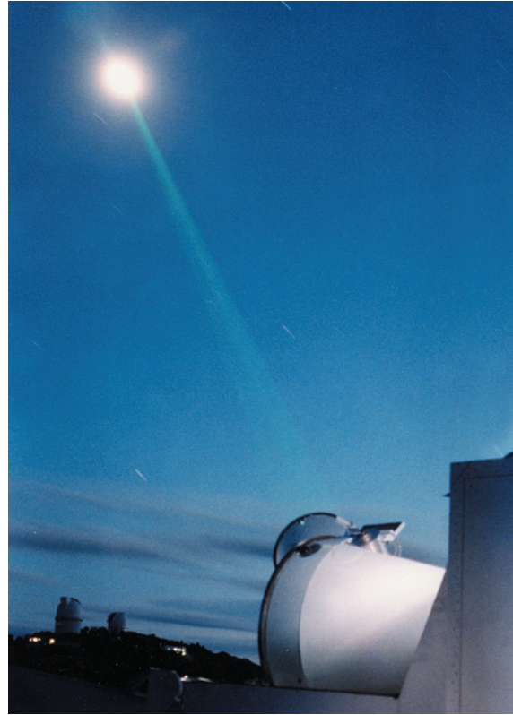
Fig 8.6. The 2.7 m telescope of the McDonald Observatory, Texas, has been used to fire a laser beam at a reflector on the Moon, then they detect the weak return. By timing the round trip, the distance to the Moon is very accurately determined. [McDonald Observatory]
