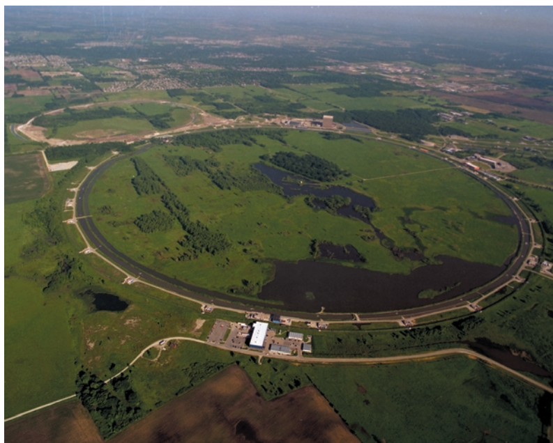
Fig 21.18. Aerial view of Fermilab, the large particle accelerator outside Chicago. The ring has a diameter of over 6 km. [Fermilab photo]
