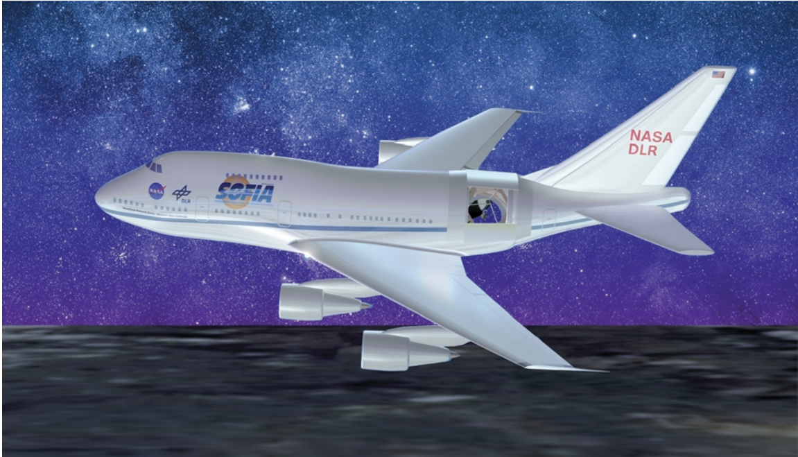
Fig 4.23. Artist's impression of the Stratospheric Observatory for Infrared Astronomy (SOFIA), which will be made from a converted 747 SP. [NASA]
