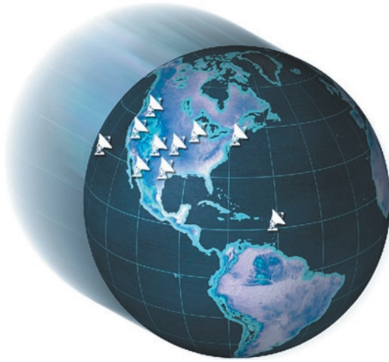
Fig 4.31. Arrangement of telescopes for the Very Long Baseline Array (VLBA), operated by the NRAO. There are ten telescopes, each 25 m in diameter. It operates down to a wavelength of 1 cm. [NRAO/AUI/NSF]
