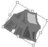
Figure 10-2: The bounding box shows the original placement angle and can reset to that angle.
