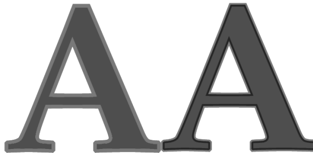
Figure 7-2: Text as it appears in InDesign (left). Text (right) as it appears when printed with trapping applied.
