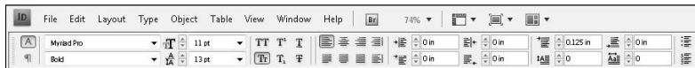
Figure 2-5: The Control panel as it appears when the Type tool is active.
