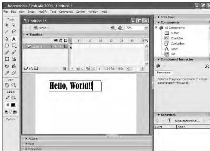
Figure 2-4: With the Text tool, you can easily write text onto the Stage.
