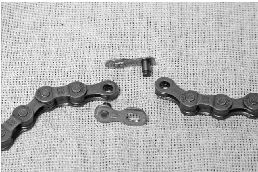
Figure 10-1: An SRAM PowerLink chain.
