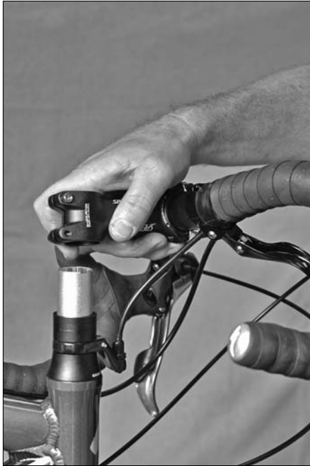
Figure 15-13: Removing the stem.
