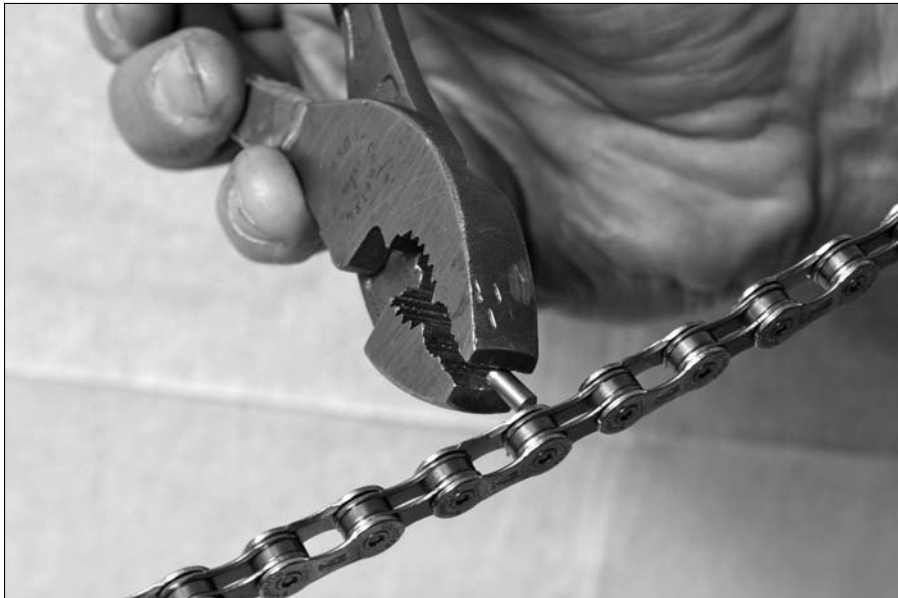
Figure 10-15: Snapping off the replacement pin's head.
