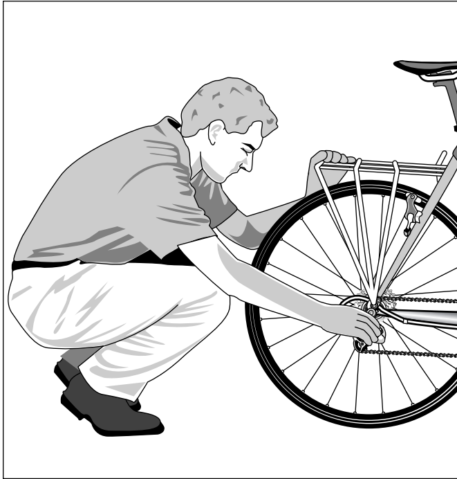
Figure 12-5: Checking the frame from the back.
