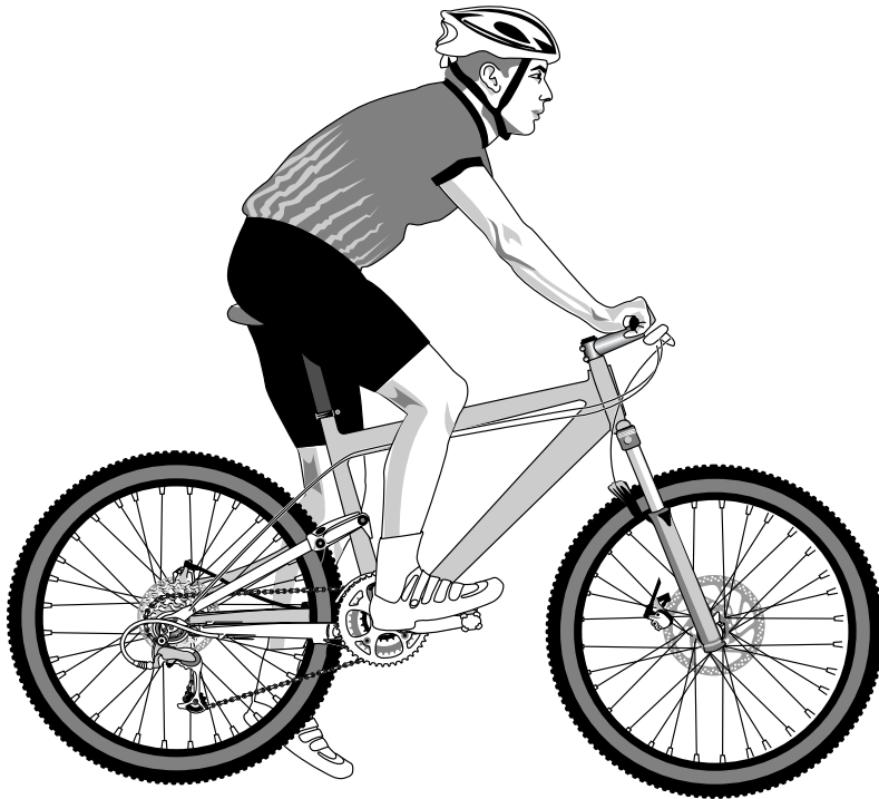
Figure 18-2: The proper saddle height.
