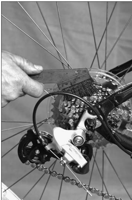
Figure 16-1: Using a brush to clean the sprockets.
