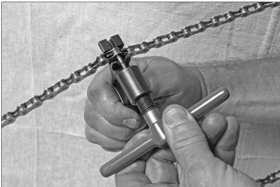
Figure 10-11: Preparing to separate a chain
