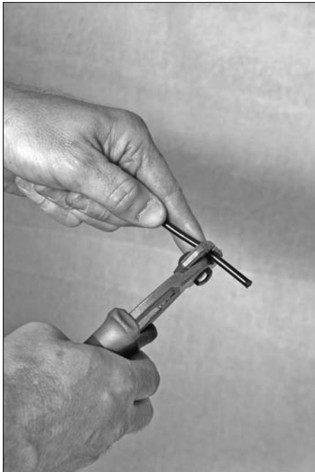
Figure 8-21: Cutting the cable housing.
