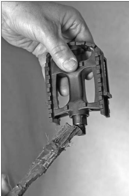
Figure 13-3: Lubricating the pedal.
