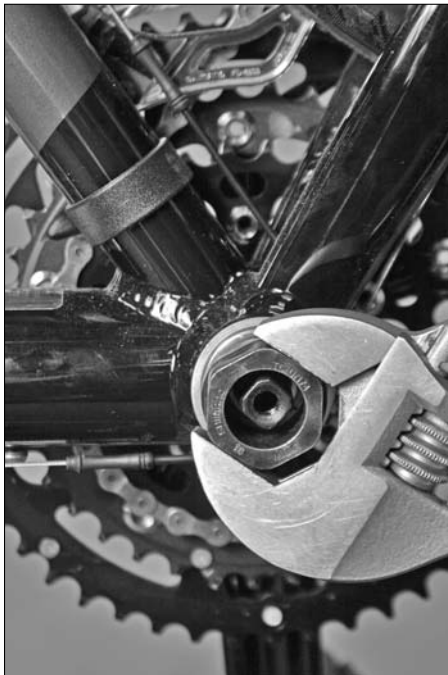
Figure 13-12: Using the bottom bracket tool.
