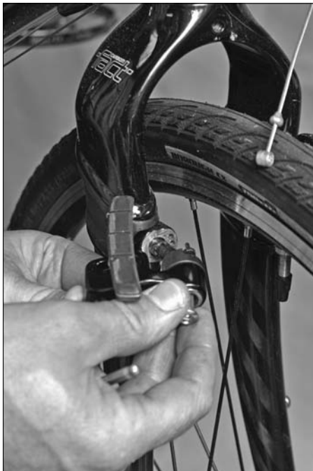
Figure 8-8: Removing the brake.
