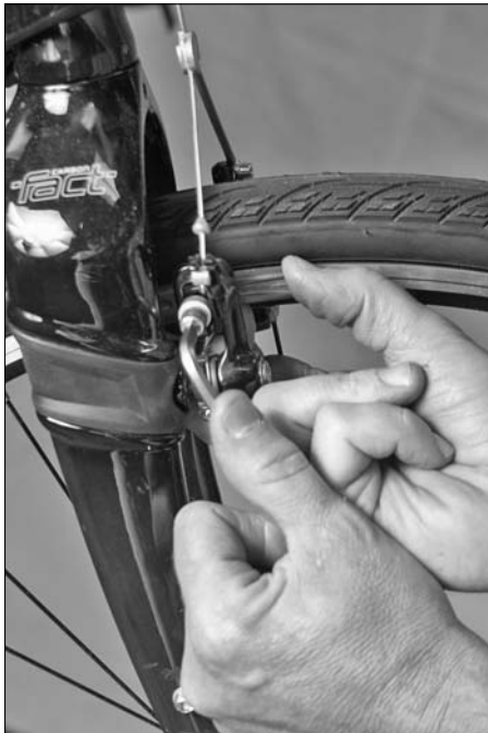
Figure 8-12: Adjusting the brake.
