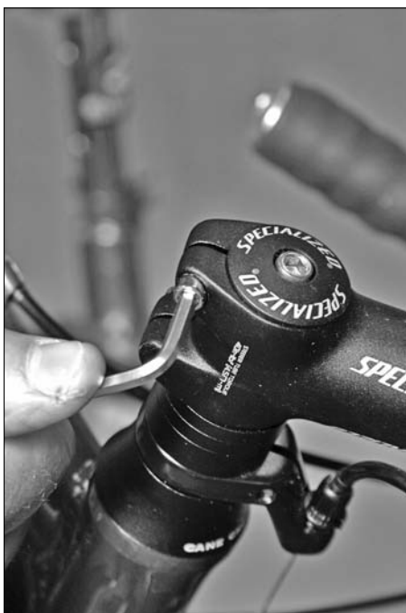
Figure 15-12: Undoing the clamp bolt.
