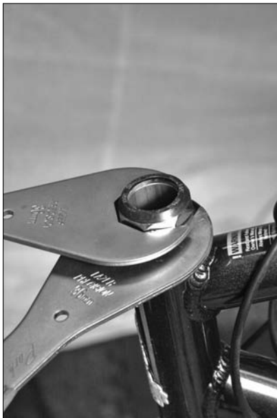
Figure 15-20: Undoing the locknut.
