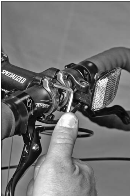
Figure 14-16: Adjusting the position of the gear shifters.
