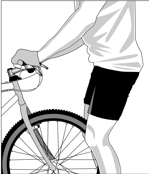
Figure 18-3: Checking for loose- ness in the handlebars and stem.
