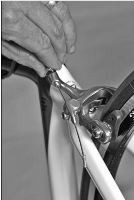
Figure 8-16: Adjusting the cable on center- mount brakes.
