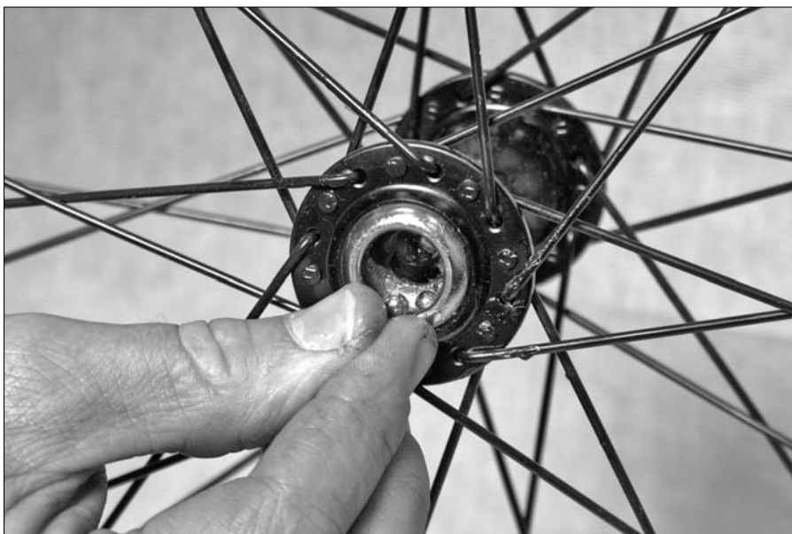
Figure 7-9: Inserting the bearings.
