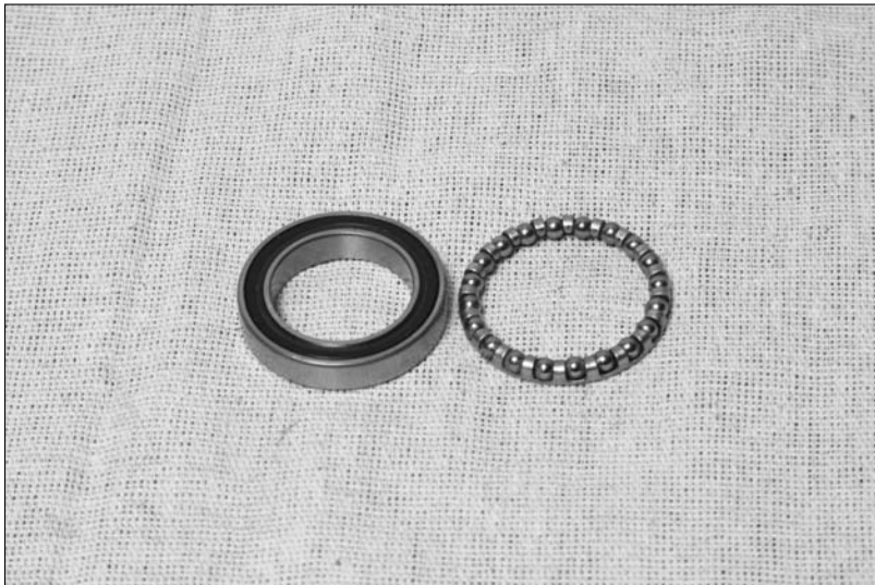
Figure 15-17: Two styles of bearings.
