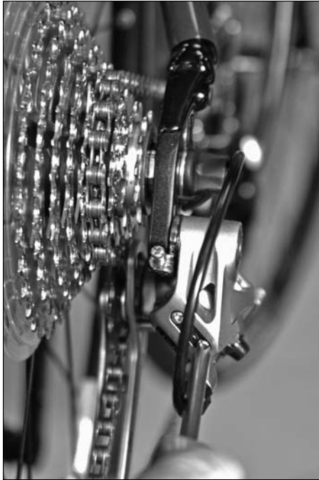
Figure 14-7: Adjusting the L screw.
