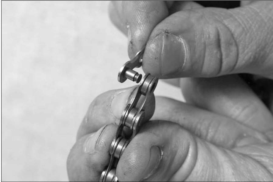
Figure 10-13: Connecting an SRAM PowerLink- type chain.
