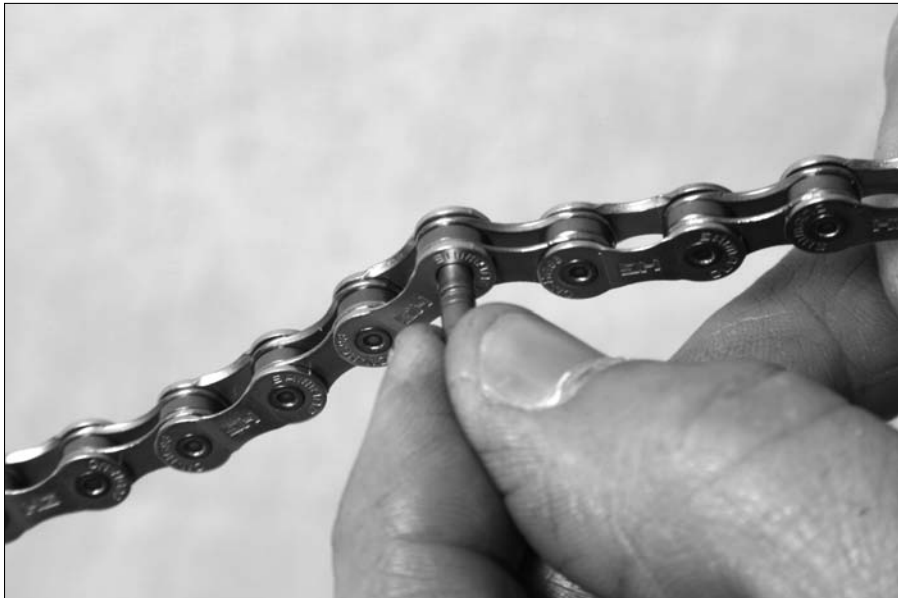
Figure 10-14: Inserting the pin.
