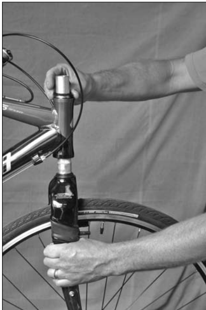
Figure 15-15: Removing the fork.
