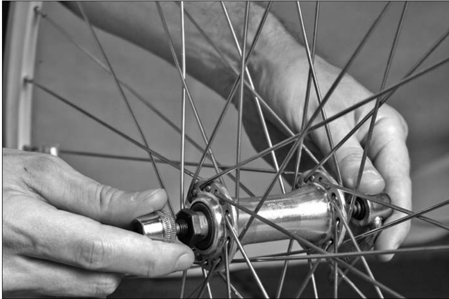
Figure 7-2: Removing a quick- release wheel.
