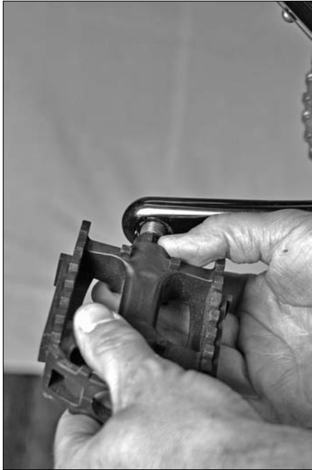
Figure 13-4: Reattaching the pedal.
