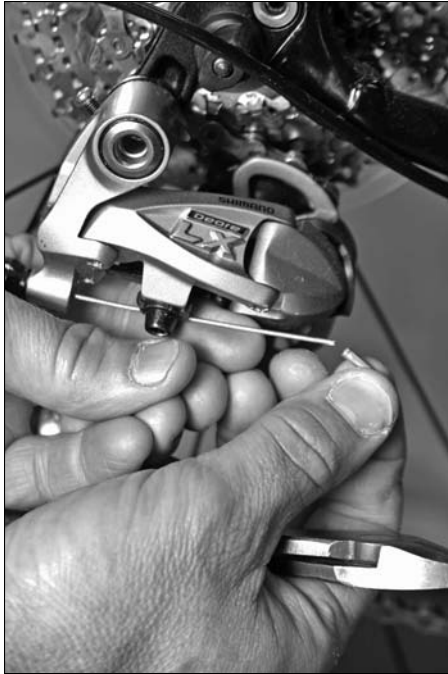
Figure 14-9: The cable cap.
