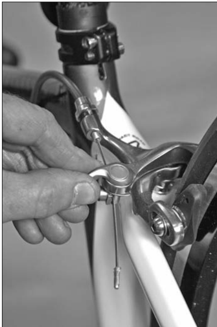
Figure 8-14: Moving the lever on center- mount brakes
