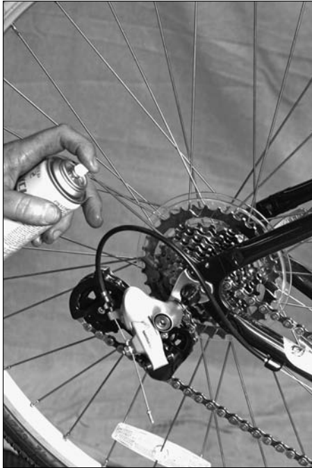
Figure 16-2: Degreasing various parts of a bike.
