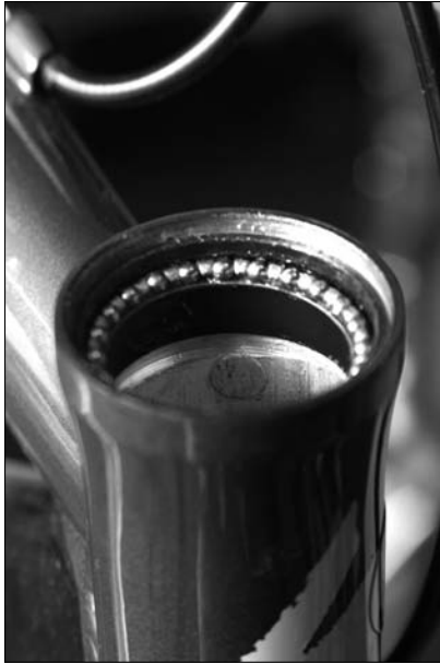
Figure 15-16: Bearings in the headset.
