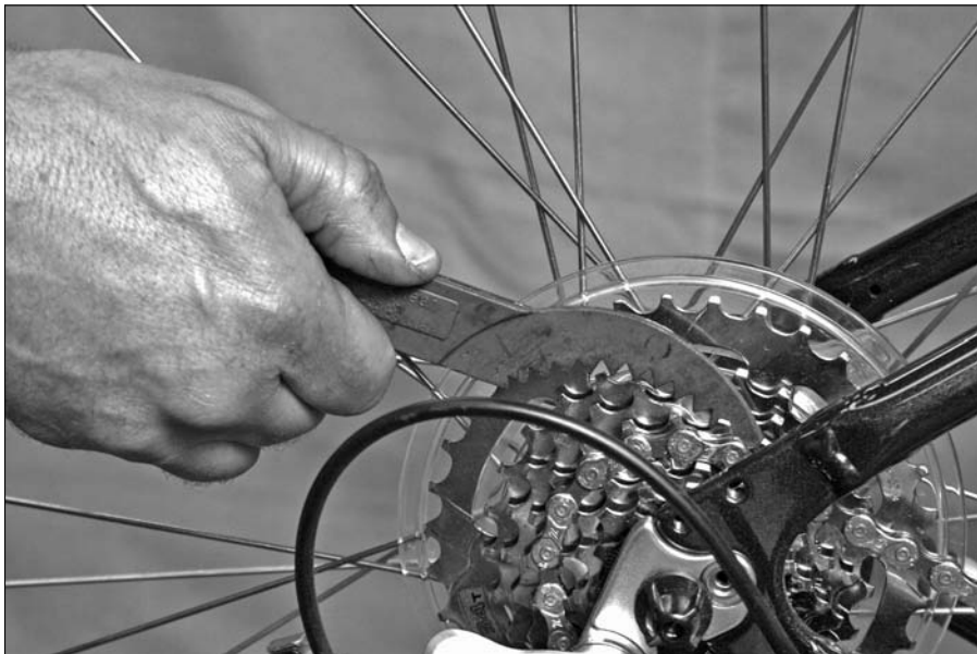
Figure 16-3: Digging out dirt between the cogs.
