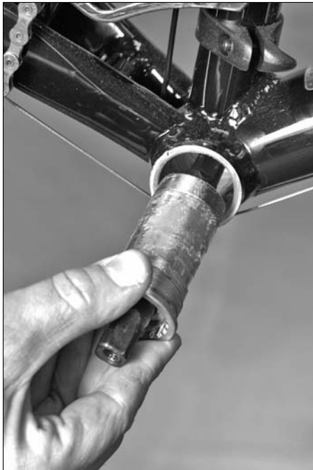
Figure 13-13: Removing the cartridge
