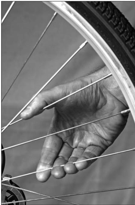
Figure 7-13: Feeling for loose areas.
