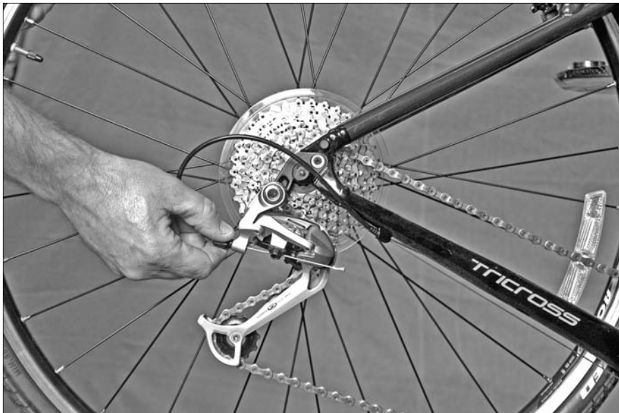
Figure 14-10: The barrel adjuster.
