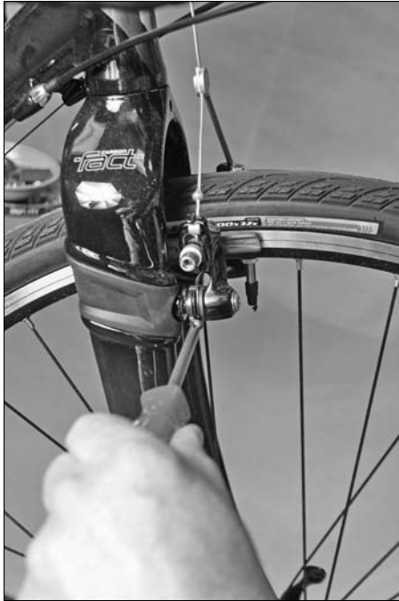
Figure 8-13: Adjusting brake tension.
