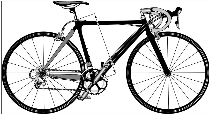
Figure 19-3: How frame size is measured.
