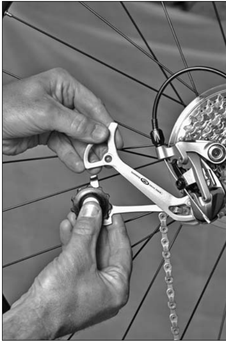
Figure 14-4: Separating the cage.
