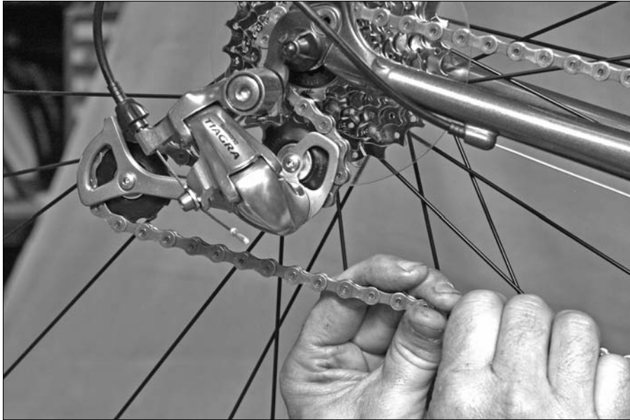
Figure 10-12: Measuring the chain
