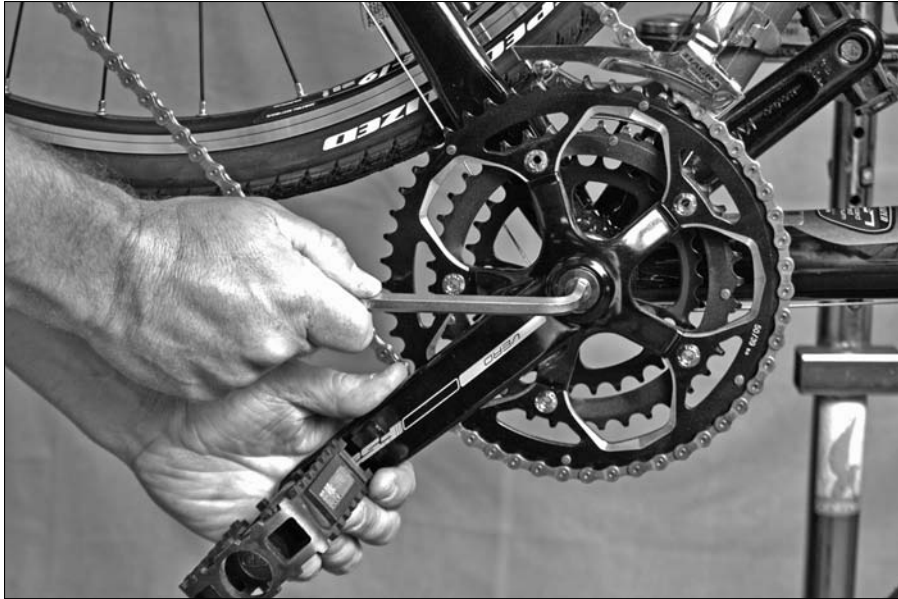
Figure 13-7: Loosening a cotter- less crank with an Allen wrench.
