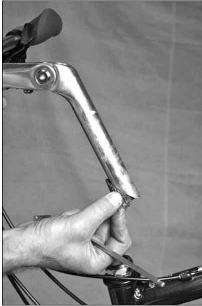
Figure 15-19: Removing the stem.
