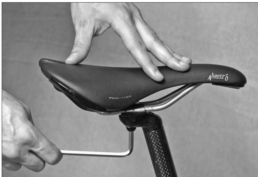
Figure 9-8: Adjusting the saddle
