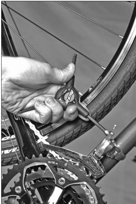
Figure 14-11: Removing the cable.
