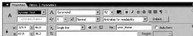
Figure 4-13: To display data in a dynamic text box, you enter the applicable variable name.
