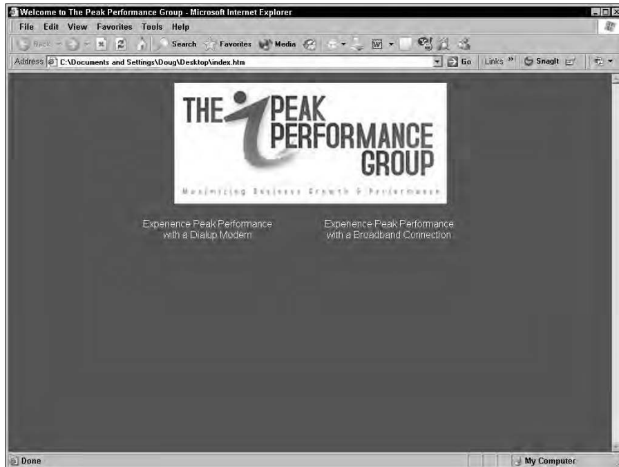
Figure 2-1: You create an HTML portal to direct viewers to the version of your site that suits their connection speed.
