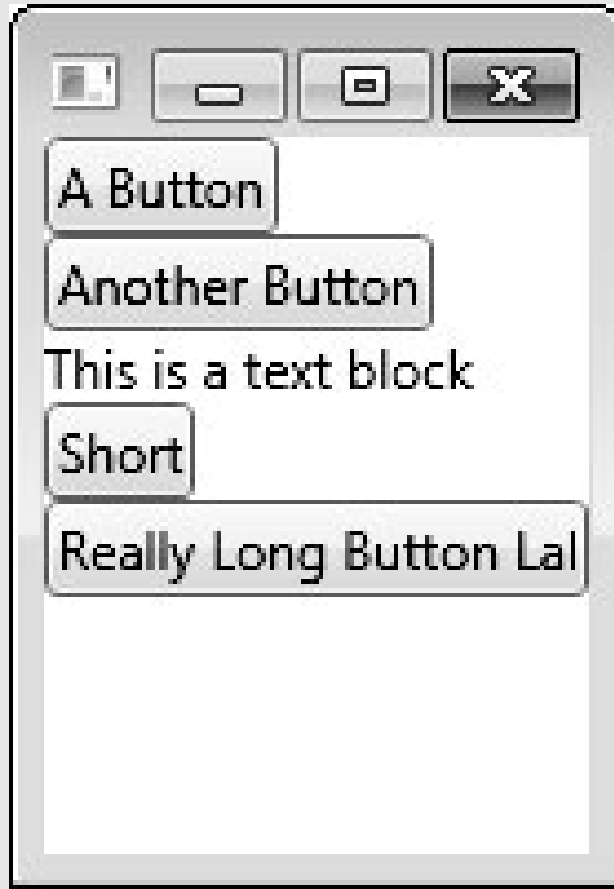
A Stack Panel
