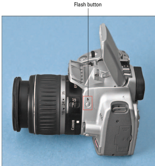
Figure 5-22: Want flash? Just press the Flash button, and you're set to go.
