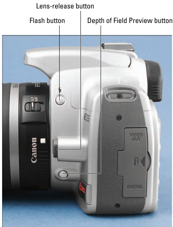
Figure 1-8: Press the Flash button to bring the built-in flash out of hiding.
