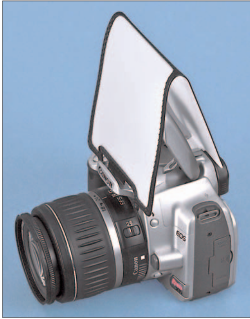
Figure 5-30: If you don't own an external flash head, try using a diffuser to soften the light from your built-in flash.
