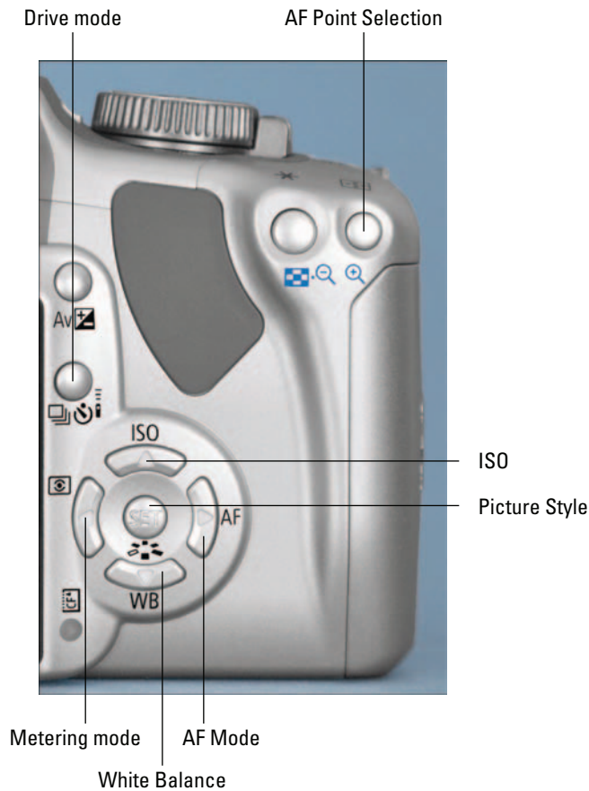
Figure 7-1: You can access several critical settings with a press of a single button.
