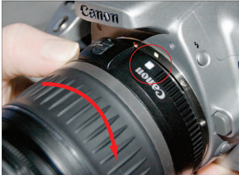
Figure 1-2: Place the lens in the lens mount with the mounting indexes aligned.
