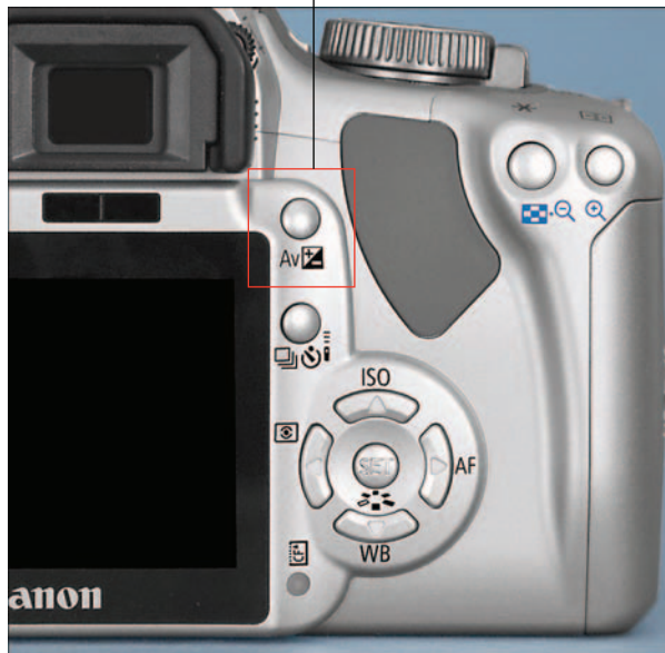
Figure 5-16: To set aperture in M mode, press the Exposure Compensation button as you rotate the Main dial.
