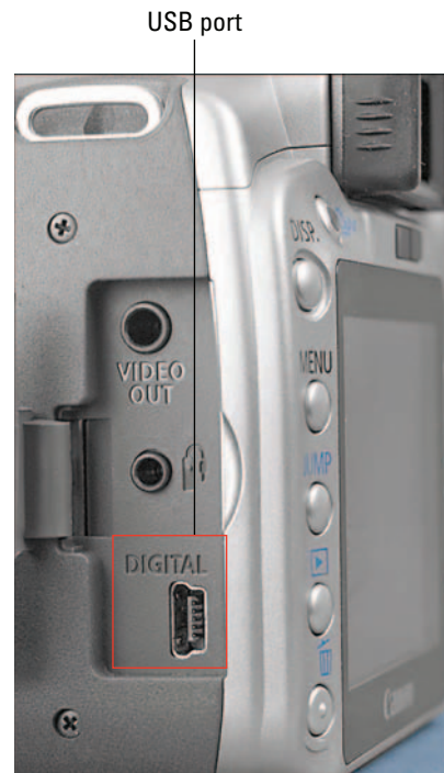
Figure 8-3: The USB port is hidden under the little rubber door on the left rear side of the camera.
