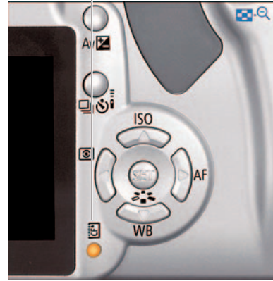
Figure 2-4: The card access lamp lights while the camera sends the picture data to the card.
