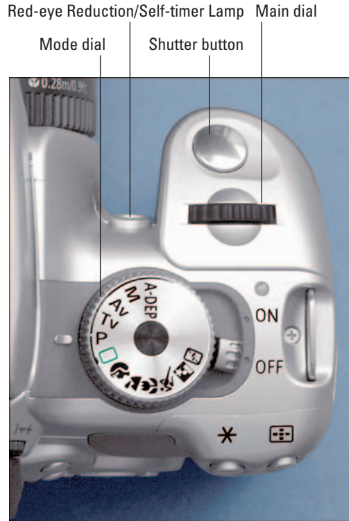
Figure 1-6: The tiny pictures on the Mode dial represent special automatic shooting modes.
