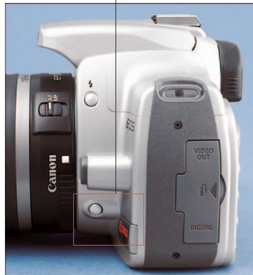
Figure 6-13: Press this button to see how the aperture setting will affect depth of field.
