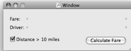
Figure 6-3: Add four Label controls, a push button, and a check box to the interface.
