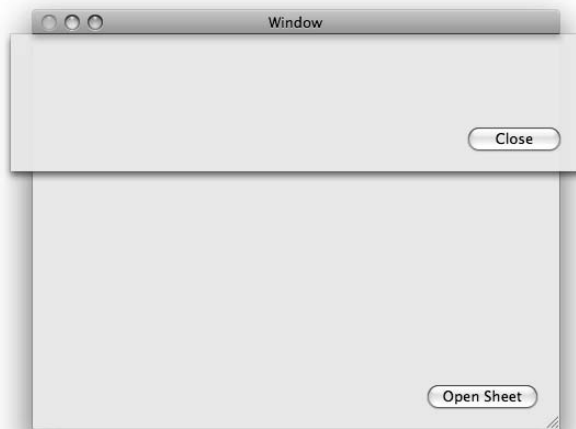
Figure 8-5: When the functionality of your window is directly tied to another window, display it as a sheet.
