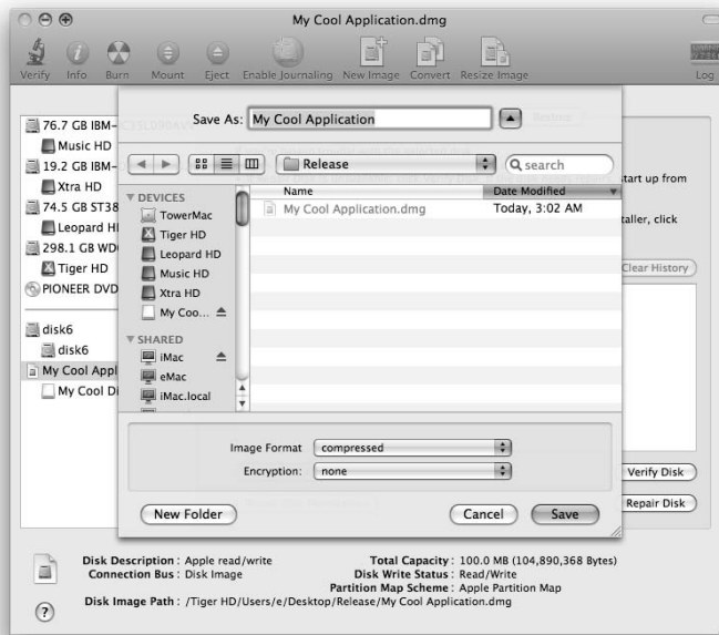
Figure 5-19: Create a new compressed disk image to eliminate the extra space from the original disk image.
