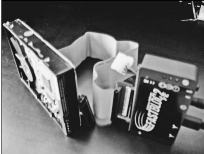
Figure 6-10: Positioning an EIDE write block device and an EIDE hard drive.
