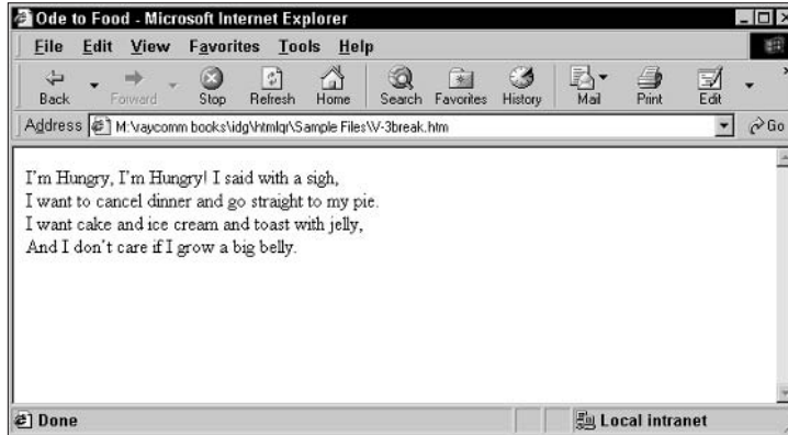
Figure 5-3: Using <BR> to force line breaks helps you control the way your Web page text appears.
