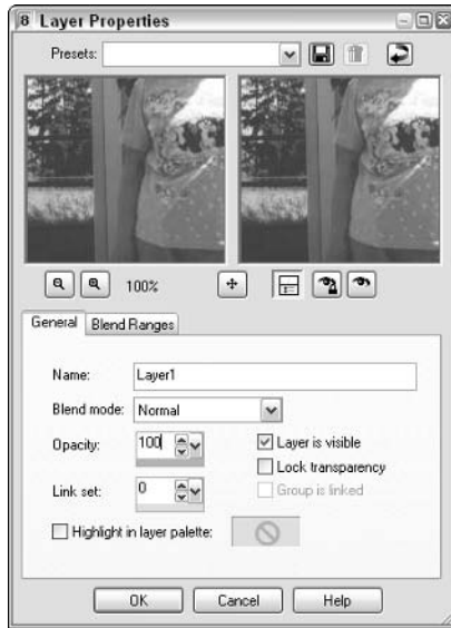
Figure 4-4: In Paint Shop Pro, you use the Layers Properties dialog box to set the transparency attribute for an image.
